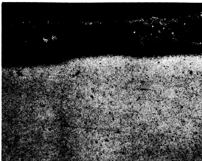
Figure 7. Photomicrograph of Inconel 690 Electrode Exposed to Glass Containing 21 Wt% ZrO_2 Calcine
