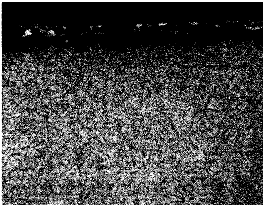
Figure 6. Photomicrograph of Inconel 690 Electrode Exposed to Gas Phase from Glass Containing 21 Wt% ZrO_2 Calcine
