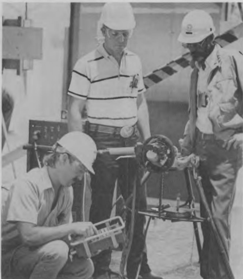
Parameters for the automatic welding head are set using a hand-held keyboard.
