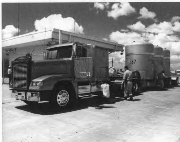
Contact handled transuranic waste shipped to WIPP has specially designed packagings.
