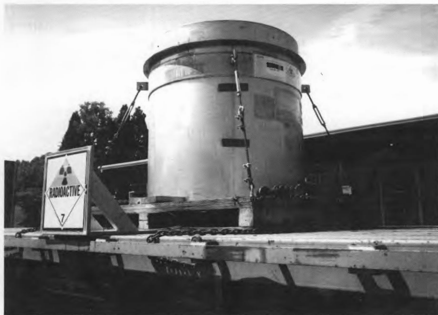
Materials with higher levels of radioactivity are transported in Type B packages.
