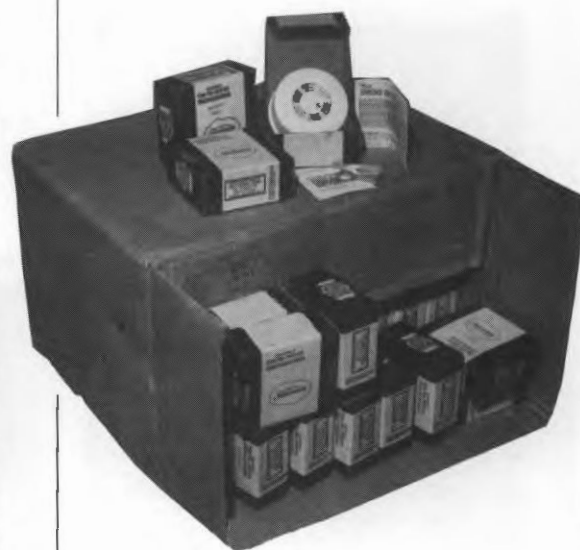
Excepted packages are used to transport materials that present low hazards because of their low concentration of radioactive material. Examples are consumer goods, such as smoke detectors.
