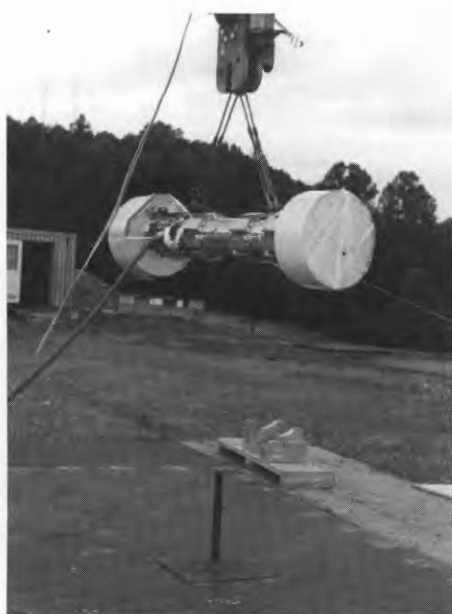
This scale model of a spent fuel cask is ready for the puncture test. Instruments attached to its left side will collect performance data.
