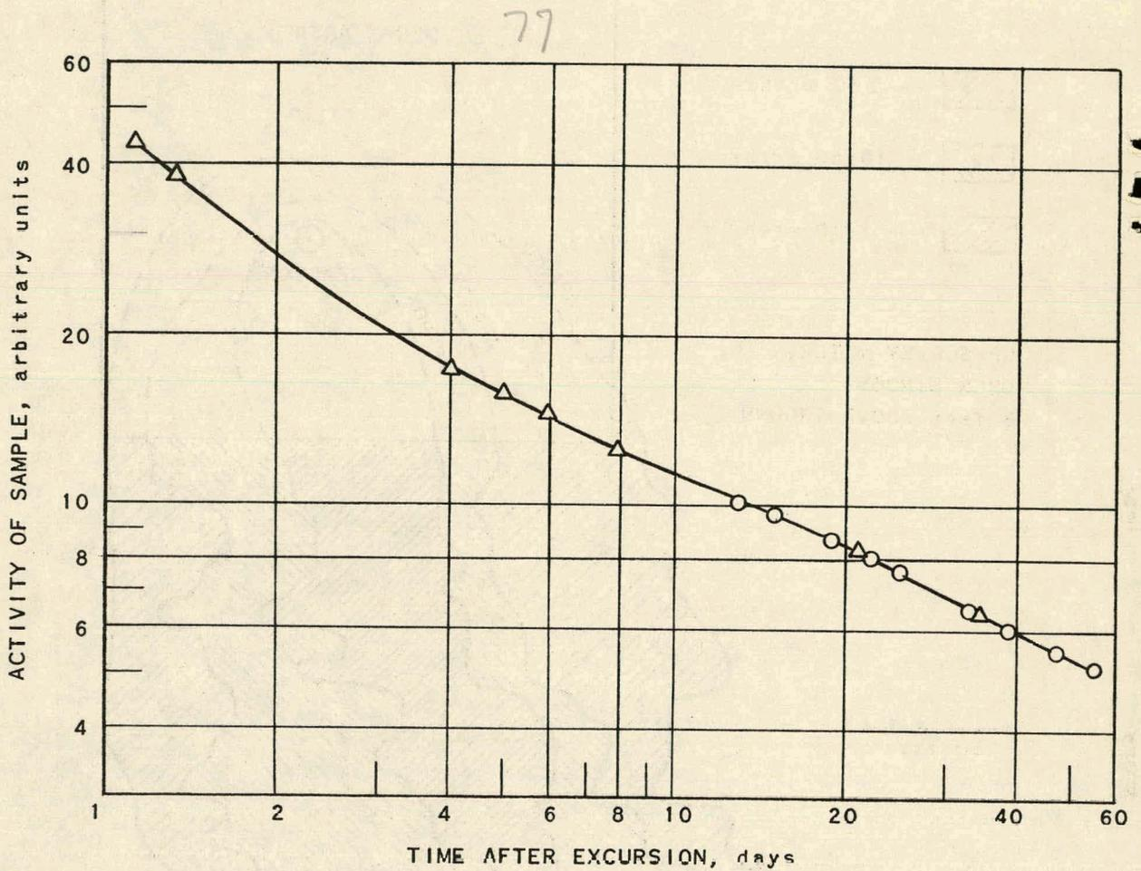
△ MEASUREMENTS BY IDO RADIATION PROTECTION SECTION (CONTAMINATION FROM SHOE COVER)
