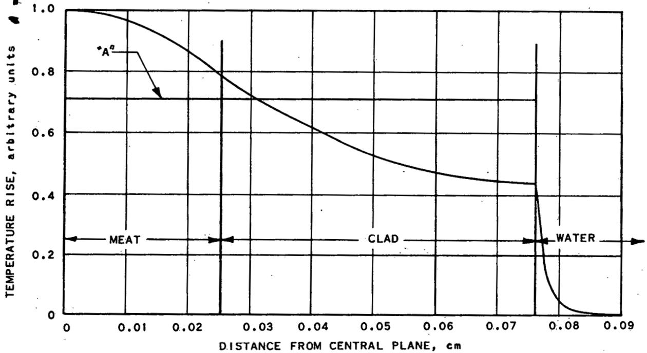
LINE 'A' MARKS UNIFORM TEMPERATURE RISE WHICH WOULD EXIST IF FUEL PLATE CONDUCTIVITY WERE INFINITE AND NO HEAT WERE LOST TO WATER
