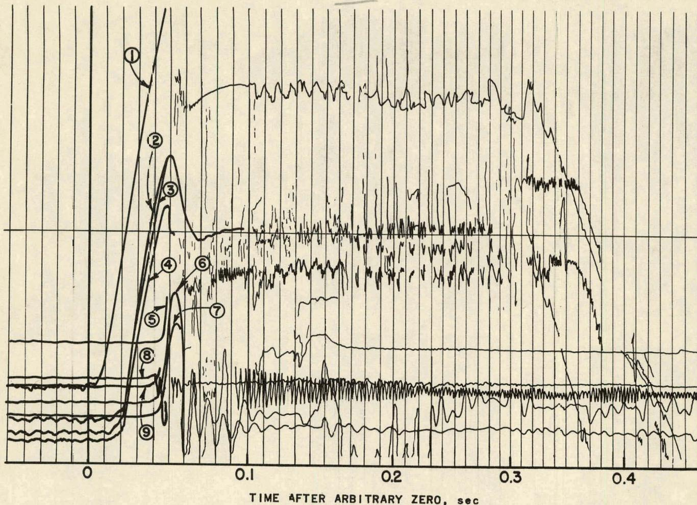
TRACES 1,2,3 & 4 ARE LOGARITHMIC RECORDS OF CURRENTS FROM ION CHAMBERS IN VARIOUS POSITIONS
