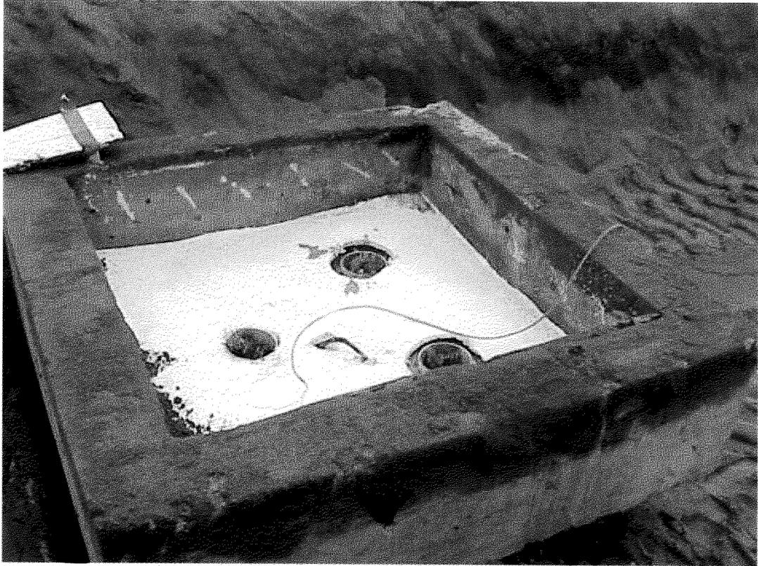
Figure 22. GMENT-12 thrust block (underside showing Styrofoam liner).
