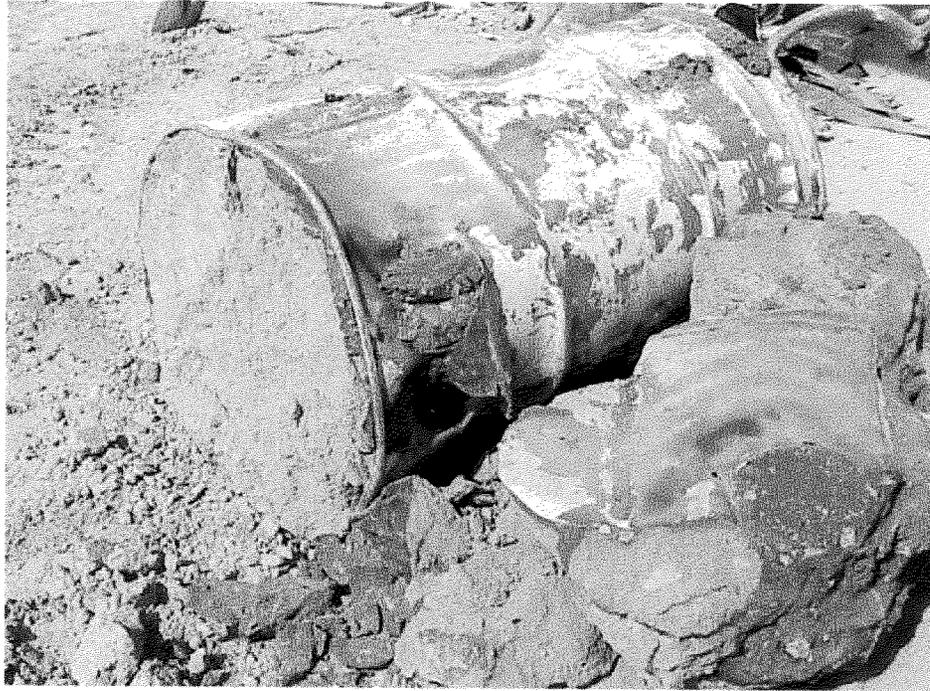
Figure 52. Puncture of drum by the drill steel (left-hand side of drum), showing the cylindrical shape of the drill steel.
