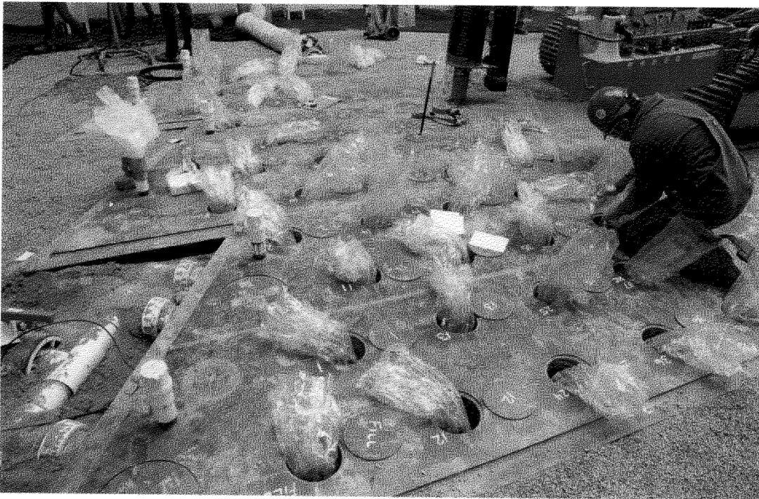
Figure 39. Plastic sleeves extended out of thrust block in preparation for testing (treated with talcum powder) (Photo PN01-520-3-5A).
