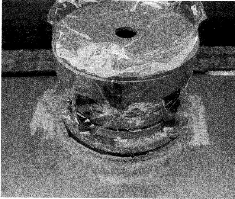
Figure 38. Detail of the underside of the thrust block showing plastic diaphragm and the rigid plastic plate.
