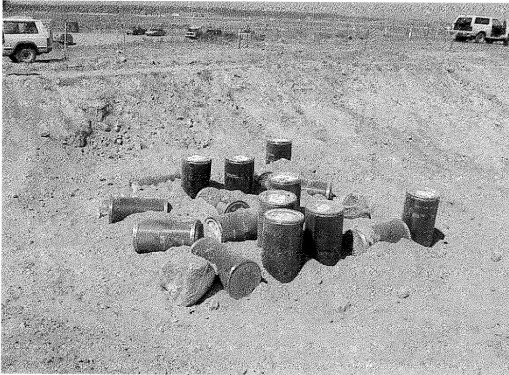
Figure 33. Layer 3, surrogate waste orientation 1.2–1.8 m (4–6 ft).
