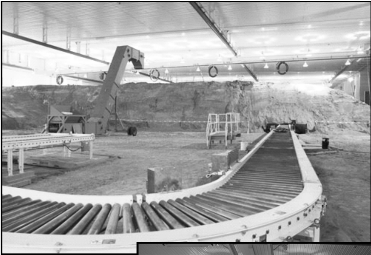
Figure 22. Transuranic Storage Area waste retrieval operations in the Advanced Mixed Waste Treatment Facility retrieval enclosure.
