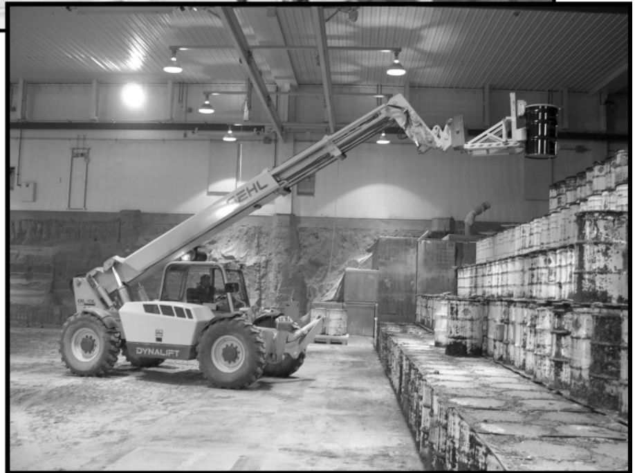
Figure 22. Transuranic Storage Area waste retrieval operations in the Advanced Mixed Waste Treatment Facility retrieval enclosure.
