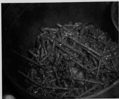
Fig. 1. Low bulk density electrorefined uranium product.
