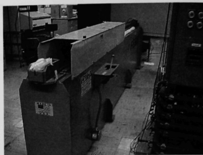
Fig. 2. Laboratory-scale hydraulic drawbench to fabricate (\text{Th,U})\text{O}_2 cermet fuel pins in CMT.
