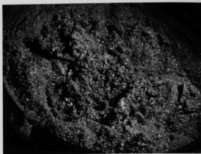
Fig. 2. High bulk density electrorefined uranium product.
