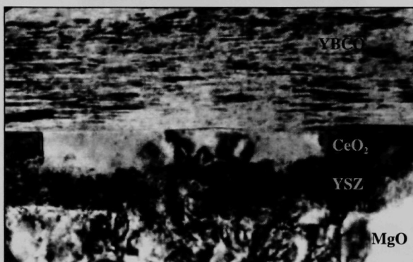
Fig. 12. TEM cross-sectional image of YBCO film deposited on YSZ- and \text{CeO}_2 -buffered ISD MgO on HC substrate.
