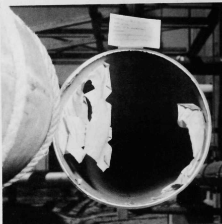
Figure 5. View of 12-inch Stainless Steel Sodium Line with Remnants of Temporary Paper Plug Used during Welding.
