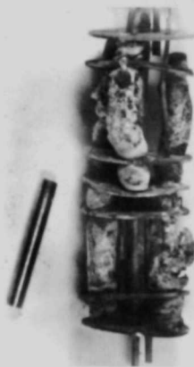
Figure 4. Uranium-fissium alloy specimens after irradiation while still in holder in which they were irradiated and oriented as shown in the autoradiograph in Figure 3. The object at the lower left is a length standard.
