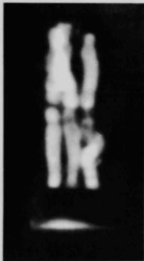
Figure 3. Autoradiograph taken before the capsule containing the specimens shown in Figure 4 was opened. The orientation of the specimen is the same as in Figure 4. The radioactive material below the specimen is Al-0.5 w/o Co alloy originally adjacent to the specimens for neutron monitoring but which melted during irradiation and dropped to the bottom of the capsule.
