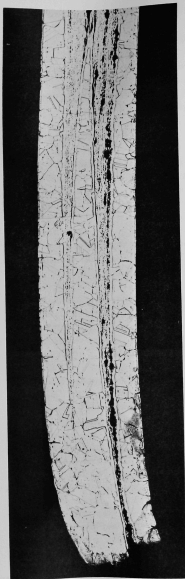
Fig. 89. Metallographic Section of Torn Lower End of Fuel Plate from Element 14, Superheater Fuel Assembly C-3, Core CSH-1
