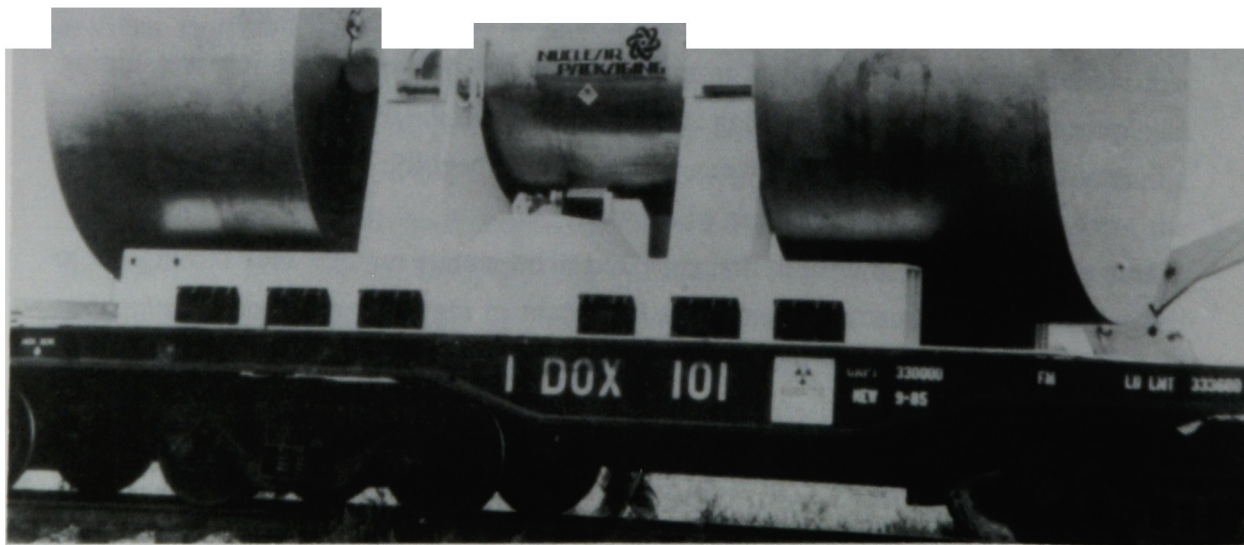
Figure 18. Exploded view of NuPac-125B rail cask and photo of cask on railcar.
