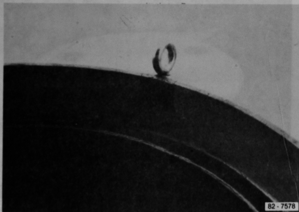
Figure 12. Top-edge detail before and after installation of lift eyes.
