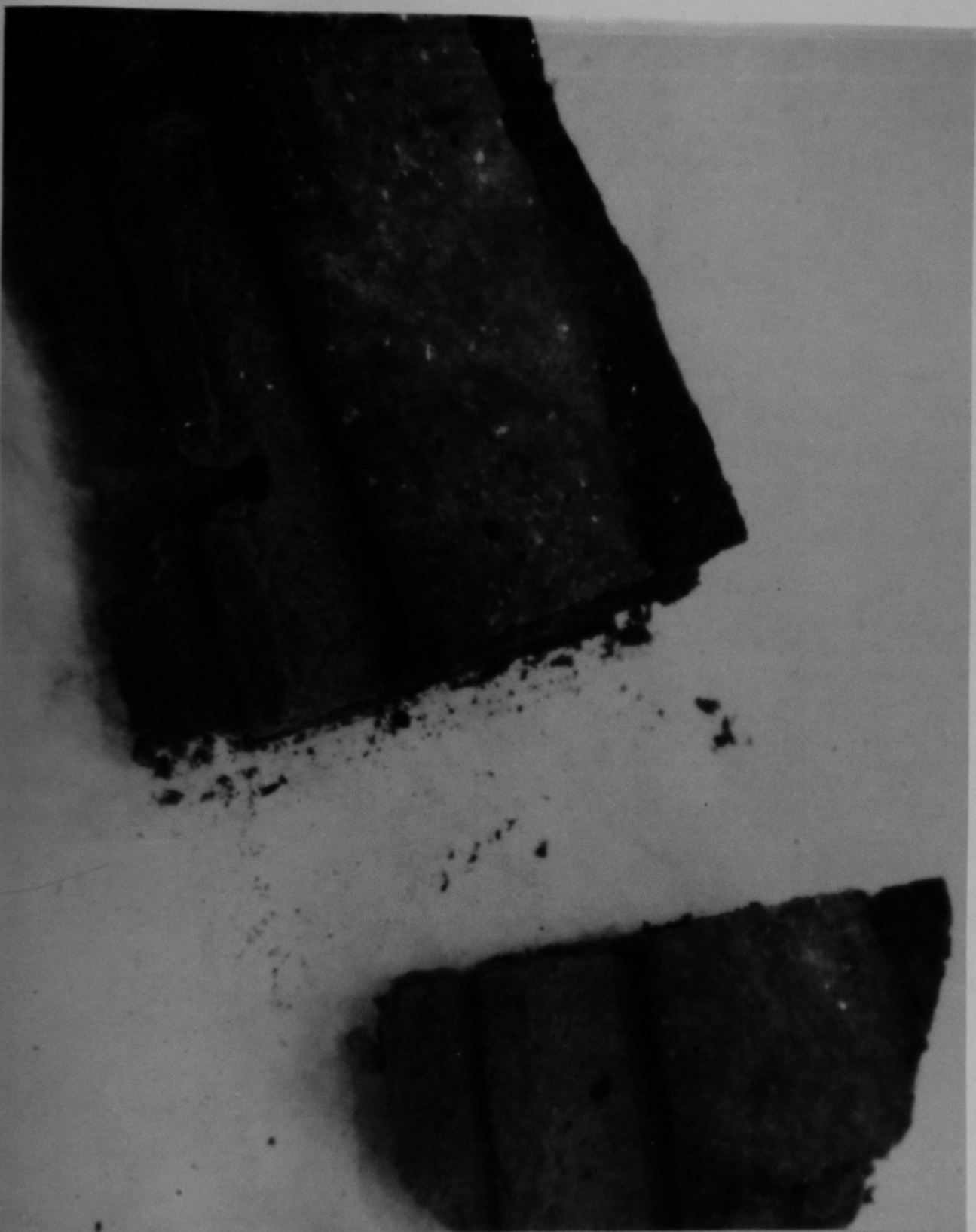
Fig. 2. MUF-2B filter sectioned for metallographic mounting.
