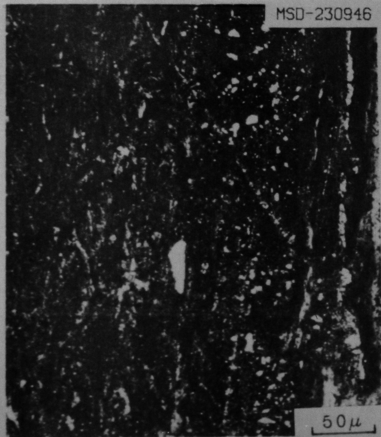
Fig. 3. Optical images of a sample of material from the MUF-4A filter that was mounted in epoxy and polished.
