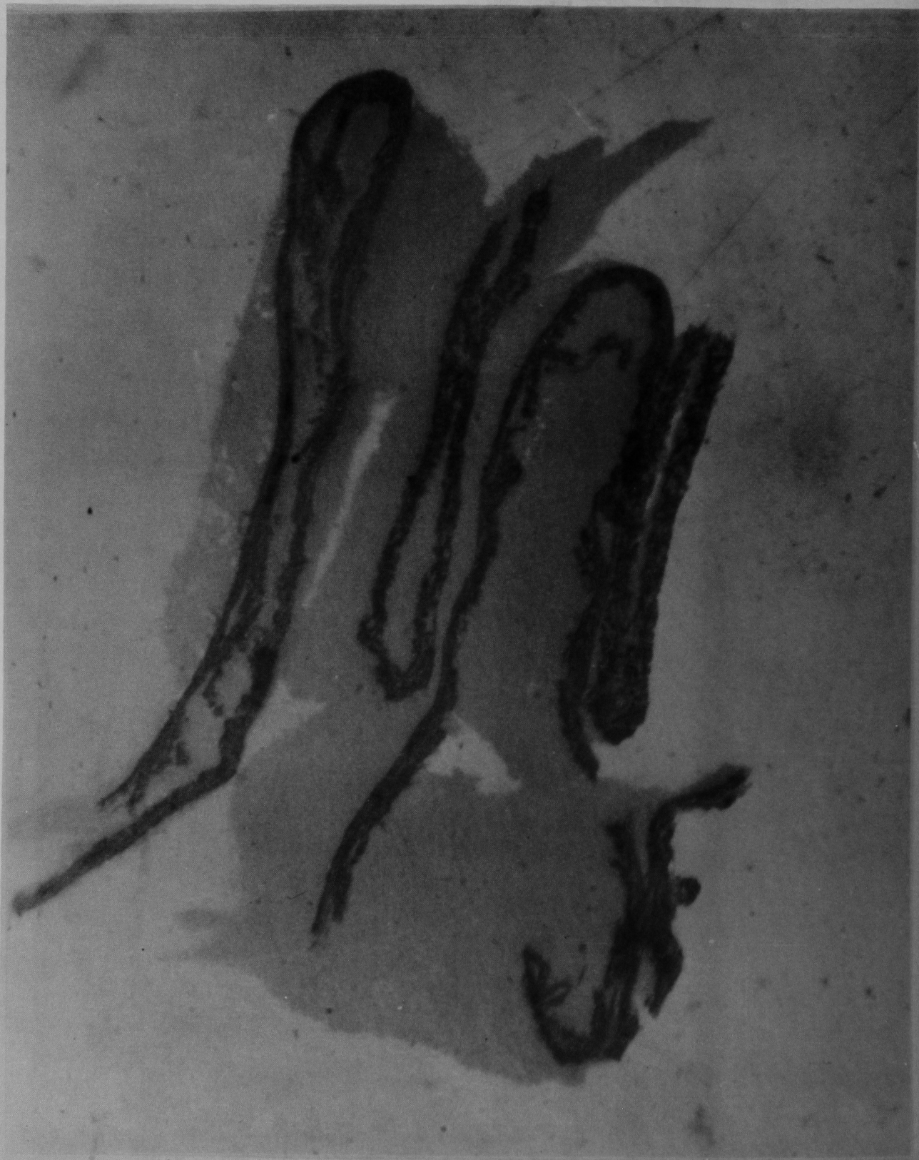
Fig. 3. Metallographically mounted section of MUF-2B filter ready for examination.
