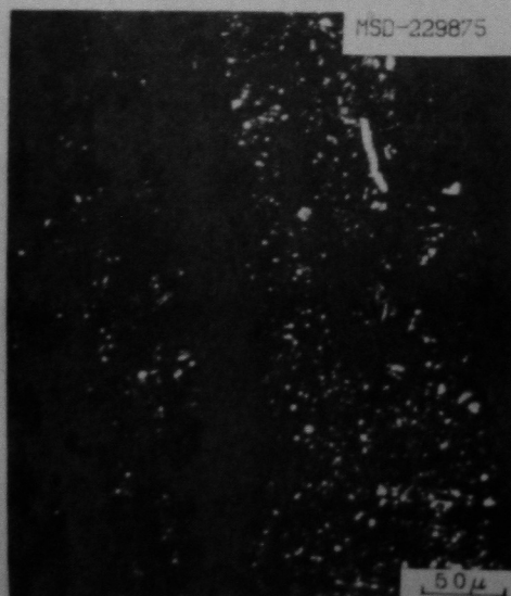
Fig. 1. Optical images of a sample of material from the MUF-5B filter that was mounted in epoxy and polished.
