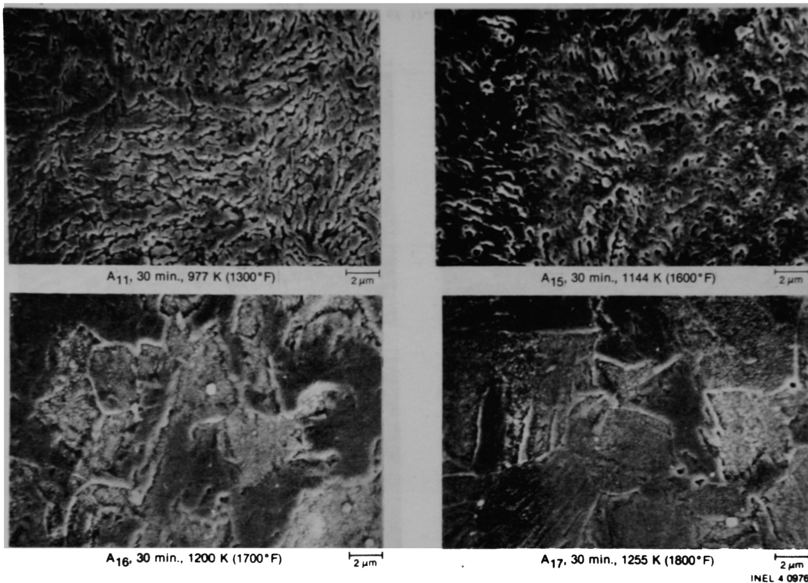
Figure A-8. SEM micrographs of 17-4 PH SS Standards A 11 , A 15 , A 16 , and A 17 .
