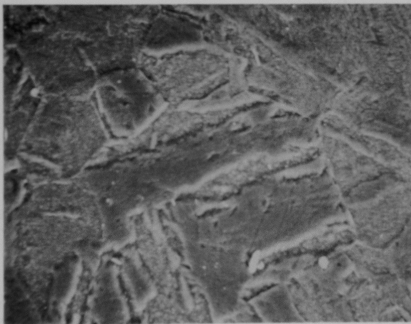
Figure 19. SEM micrograph of Sample 7a (304 SS) microstructure.
