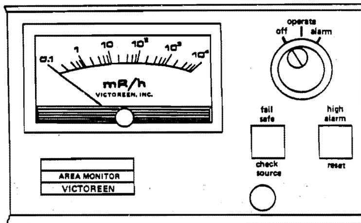
FIGURE 8. Rateometer Face. The Victoreen channel measures radiation rates of from 0.1 to  $10^4$  mR/H.
