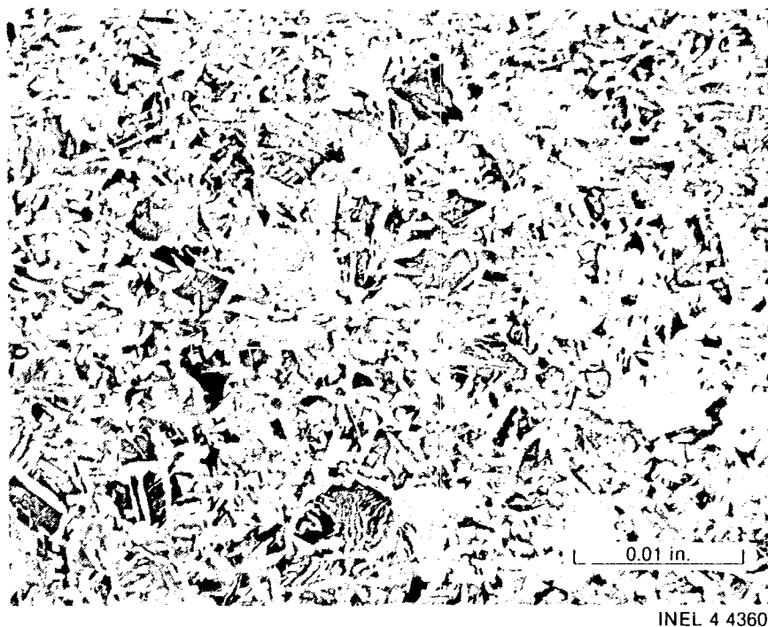
Figure 42. Photomicrograph of the base metal taken from the bottom plate of Section 4, Specimen 11 from liner PF-16 showing pearlitic (black) and ferritic (white) structures (ASTM duplex grain size No. 6 to 8).
