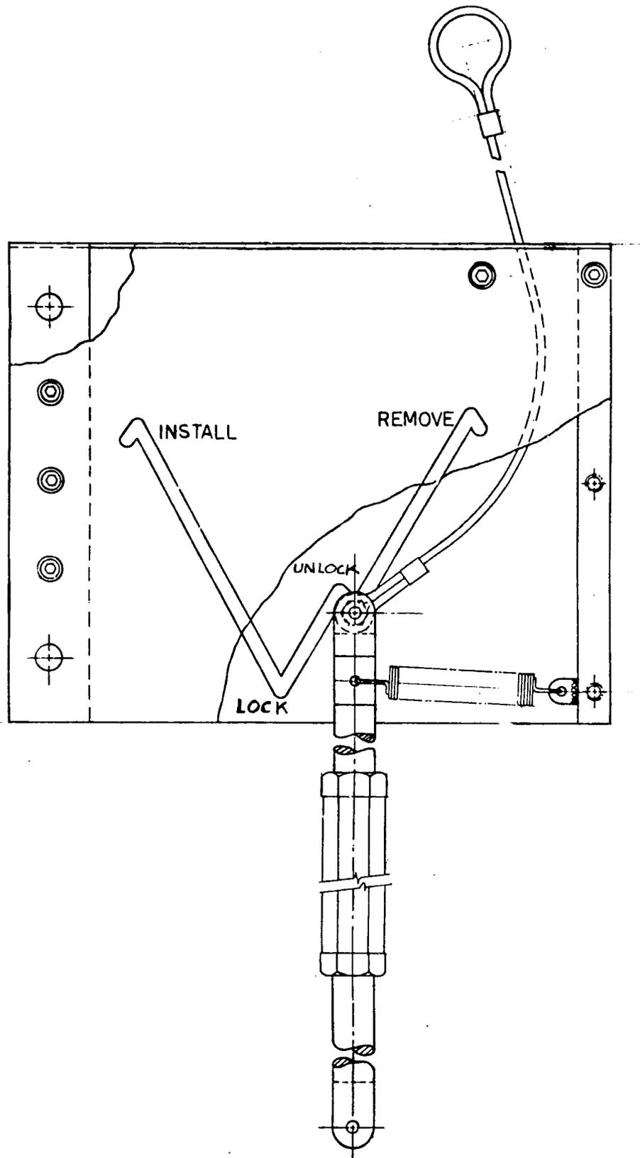
Figure 5 Pendant Latch/Unlatch System
