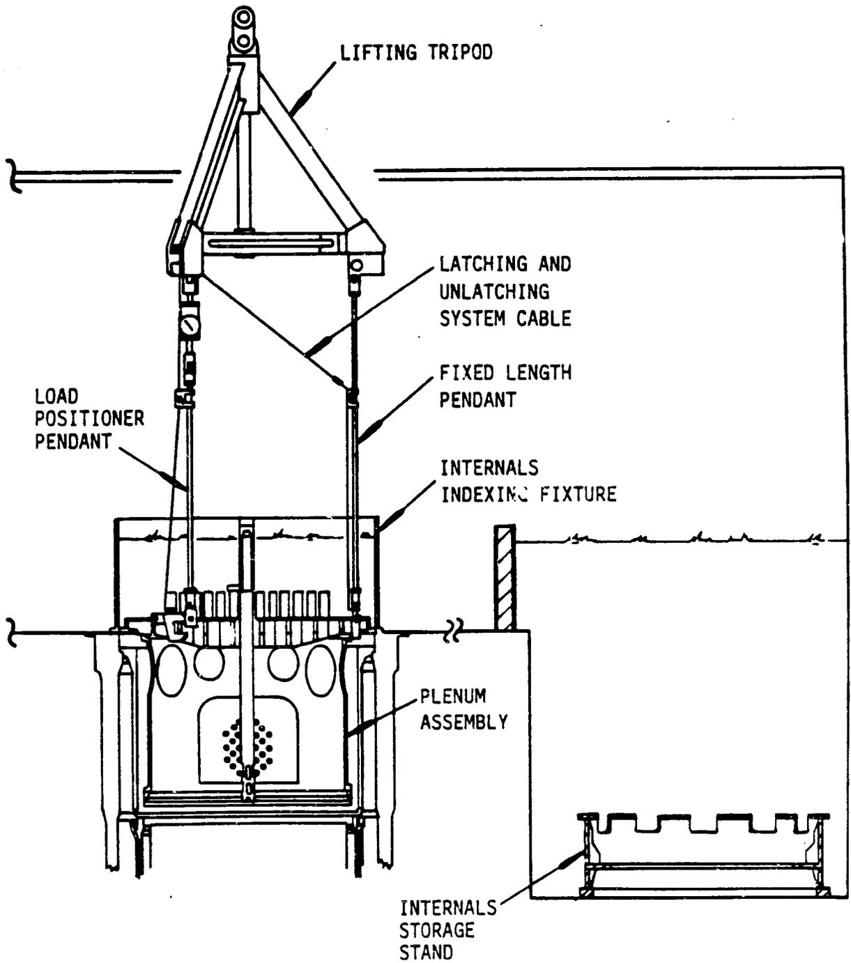
Figure 2 Plenum Lift General Arrangement
