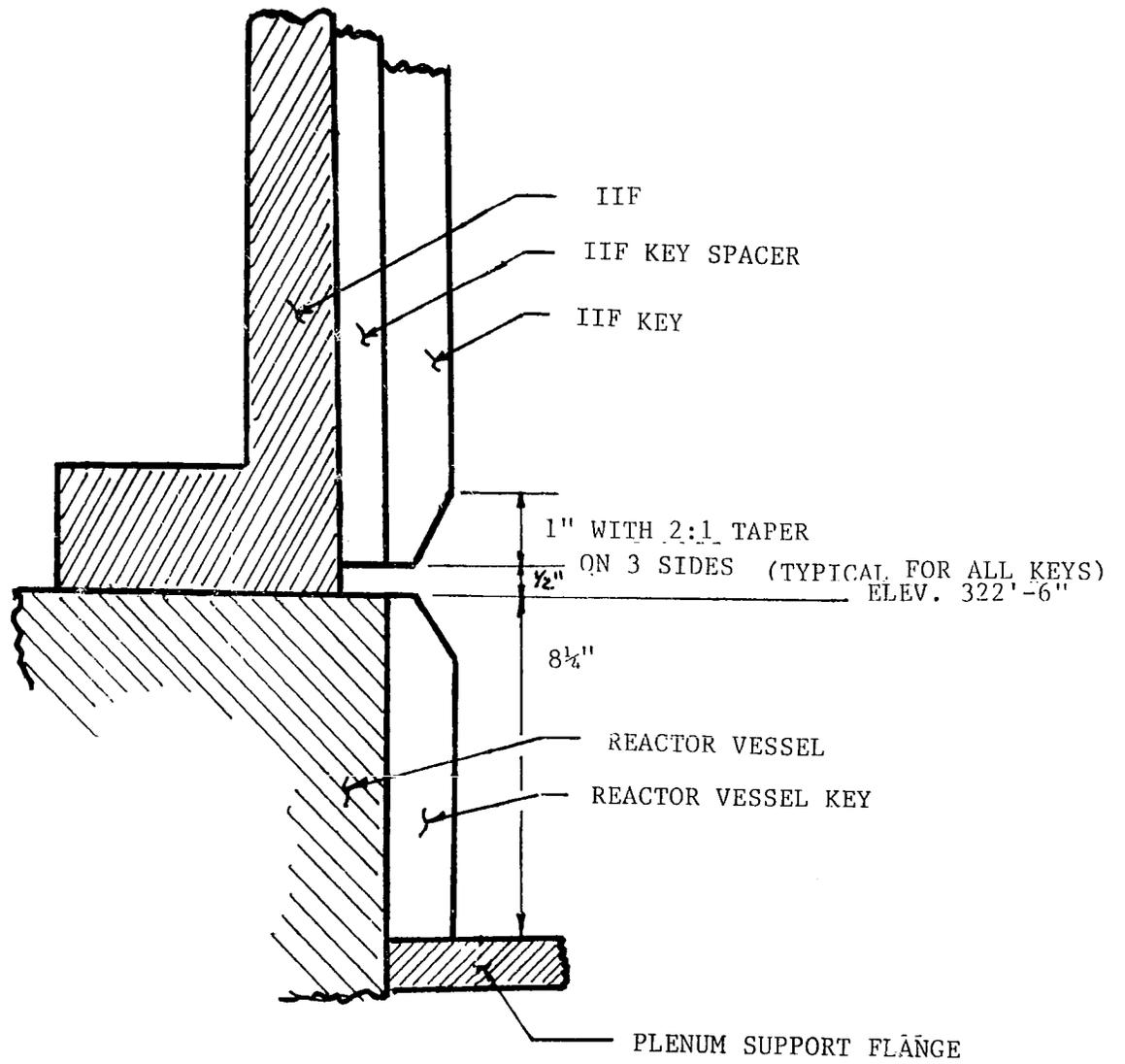
Figure 14 Reactor Vessel/IIF Key Transition
