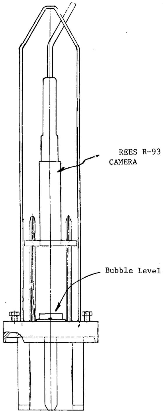
Figure 9 Bubble Level Fixture
