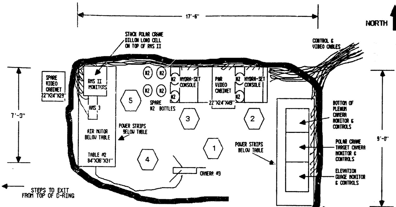
Figure 18. Shielded Lift Control Station
