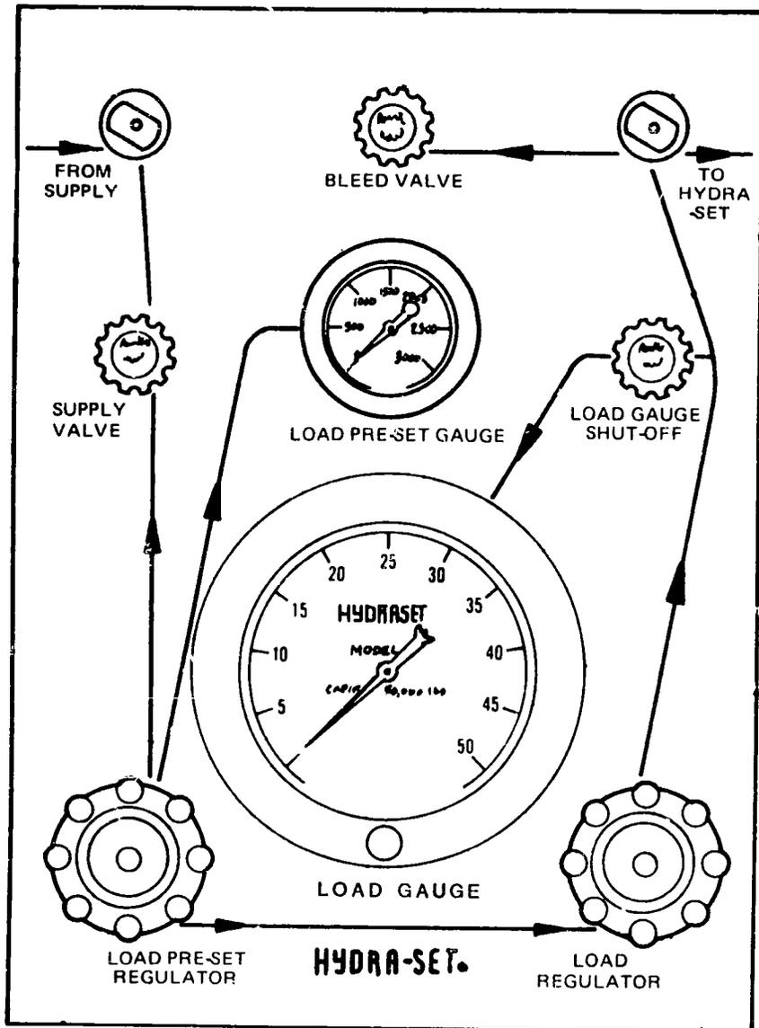
Figure 7 Hydra-Set Remote Control Console
