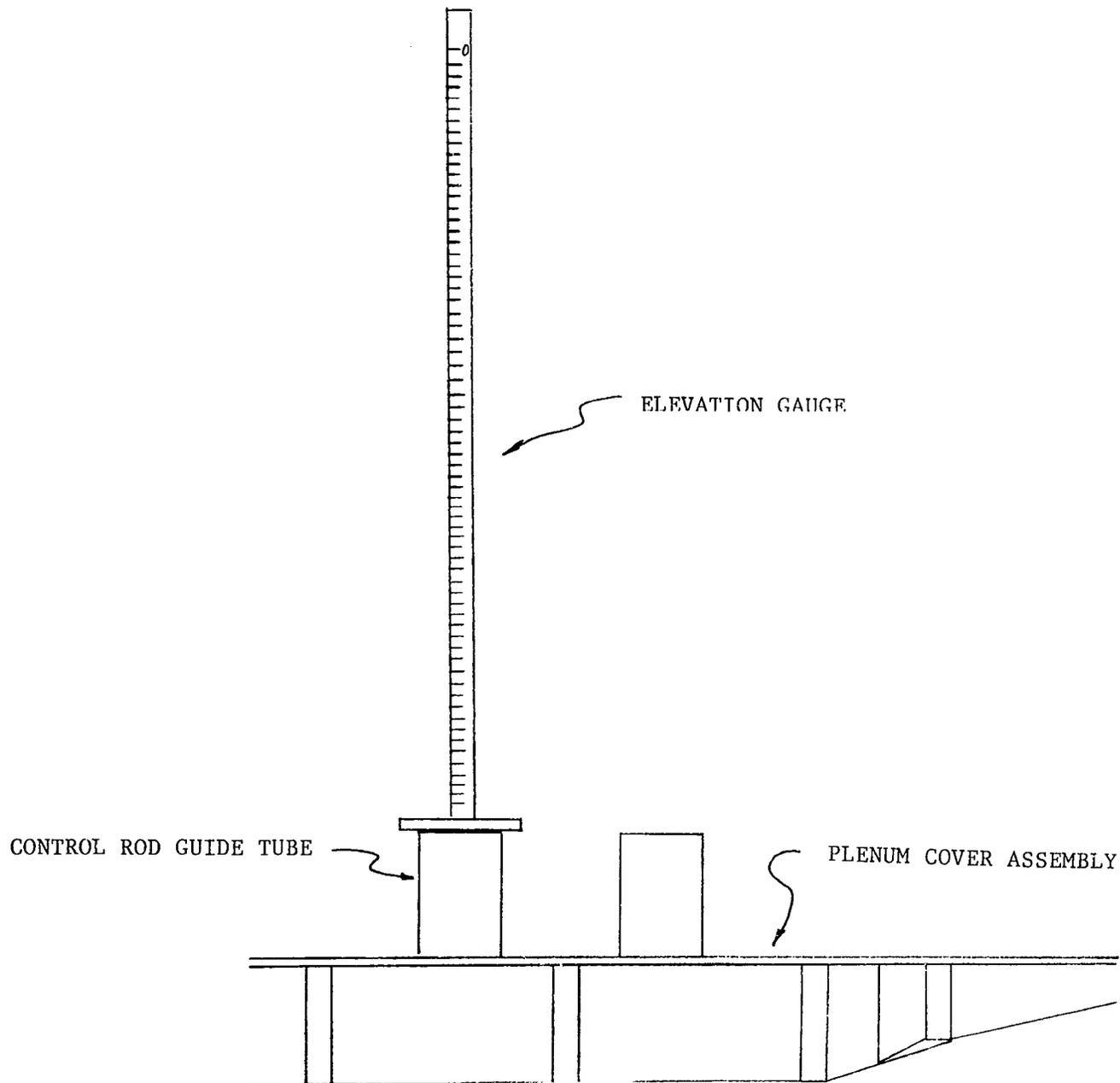
Figure 10 Elevation Gauge
