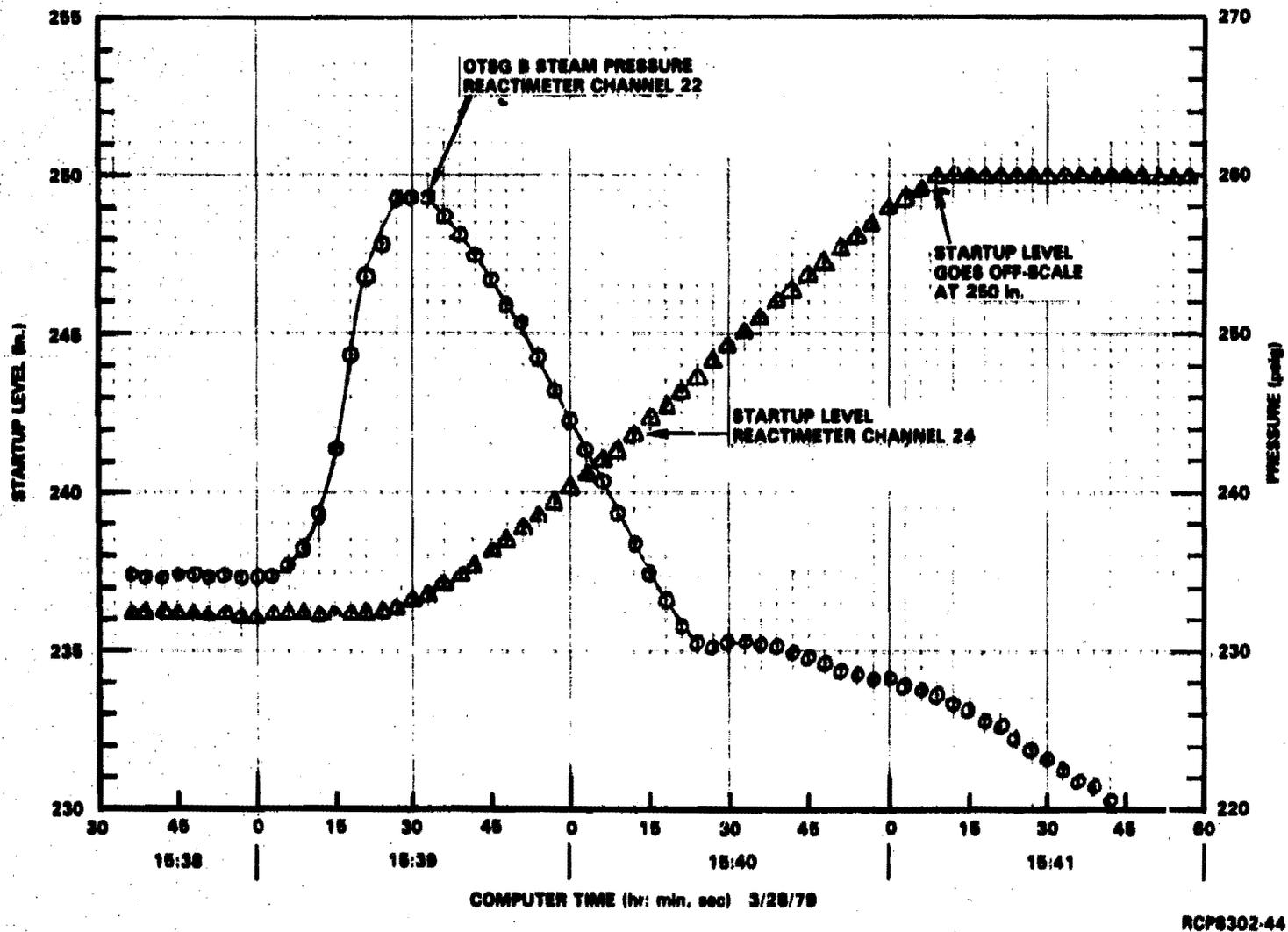
FIGURE 5. Response of OTSG B to Emergency Feed-Water Flow at 15:39.
