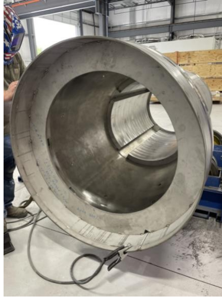
Figure 7. Fit-up of the internal shield plates to the vessel shell. Note that the supplier tack welded a temporary stiffener ring.
