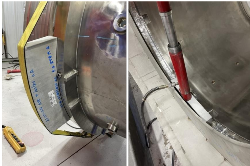
Figure 6. The top ring of the guard vessel necessitated finite tolerancing as this component served as the primary interface with the mating primary coolant system. Minimizing weld distortion in this zone was critical for functionality of the system. Note that the supplier used chill blocks on the inside (left image) and outside (right image) of the weld seam.
