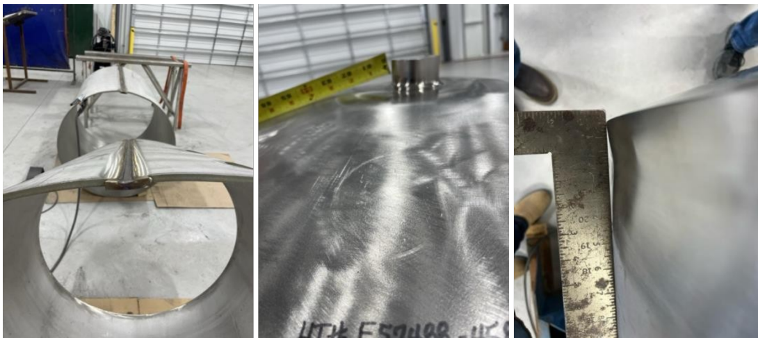
Figure 4. (Left) First occasion of weld distortion on the upper conical section of the guard vessel, where temporary attachments would have retained “roundness” and mitigated distortion (January 2024). (Center) Second occasion of weld distortion after welding the sump to the bottom cone, where the sump “sank” into the mating cone, which should have been restrained (April 2024). (Right) Third occasion of weld distortion following the welding of the lower transition ring on the bottom of the guard vessel (May 2024).
