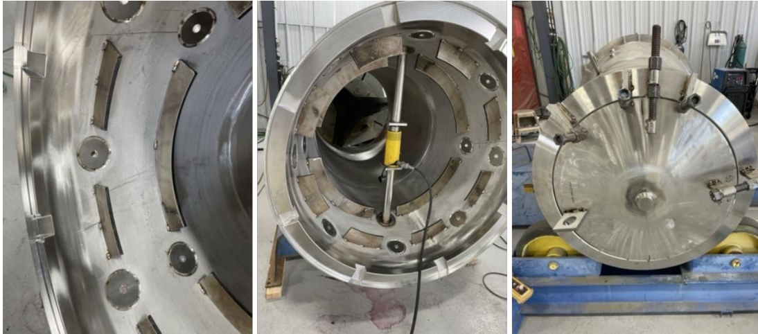
Figure 5. (Left) Strongbacks inside the guard vessel prior to welding the flanged couplings (April 2024). (Center) A hydraulic jack used in concert with strongbacks to maintain pressure on the flanged couplings during weld out , which prevented the “sinking” that had been evidenced on the sump plug to the lower cone weld (April 2024). (Right) Strongbacks and stiffeners prior to welding of the bottom cone of the guard vessel (August 2024).
