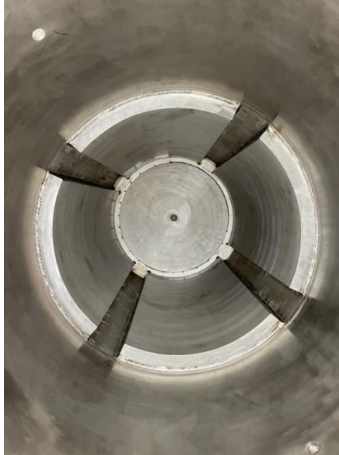
Figure 10. Completed fillet welds on the internal shield plates.
