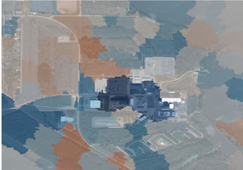
Figure 5. Explainability analysis of a nuclear generation plant in Minnesota. Red areas indicate negative correlation, and blue areas indicate areas of positive correlation. (Imagery © 2022 Maxar)
