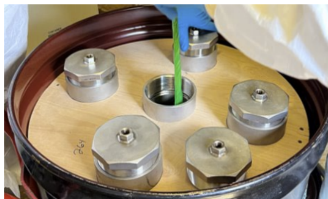
Fig. 12. A Pu-238 production target being loaded into a shipping container capable of holding 5 targets. Note the removed cap from the center position in the 5 o'clock position. [21]
