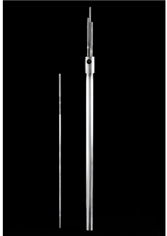
Fig.5. Partially loaded targets and target holder.[13]
