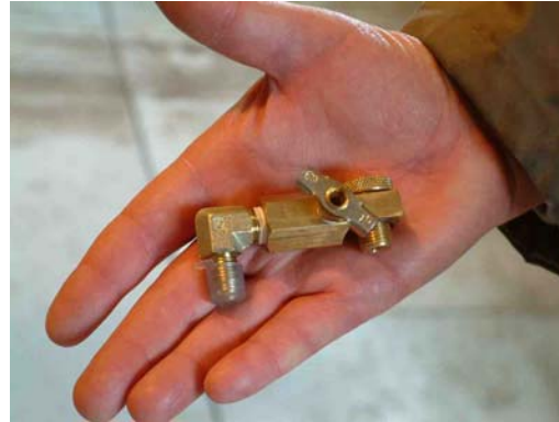
Figure 14. New puraDYN orifice assembly with oil analysis sampling valve.
