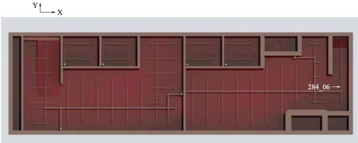
Figure 119 – Leakage Locations for the First Time History in Y Direction– PGA normalized to 1.2 g.
