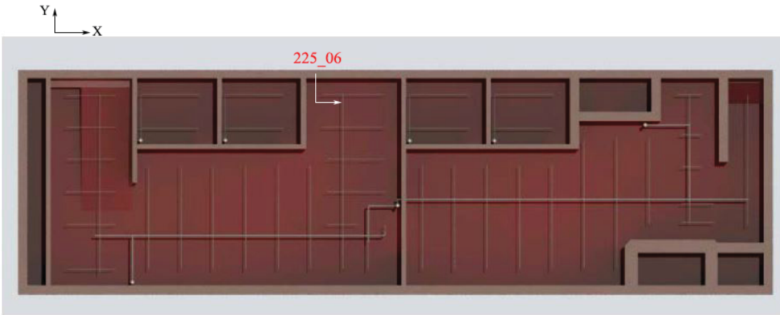
Figure 25 – Damage Locations for “Parkfield” Earthquake – 0.3 g.
