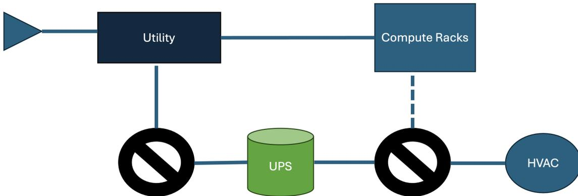
Figure 4: The UPS Configuration implemented for the microreactor peak shaving strategy. In this approach, the HVAC is wired directly into the UPS where everything else is connected to utility power. The dashed line indicates the potential to also power the compute racks from UPS in the event of utility failure, which was not tested in this study.
