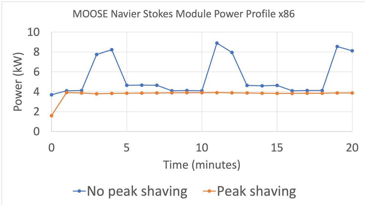
**Figure 6: Total power usage including cooling costs as a function of time for running the Navier-Stokes incompressible fluid solver on the 560 core x86 AMD EPYC cluster with and without peak shaving. In the peak shaving case, the energy storage system was the system UPS. In the first minute of operation, there is a power demand change as the system goes from idle to busy.**
