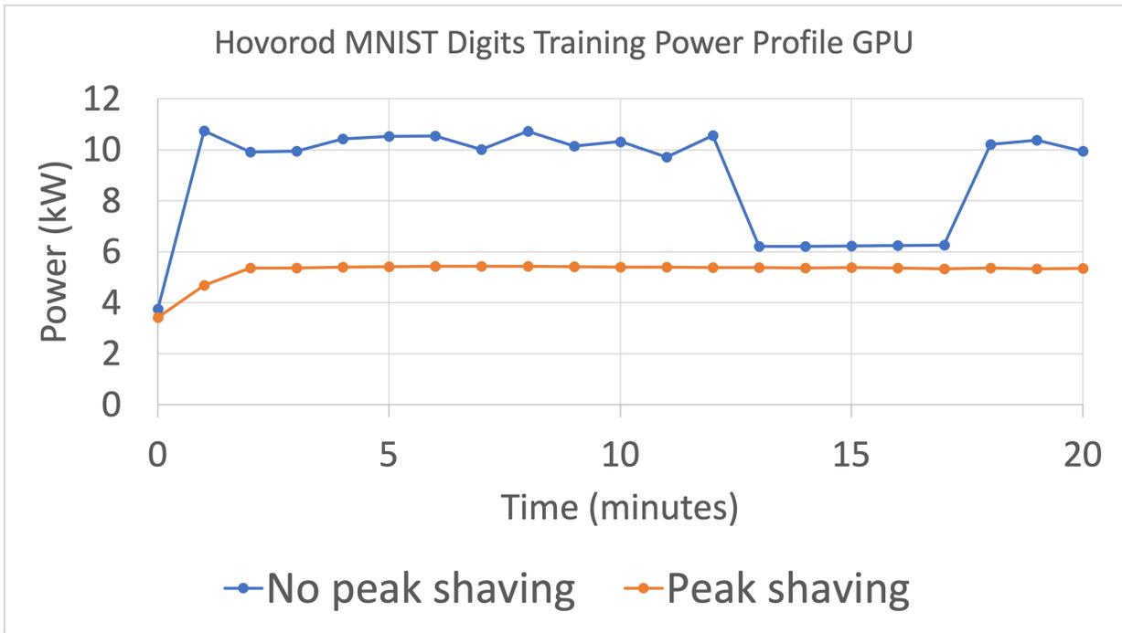
Figure 8: Total power usage including cooling costs as a function of time for using Horovod to train the MNIST dataset on the 20 NVIDIA A100 GPUs with and without peak shaving. In the peak shaving case, the energy storage system was the system UPS. In the first minute of operation, there is a power demand change as the system goes from idle to busy.
