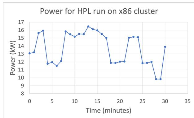
**Figure 1: Total power usage including cooling costs as a function of time for running HPL on the 560 core x86 cluster detailed in Table 1. The simulation began at the 2 minute mark and finished at the 27 minute mark. Cooling accounts for most of the variation in power usage. The ARM and the GPU clusters in Table 1 were also on but idle during this run.**
