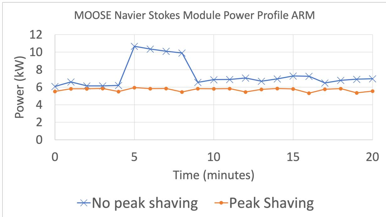
**Figure 7: Total power usage including cooling costs as a function of time for running the Navier-Stokes incompressible fluid solver on the 1536 core ARM A64FX cluster with and without peak shaving. In the peak shaving case, the energy storage system was the system UPS. There is no change for this architecture in the power demand as the system goes from idle to busy.**
