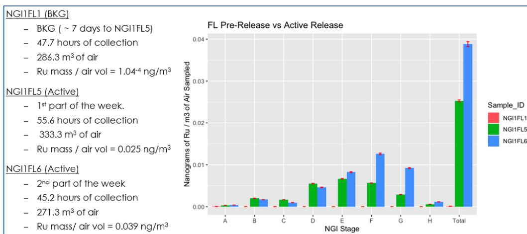
Figure 8. ICP-MS analysis of two FL NGI collection during the second week of active releases.
