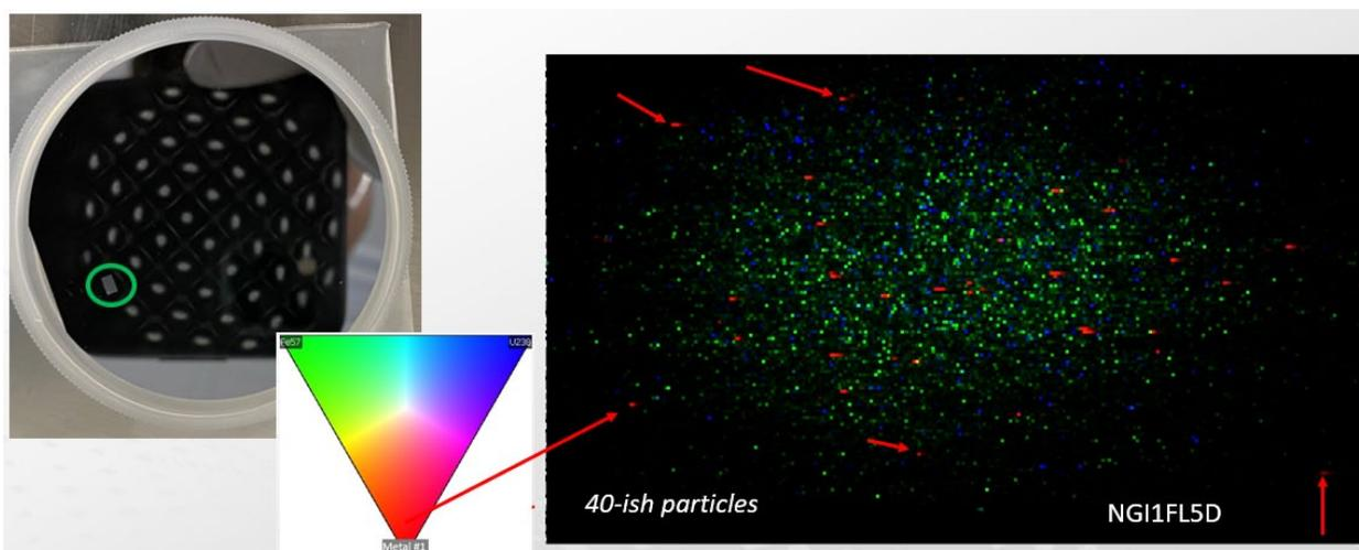
Figure 5. LA-ICP-MS analysis of a single pocket from FL NGI collector plate D. Red dots are particles containing  $^{101}\text{Ru}$ . Green are  $^{57}\text{Fe}$ -containing particles, and blue dots note particles that contain  $^{238}\text{U}$ .
