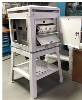
Figure 3. SRNL high-volume WAES prototype electrostatic collector.
