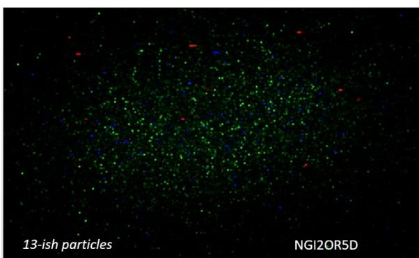
Figure 6. LA-ICP-MS analysis of a single pocket from OR NGI collector plate D. Red dots are particles containing  $^{101}\text{Ru}$ . Green indicate  $^{57}\text{Fe}$ -containing particles, and blue particles contain  $^{238}\text{U}$ .
