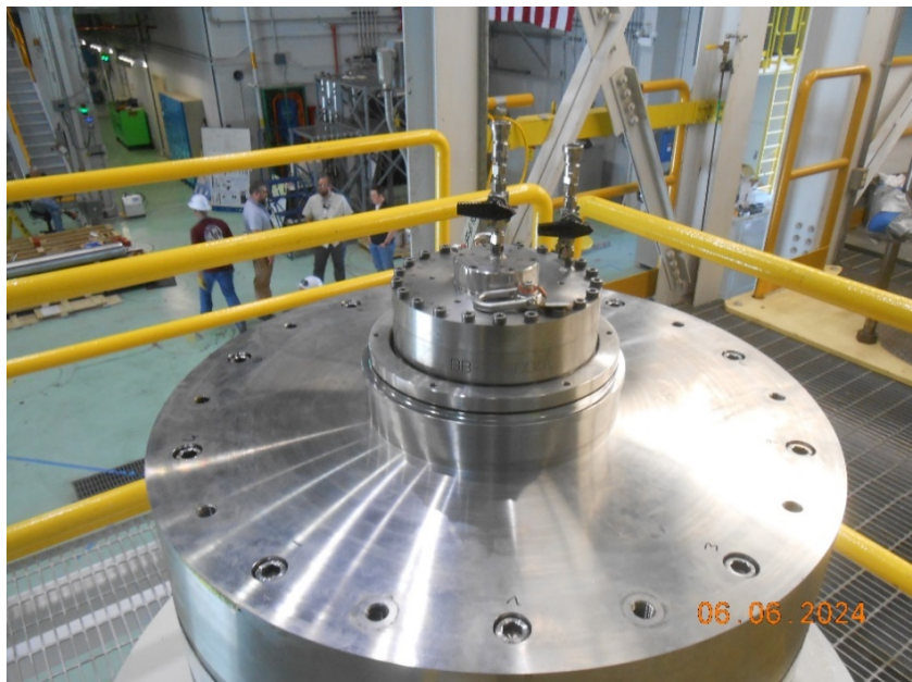
Figure 26 The HFEF-15 cask fully assembled using new components.
