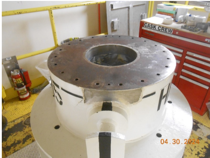
Figure 25 The disassembled and cleaned HFEF-15 cask body.
