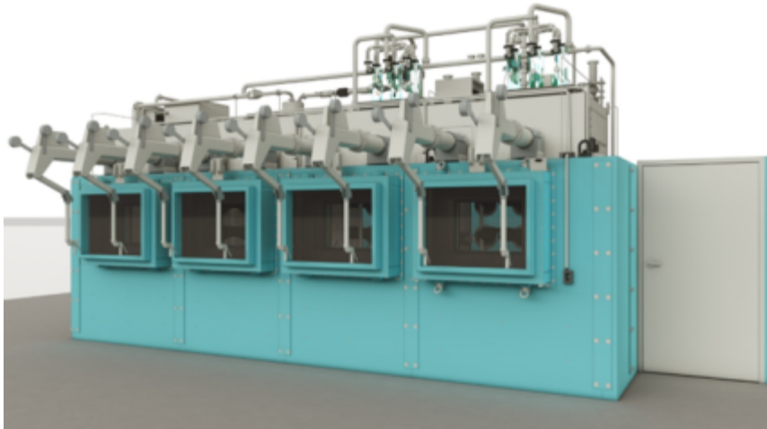
Figure 15 3D model of the MSTEC hotcell.
