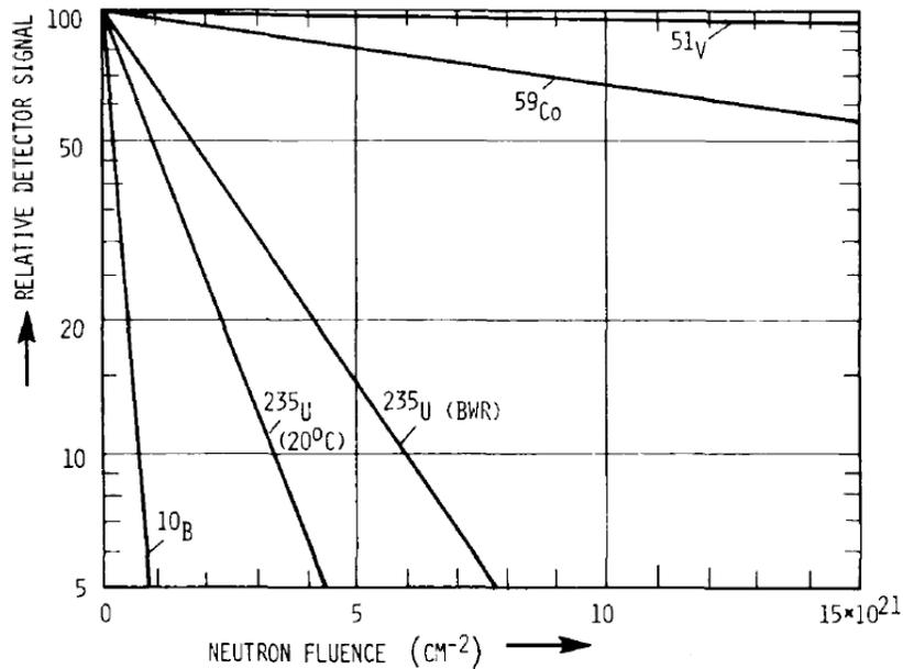
Figure 2. Detector signal degradation as a function of neutron fluence. [7]
