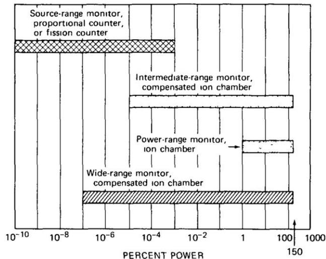
Figure 1. Typical power range separation and ex-core detector types. [2]
