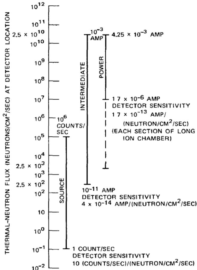
Figure A-1. Pressurized water reactor neutron flux monitoring spread.
