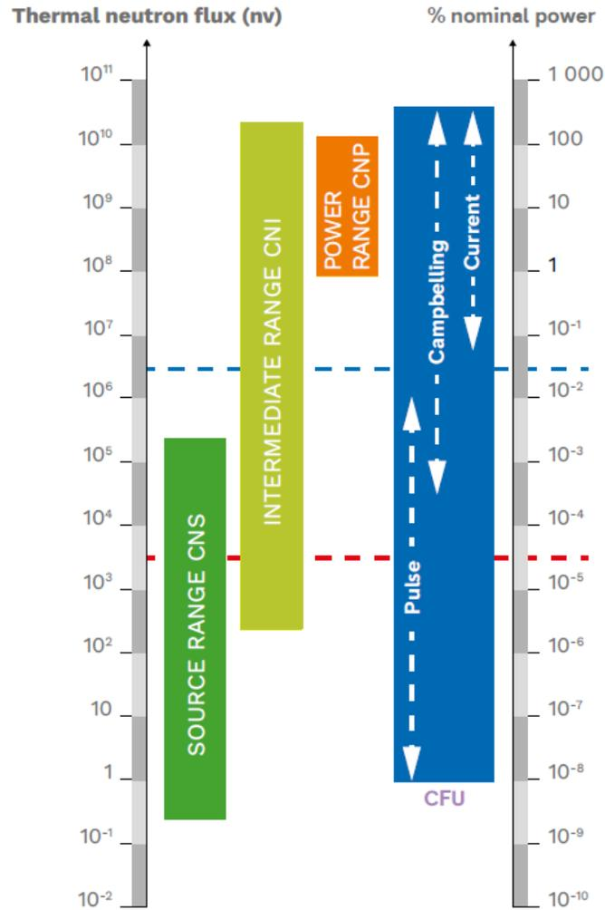
Figure A-5. Reactor power spread for power monitoring per Framatome.
