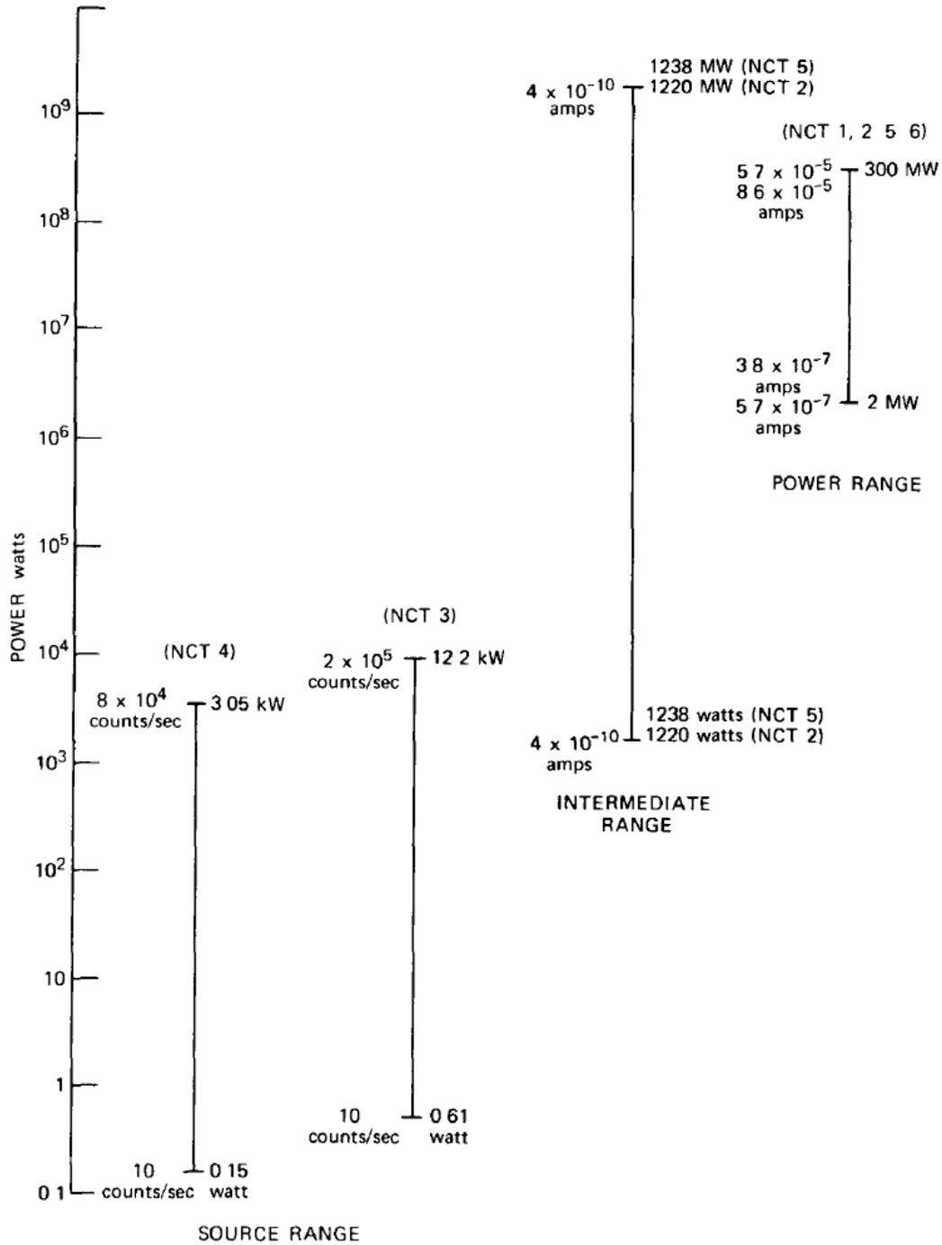
Figure A-2. Sodium-cooled reactor power monitoring spread.
