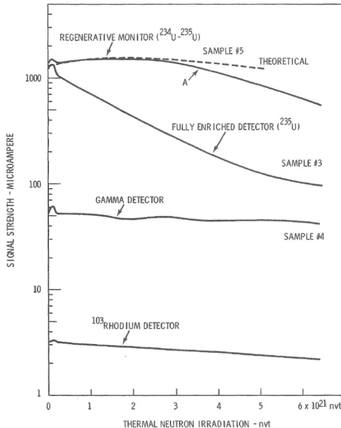
Figure 3. Detector signal for regenerative fission chamber compared to typical in-core detectors. [8]
