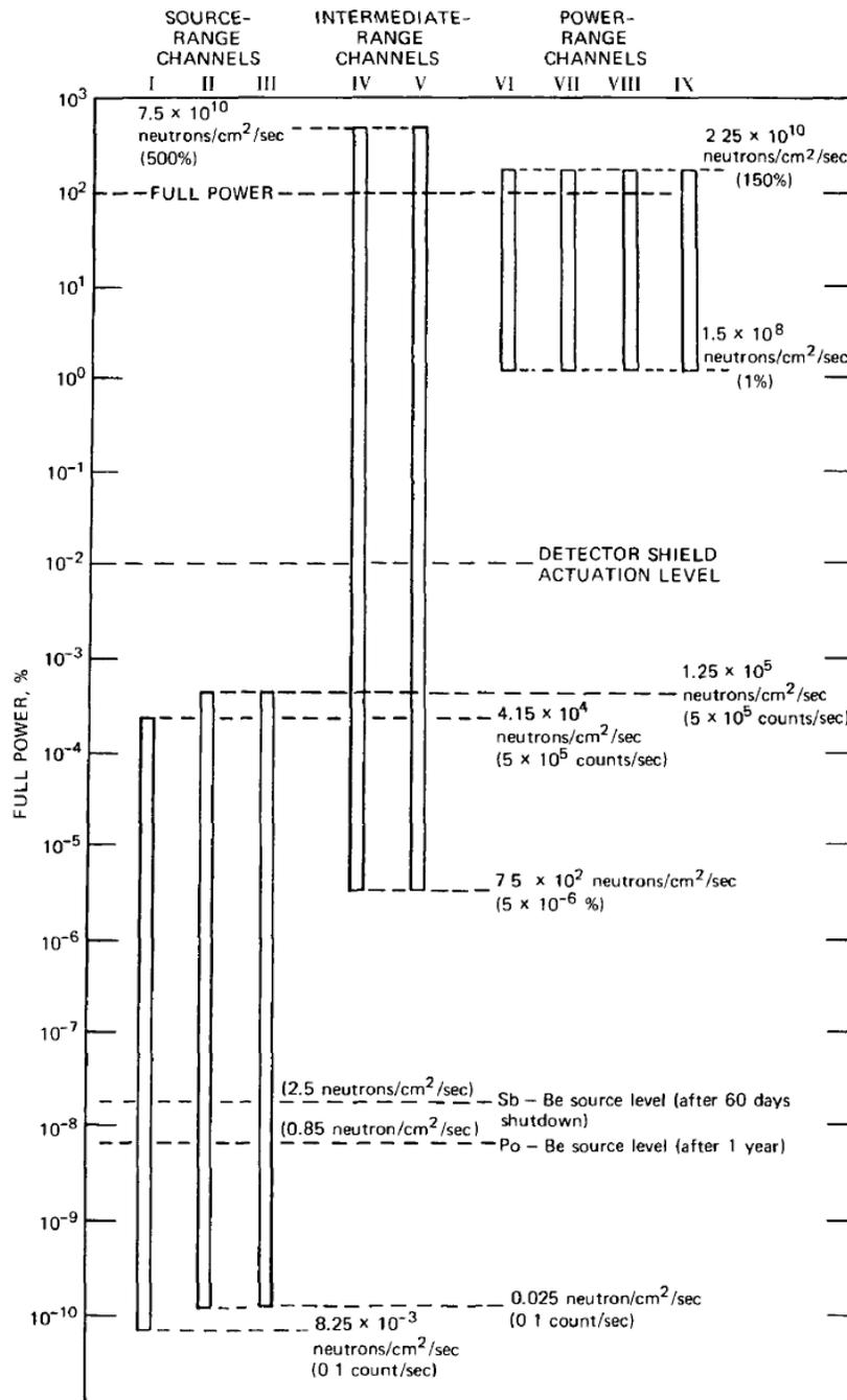
Figure A-3. High-temperature gas reactor (from Peach Bottom) power monitoring spread.
