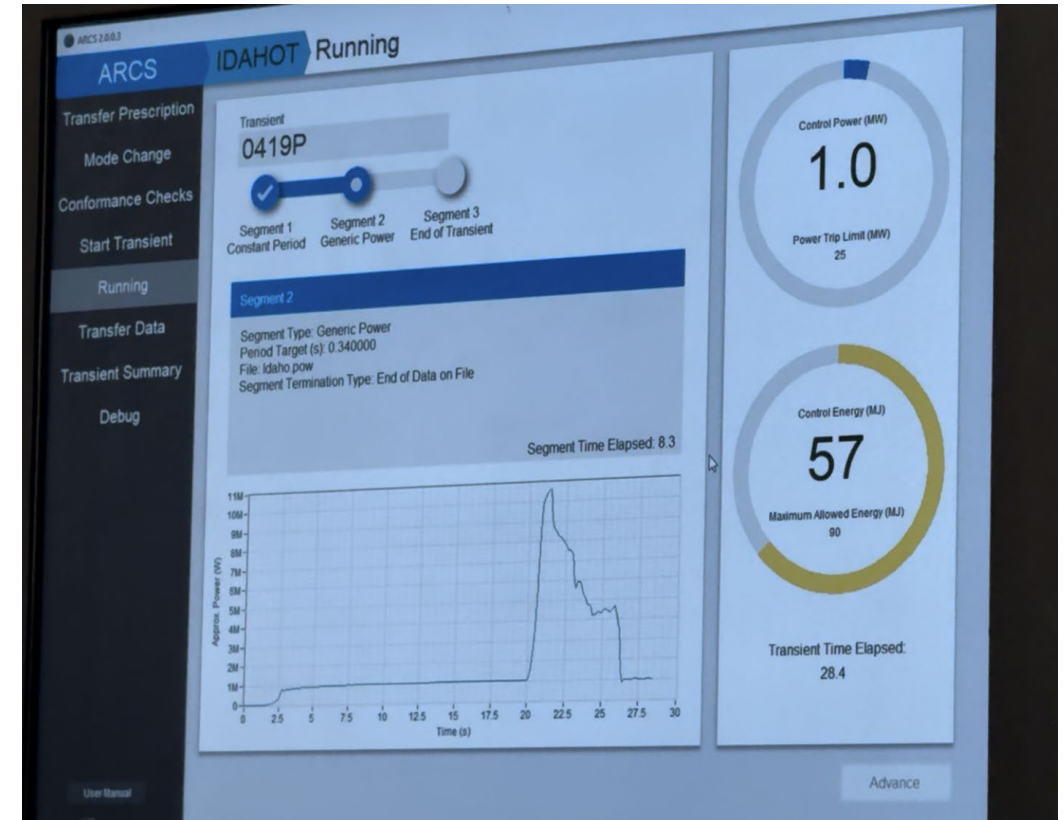
Transient using the generic power segment to create the shape of Idaho.
