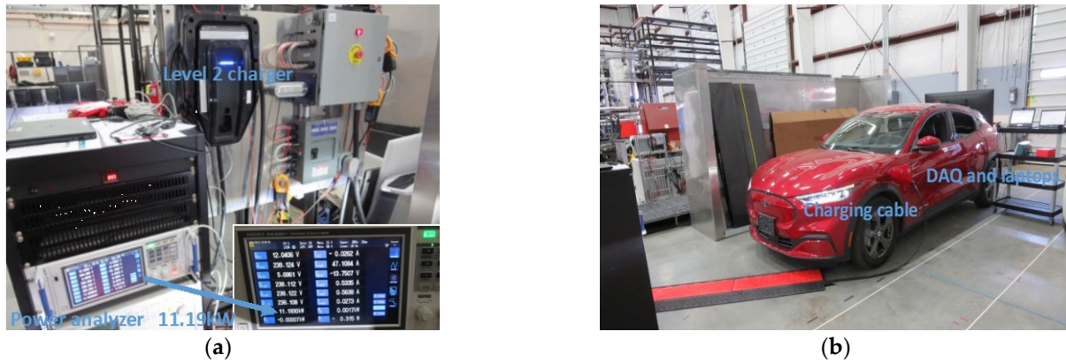
Figure 4. Lab validation of EVIRS using the Ford Mach-E. (a) Level 2 charging system with charging control and a Hikoi power analyzer, and (b) Ford Mach-E with DAQ system connected.
