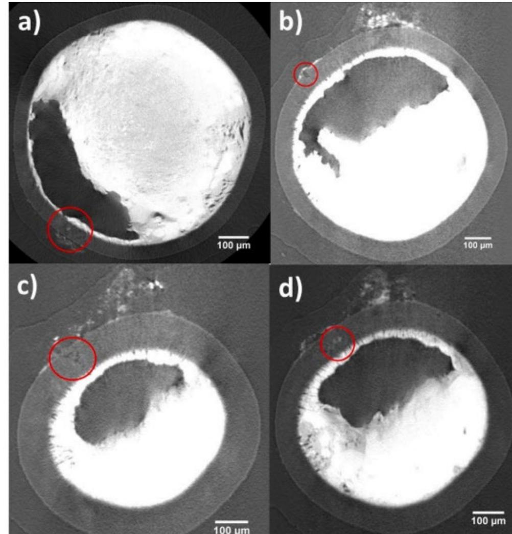
Particles from AGR-5/6/7 Compact 1-7-9. Tomographic slices from low- (top row) and high-energy (bottom row) XCT scans.
