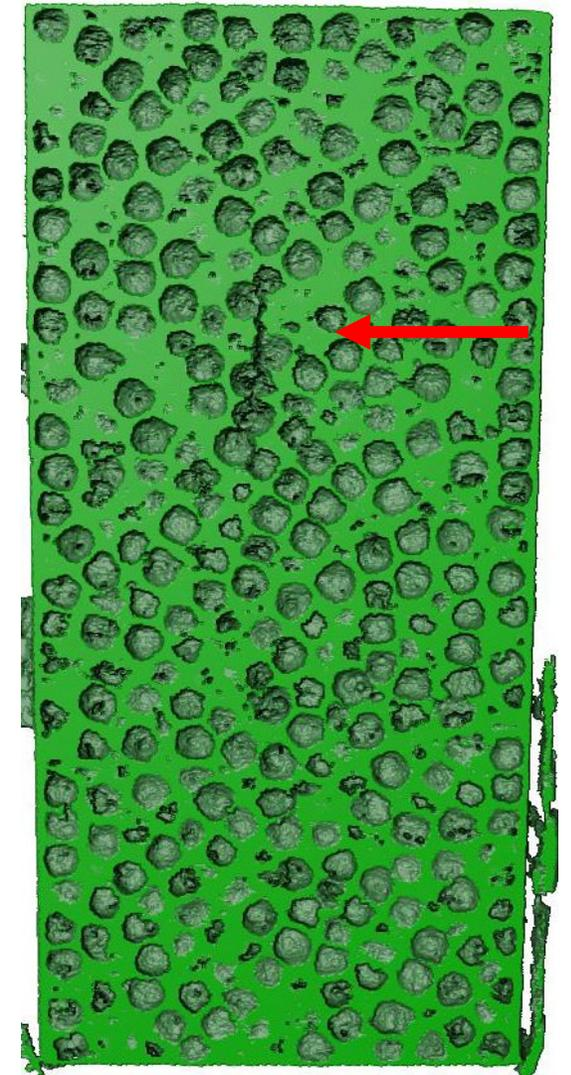
(Left) XCT slice of an unirradiated natural uranium compact, artifacts caused by X-ray attenuation prevent examination of matrix features; (Center) Neutron CT slice of the same compact, a crack is clearly resolved; (Right) A 3D rendering emphasizing the crack.
