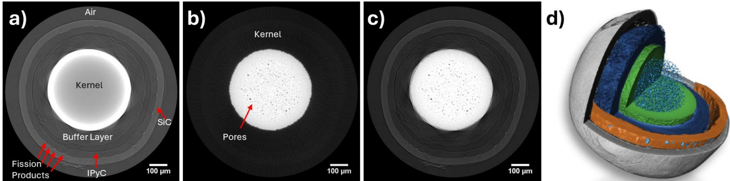
2D slices of a 3D reconstructed volume showing a) a low-energy (40 keV) scan on an irradiated AGR-2 TRISO particle, b) the corresponding high-energy (110 keV) scan of the same particle, c) the images fused together, and d) a 3D rendering of the particle using information from both datasets.
