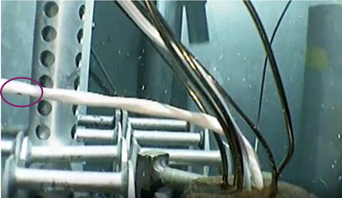
PTFE (Teflon) insulation, high temperature, water-proof, not irradiation tolerant
