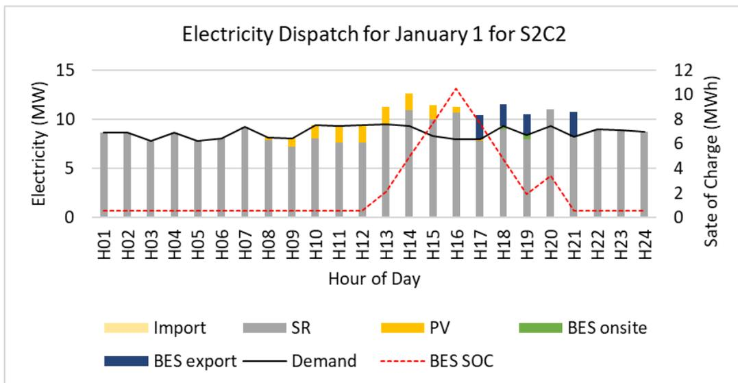
Figure 21. Time-series electricity dispatch of microgrid for January 1 for S2C2.
