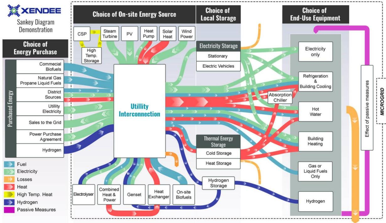
Figure A-1. Energy flows in the XENDEE optimization engine.
