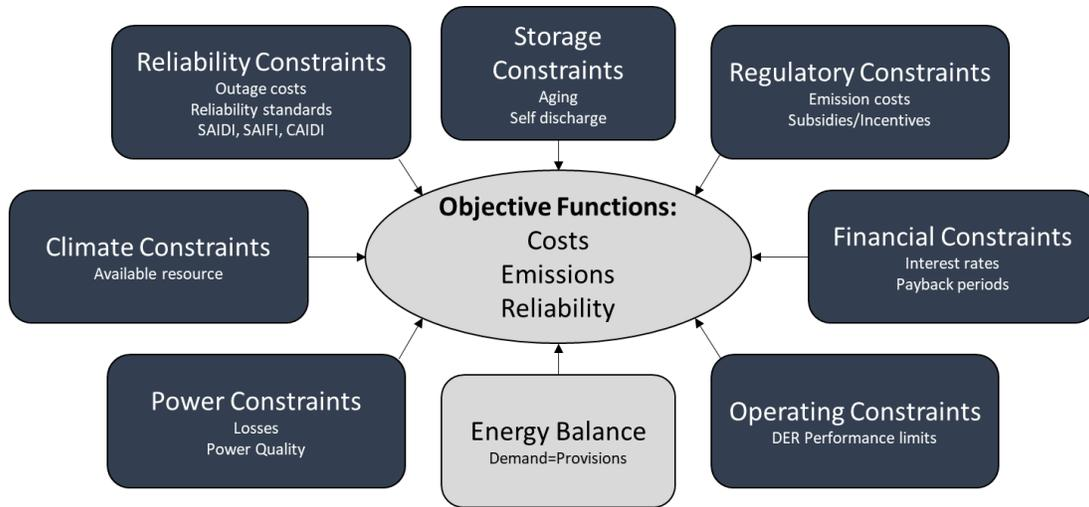
Figure A-3. Several constraints modeled in the XENDEE optimization engine.
