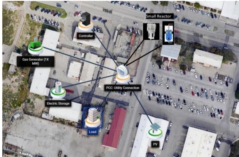
Figure 3. XENDEE single-node GIS microgrid model with potential generator options.
