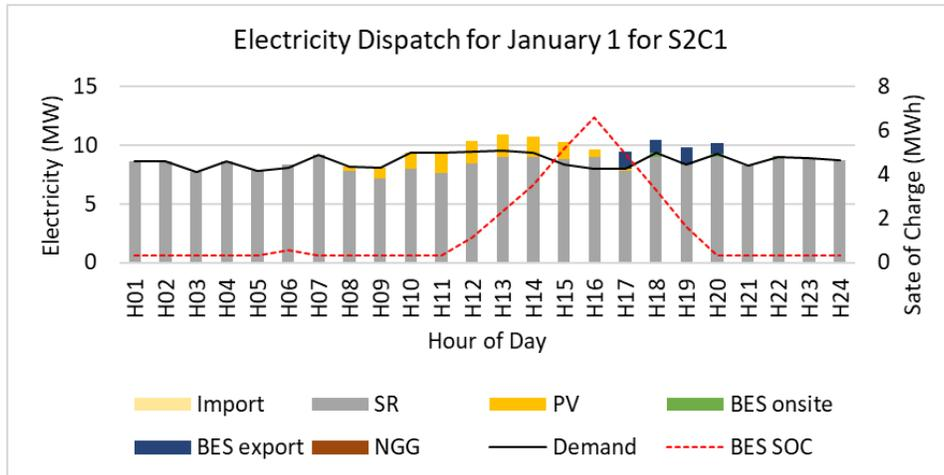
Figure 18. Time-series electricity dispatch in microgrid on January 1 for S2C1.
