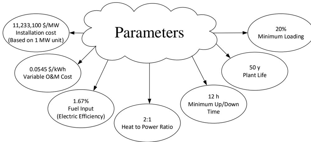
Figure 2. Parameters estimates used for the proxy model.
