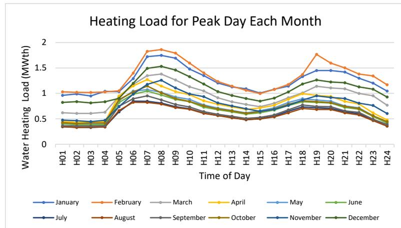
Figure 6. Time-series profile for water-heating load (shows peak day each month)
