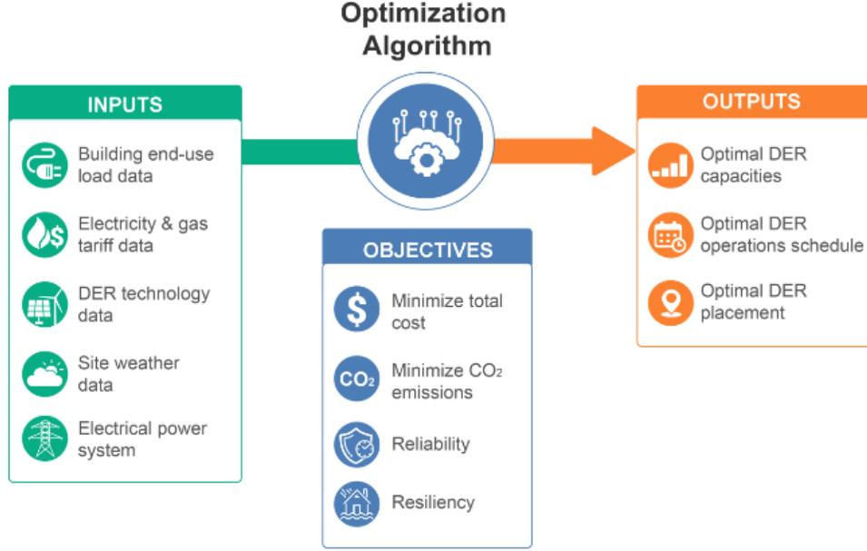
Figure A-2. The workflow of XENDEE optimization engine.
