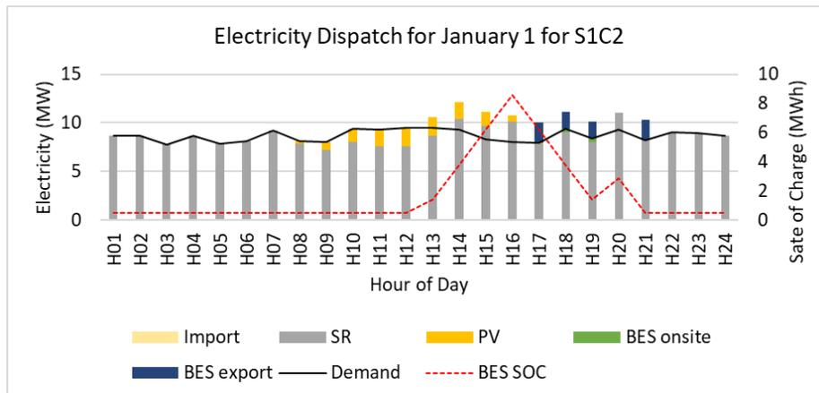
Figure 14. Time-series electricity dispatch in microgrid on January 1 for S1C2.
