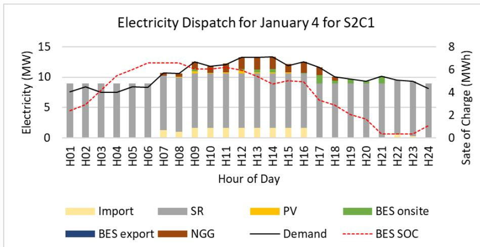
Figure 19. Time-series electricity dispatch in microgrid on January 4 for S2C1.
