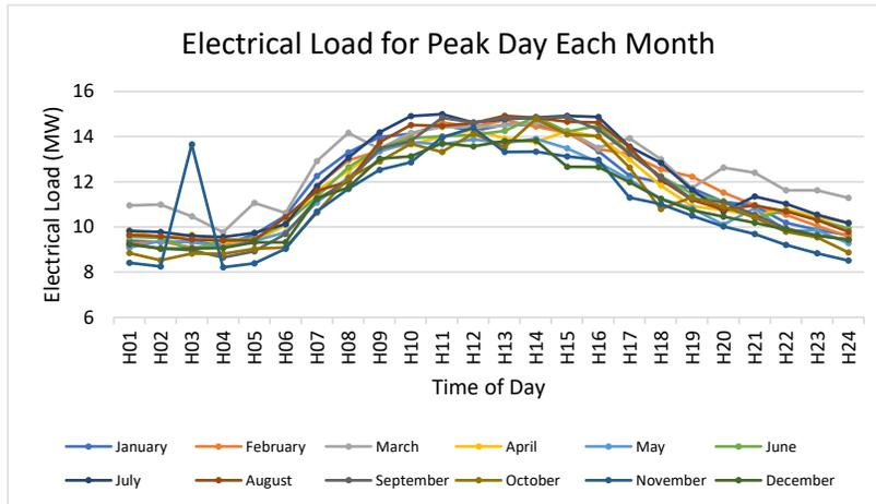
Figure 5. Time-series profile for electrical load (shows peak day each month).
