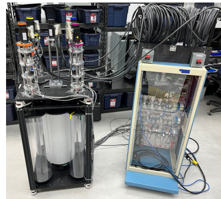
MACS Actuation System (left) controlled by Microreactor Applications Research Validation and Evaluation (MARVEL) prototype control cabinet (right).
