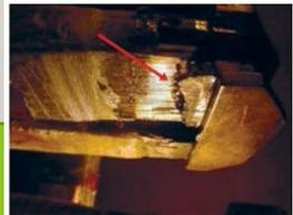
1. Broken bar was caused by absence of series blocking on an endwinding
