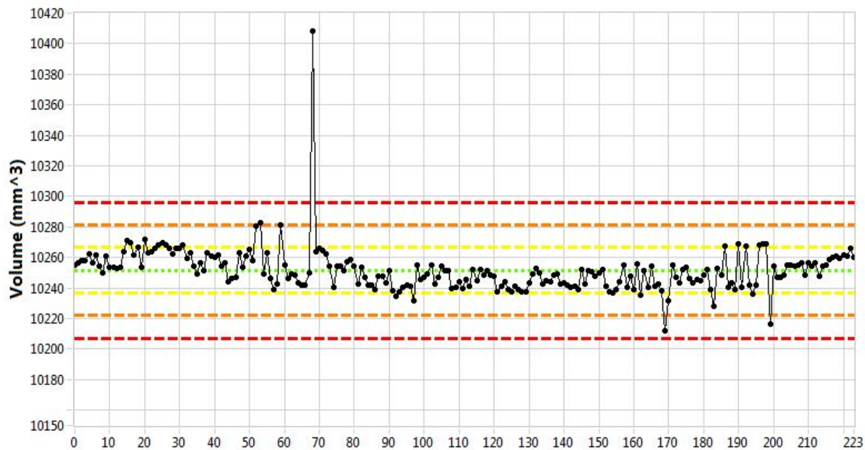
Figure B-3. Volume (mm 3 ), mean = 10251.7, standard deviation = 14.9.
