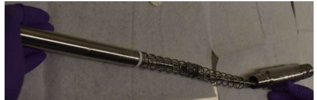
MRTI Inner Capsule w/ Springs and Top Fitting
