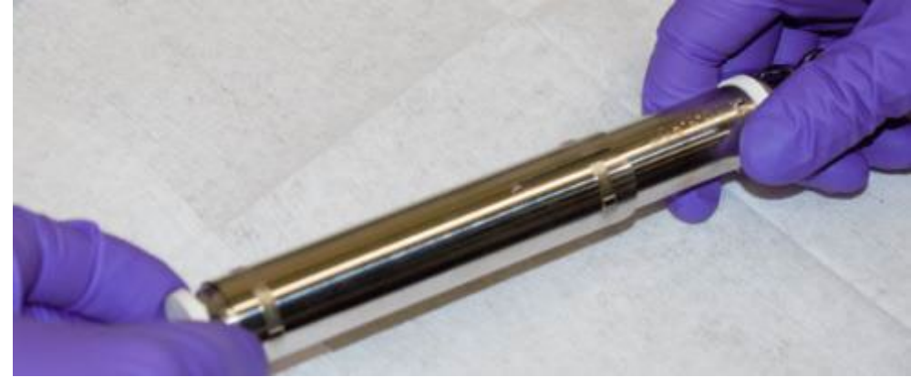
MRTI Inner Capsule w/ Springs and Top Fitting
