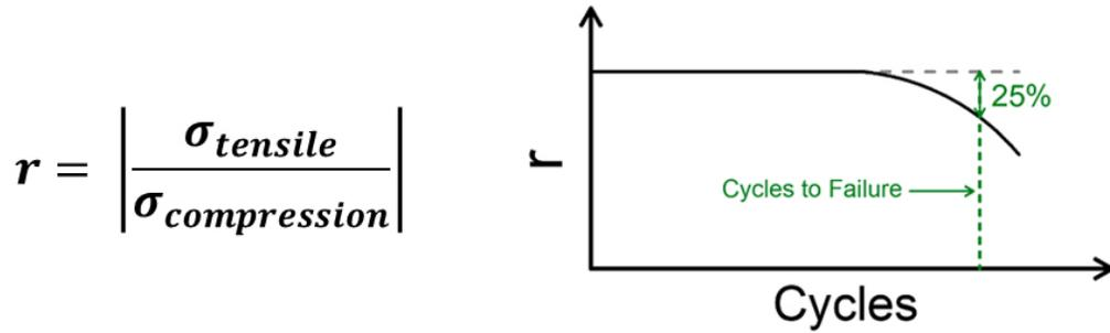
Figure 3. Evaluation criteria for cycles to failure based on a 25% stress reduction (N25).
