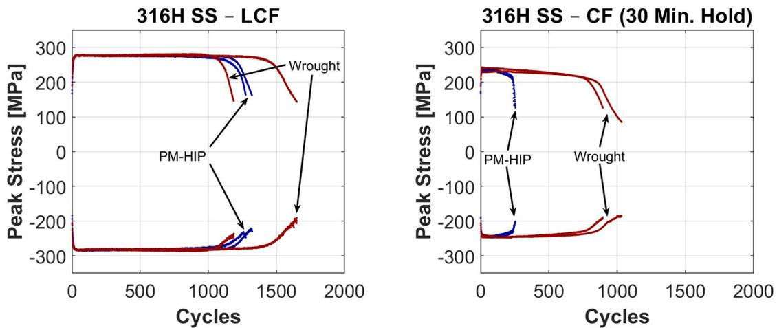
Figure 4. LCF and CF peak stress versus cycles for the UK-NAMRC PM-HIP 316H stainless steel tested at 650°C and  $\pm 0.5\%$  strain compared to a wrought 316H stainless steel.
