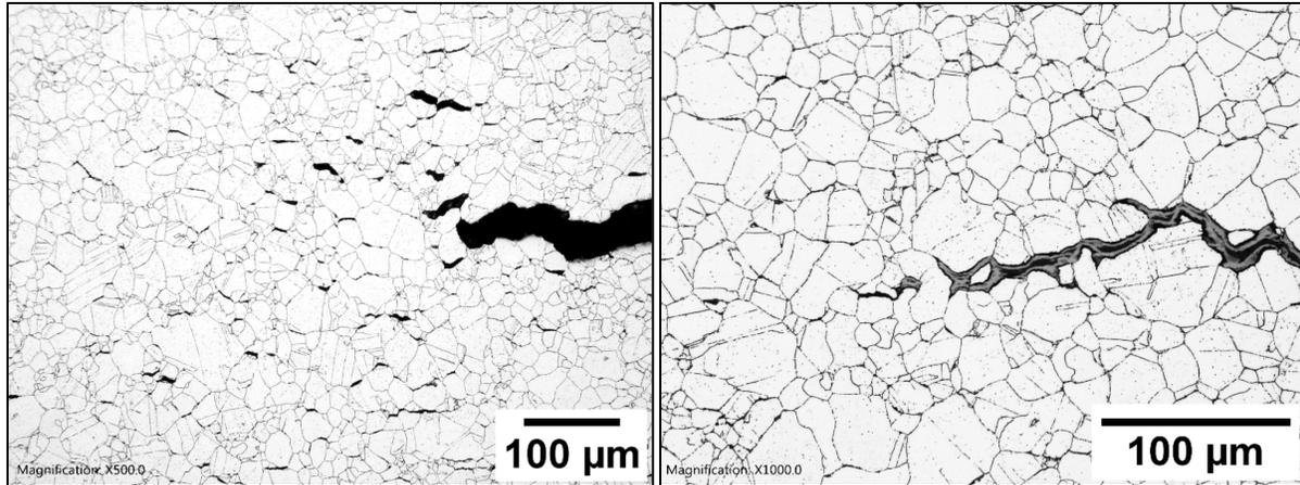
*Figure 12. Optical micrographs of the UK-NAMRC 316H stainless steel after CF testing. The left photomicrograph shows the voids ahead of the main crack, and the right photomicrograph shows another smaller crack propagating along grain boundaries (intergranular).*
