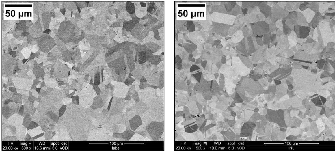
Figure 7. Backscattered electron images of the UK-NAMRC PM-HIP 316H stainless steel (left) and the MTC PM HIP 316H stainless steel (right) in the as-received condition.
