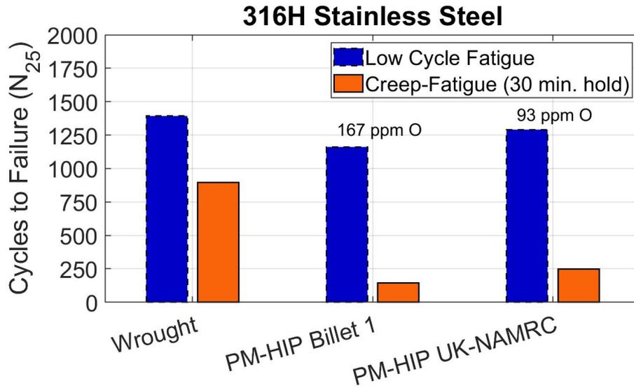
Figure 6. Comparison of cycles to failure between wrought 316H and the PM-HIP 316H materials. The reported oxygen contents are from the powder measurements.
