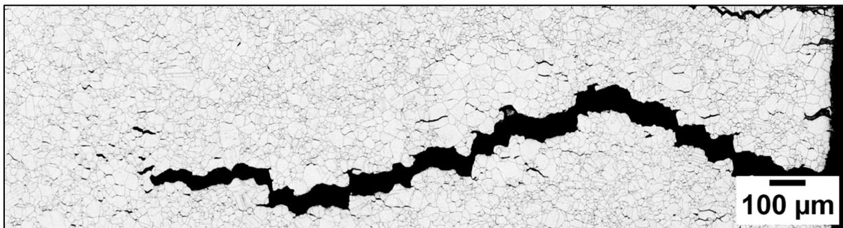
Figure 11. Optical micrograph of the UK-NAMRC 316H stainless steel from a CF test. The intergranular voids are present around and ahead of the main crack tip.
