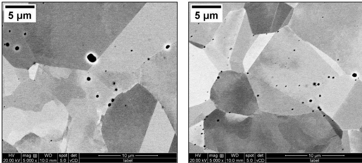
Figure 8. Backscattered electron images showing the precipitates at higher magnification.
