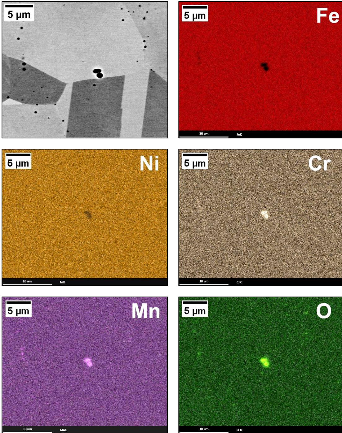
Figure 9. EDS scans of the UK-NAMRC PM-HIP 316H showing relative concentrations of elements. The upper-left backscatter electron image shows the microstructure of the EDS scanned area.
