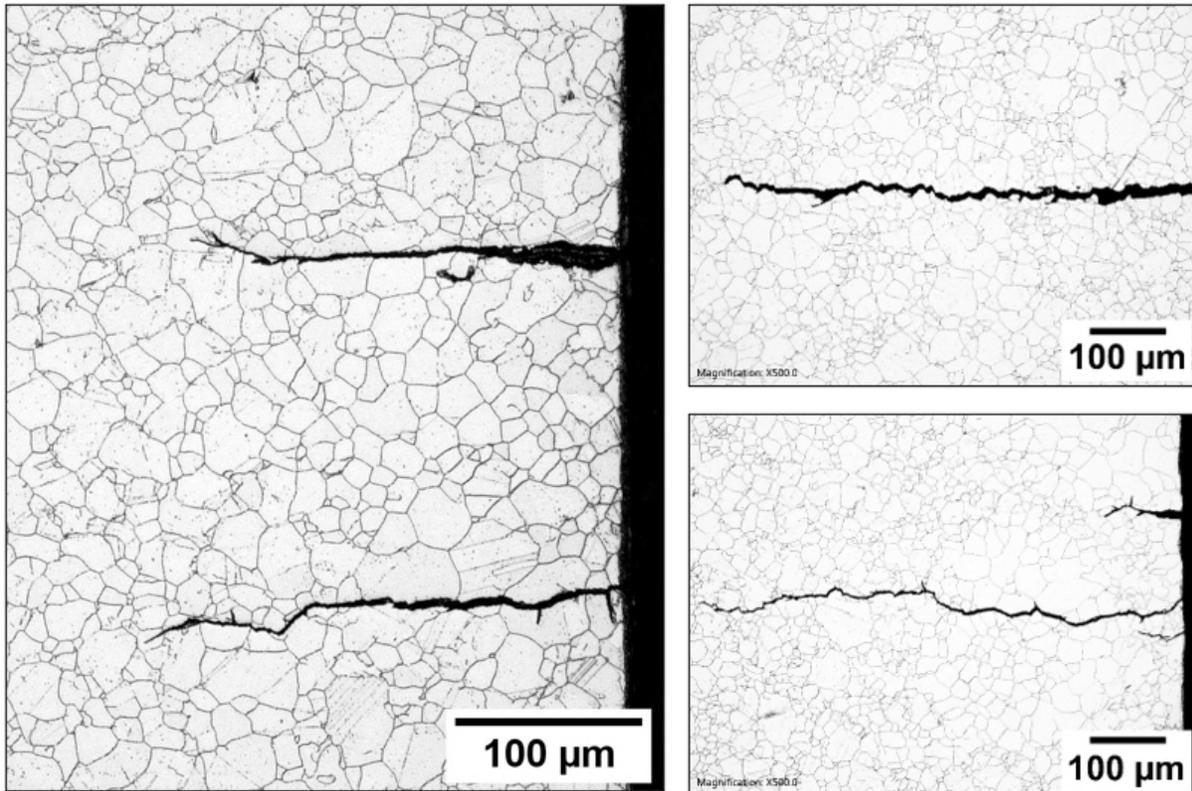
Figure 10. Optical micrographs from of the UK-NAMRC 316H stainless steel after LCF testing. Cracking appears to propagate entirely through the grain interiors (transgranular).
