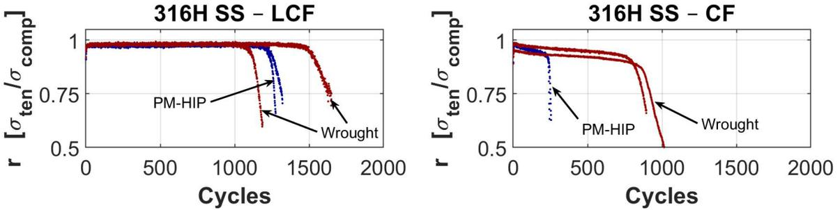
Figure 5. Ratios of maximum tension and maximum compression stress for LCF (left) and CF results (right) for the UK-NAMRC 316H results shown in Figure 4 and with comparison to a wrought 316H stainless steel.
