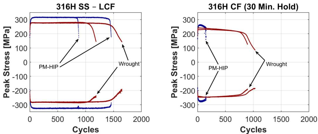
Figure 1. Peak stress versus cycles to failure for 316H stainless steel tested at 650°C with a fully reversed, total strain of 1%. Data extracted from Rupp [3].
