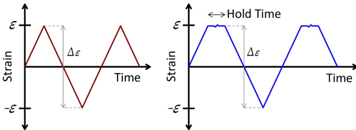
Figure 2. Schematics showing strain-controlled LCF (left) and CF (right) testing procedures.
