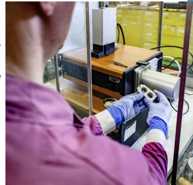
Laser Flash Analyzer for Measuring Thermal Diffusivity of Molten Salts
