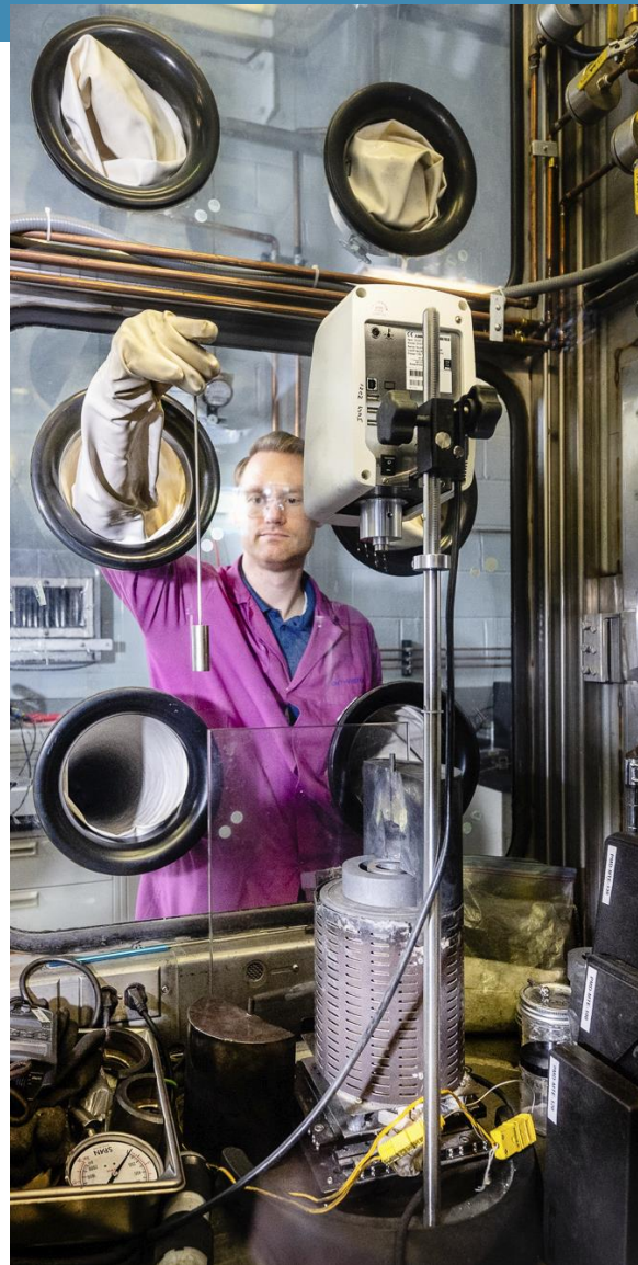
Rotational Viscometer Installed in a Glovebox for Measuring Molten Salt Viscosity
