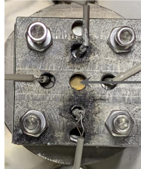
Gold-coated \text{Be}_2\text{C} mounted on stage for carbon ion irradiation
