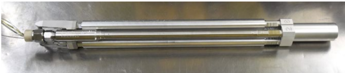
Molten Salt Research Temperature-Controlled Irradiation (MRTI) designed for instrumentation, not installed
