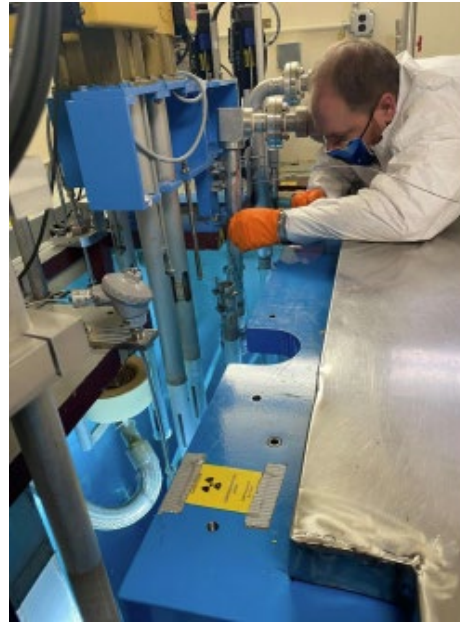
Neutron flux sensor installation in NRAD (left) and testing outside NRAD in transfer tunnel (right)
