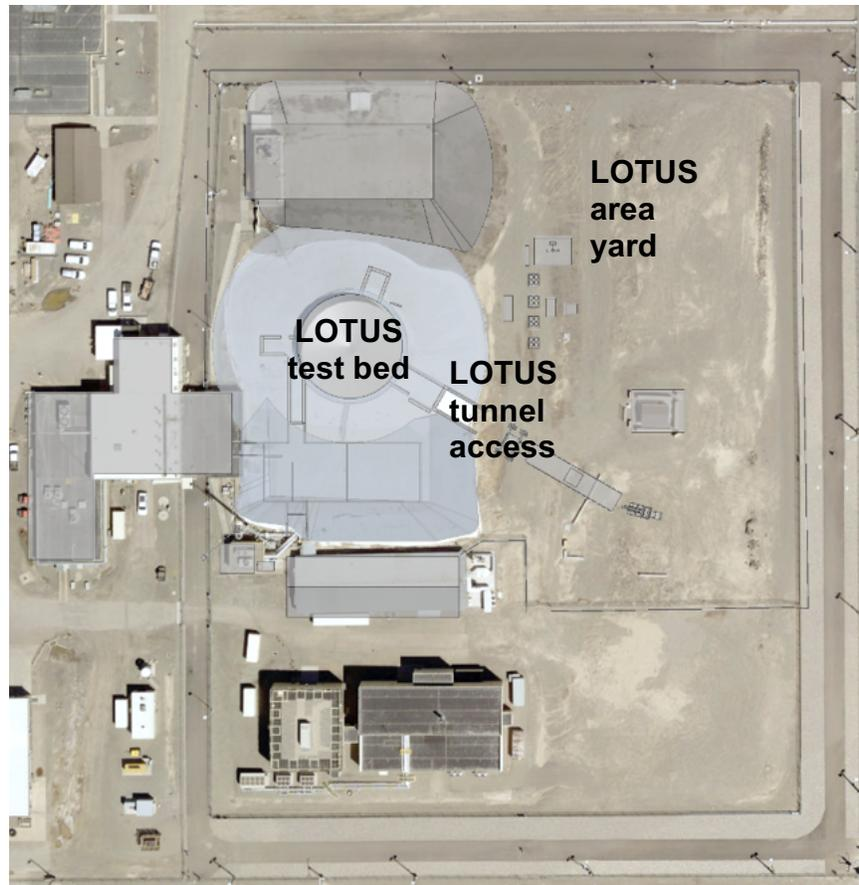
Figure 2. Aerial View of the ZPPR Area Overlaid With the Conceptual LOTUS Facility Layout Showing the Cell, Proposed Tunnel Access, Support Areas, and Yard Area.
