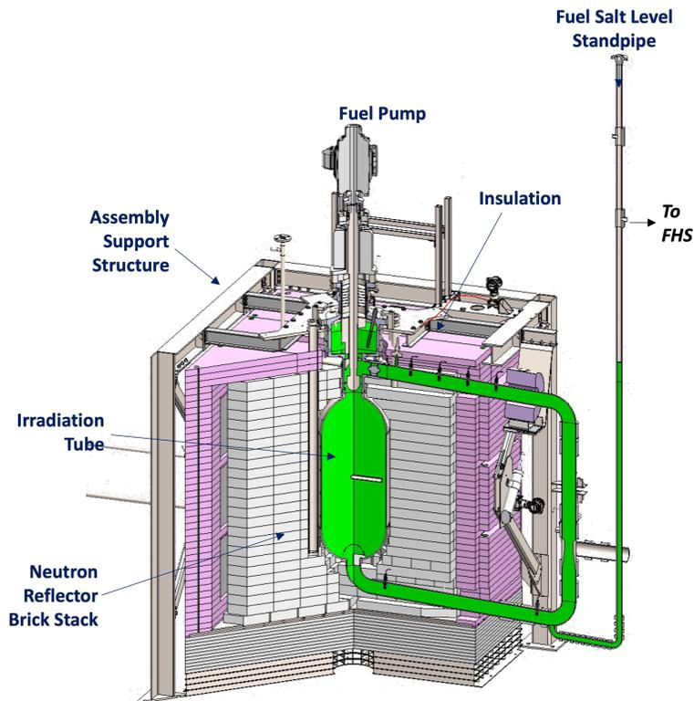
Figure 7. CAD Model Showing the Fuel System Core Surrounded by Reflector Bricks, Insulation, and the Structural Steel Frame [4].
