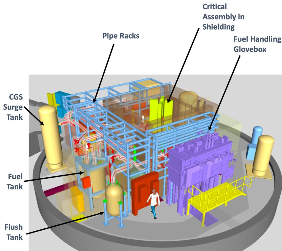
Figure 4. NavisWorks® Freedom Model Showing Some MCRE Subsystems [1].
