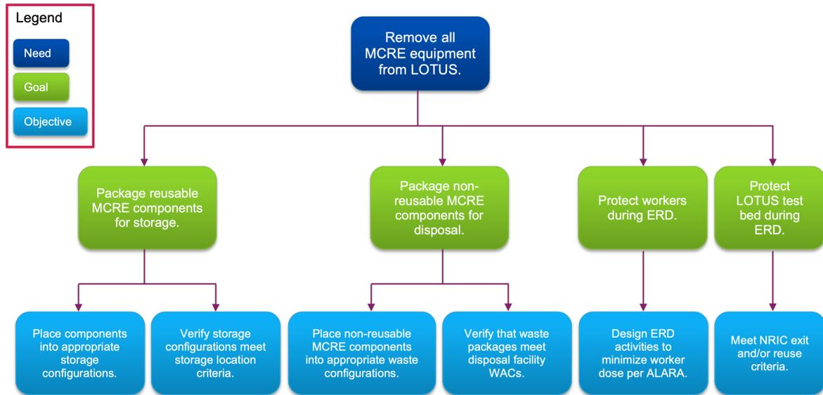
Figure 5. Needs, Goals, and Objectives for the MCRE ERD Operational Sequence.
