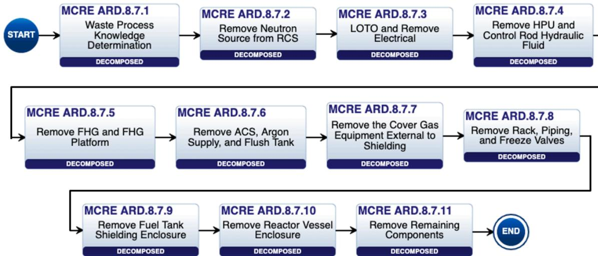
Figure 6. Diagram Showing the Decomposition for MCRE ERD. ERD begins after all fuel salt and contaminated flush salt have been removed from the system.
