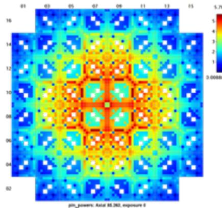
Figure 1: Radial 2D pin powers BWR mini-core.
