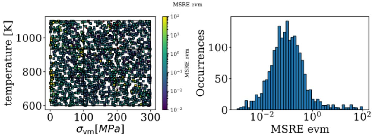
Figure 1: Validation results of 2,000 surrogate model simulations compared to physics-based simulations in terms of the mean squared relative error ( MSRE ) on the computed accumulated strain ("evm"). The training set, corresponding to this model, consists of 16,000 training and 2,000 testing simulations.
