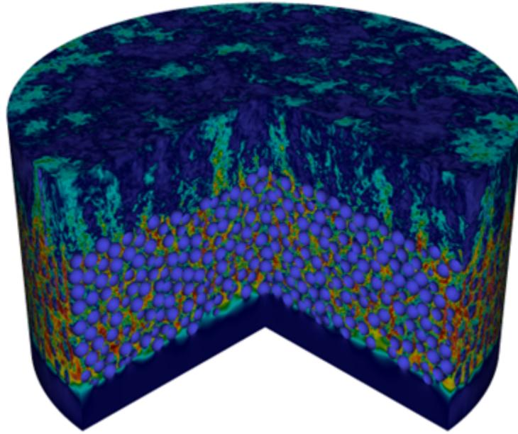
Figure 1: Instantaneous velocity field generated from LES of a bed of 7,000 pebbles.
