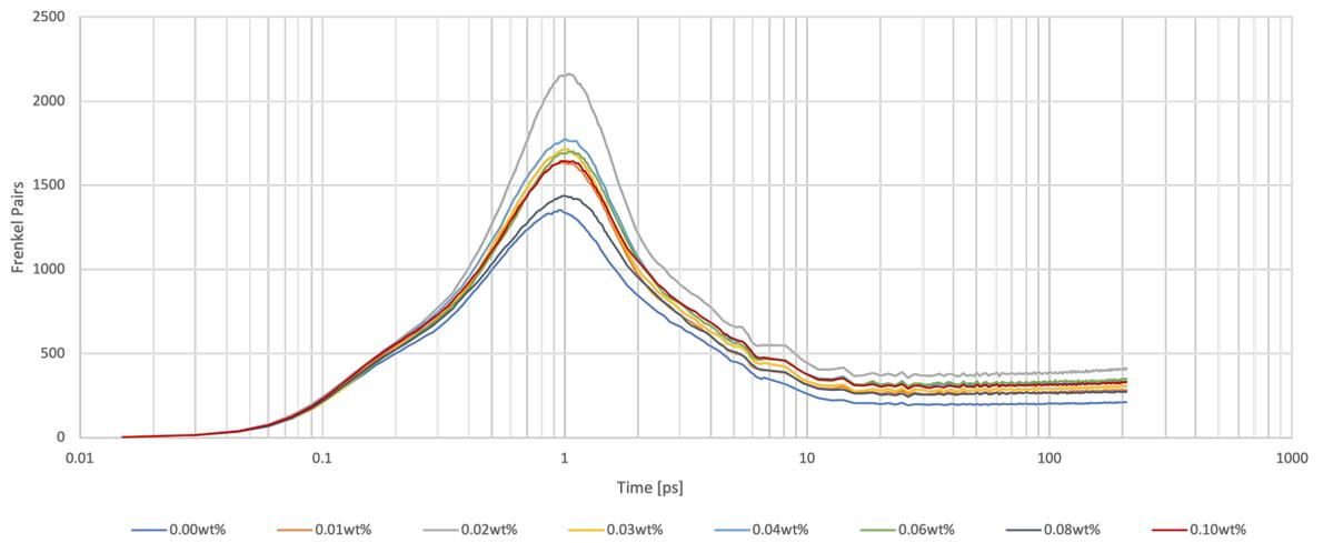
Figure 2: Number of Frenkel pairs making up the average 15 keV collision cascade as a function of time for a Fe/Cr/C alloy modeling SS-316 with a varying carbon content. Each profile is the average of 20 cascade simulations.
