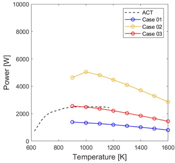
Figure 1: Capillary limit for Cases 01, 02, and 03 with different liquid gap sizes.
