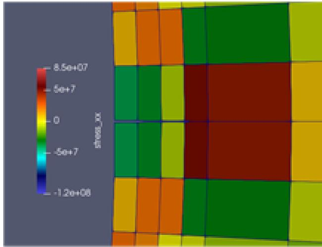
Figure 1: UN TRISO IPyC crack failure mode.
