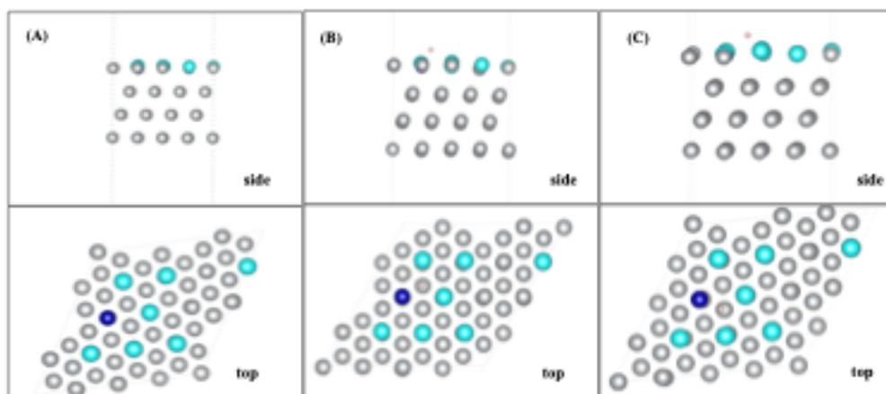
Figure 1: Density functional theory optimized structures (A) alloy structure, (B) H adsorbed at the face-centered cubic site, and (C) H adsorbed at the hexagonal close-packed site. Color codes are Ni: grey, Pt: Cyan, Co: Blue, and H: Pink.
