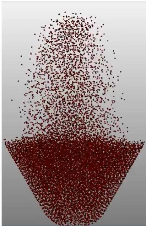
Figure 1: Image of spouted bed simulated in MFiX.
