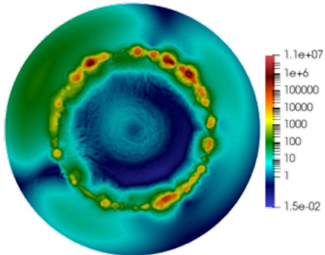
Figure 2: Radial slice of the power deposition [W/m<sup>3</sup>] for an axisymmetric electron density profile.
