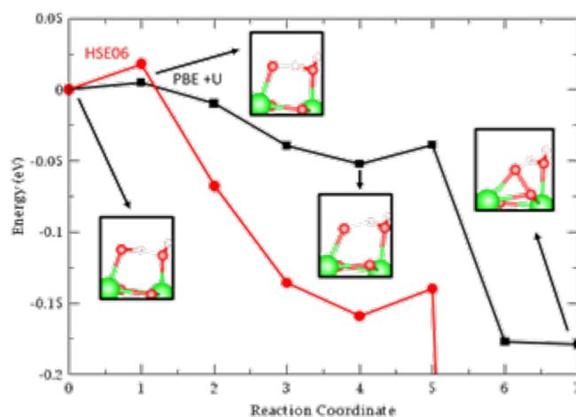
Figure 1: Calculated reaction barrier for the reaction of a hydroxyl radical with a localized hole on a lattice oxygen on the ZrO<sub>2</sub> surface. PBE +U and HSE06 results are shown in black and red, respectively. Insets show the local atomic structure at various points along the reaction path, with Zr atoms in green, oxygen atoms in red, and hydrogen atoms in pink.
