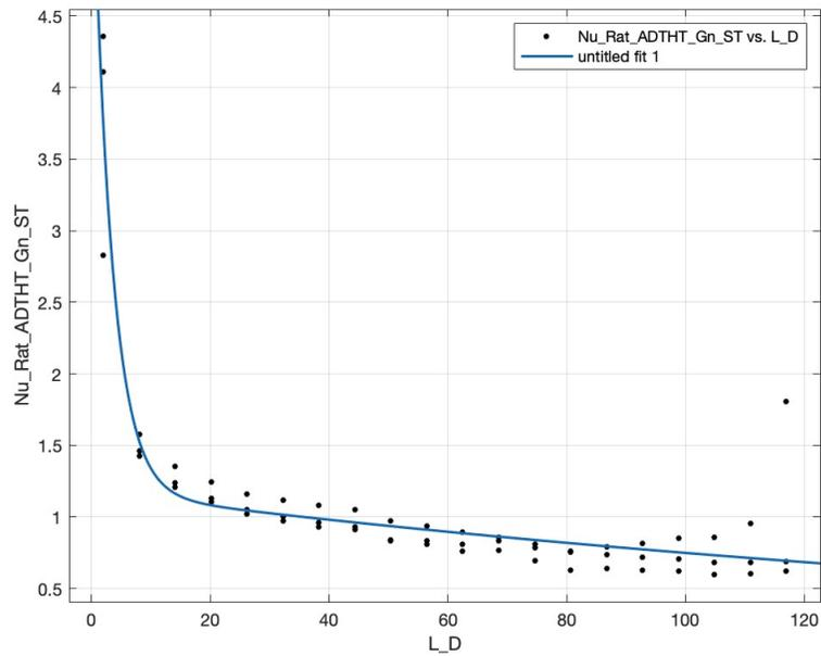
Figure 2: The ratio of experimental Nu vs. predicted Nu vs. axial position for acceleration-induced deteriorated heat transfer.
