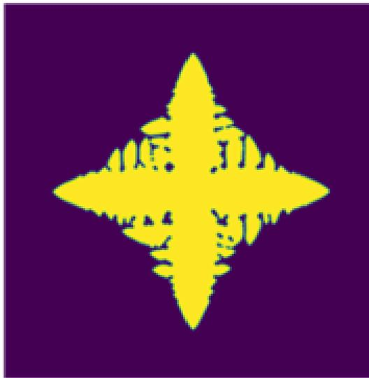
Figure 3: The true Fe-C dendrite for a given cooling temperature and initial carbon concentration at a given timestep.
