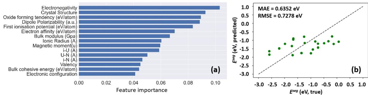
Figure 3: ML results: (a) feature importance analysis (i: solute) and (b) predicted segregation energy ( $E_{seg}$ ) vs. computational  $E_{seg}$  from the optimized kernel ridge regression model.
