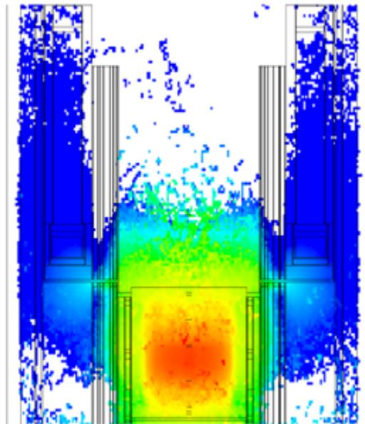
Figure 1: Optimized neutron flux to estimate intermediate heat exchangers sodium activation.
