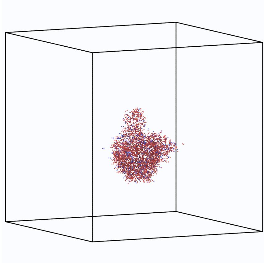
Figure 1: Distribution of interstitials in a Fe/Cr/C alloy modeling SS-316 at the peak of a 15 keV collision cascade.
