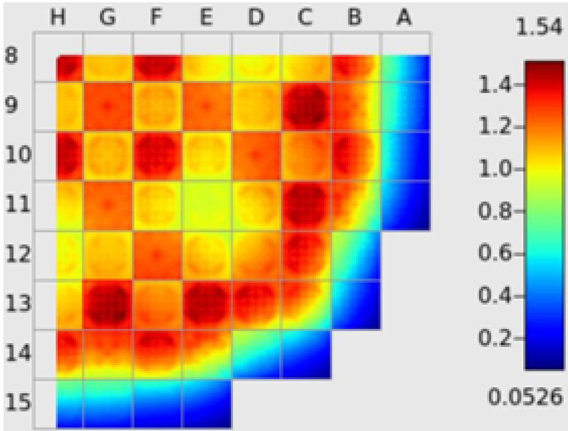
Figure 1: Radial rod-wise power distribution at the burnup where maximum Fdelta H occurs.
