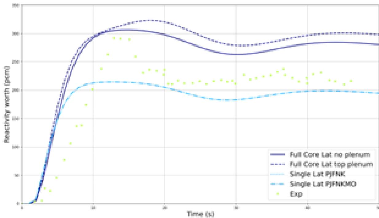
Figure 1: Pump startup simulation results compared to experimental data.
