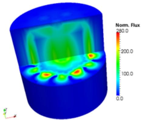
Figure 1: Thermal flux distribution at time of maximum power (2.12 seconds) during an inadvertent drum rotation accident.
