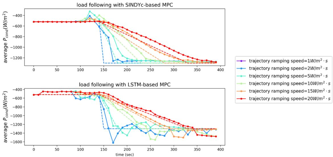
Figure 4: Load following with SINDYc- and LSTM-based MPCs, with different magnitudes of final setpoints.
