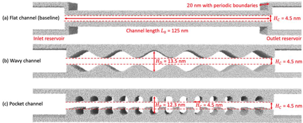
Figure 1: Visualization of the three channel geometries: (a) flat channel, (b) wavy channel, and (c) pocket channel.
