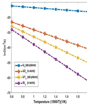
Figure 3: Diffusion coefficients as a function of temperature.
