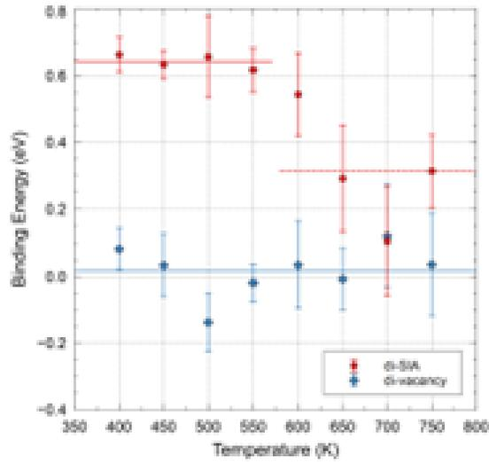
Figure 2: Binding energies for a di-SIA and a di-vacancy in -uranium.
