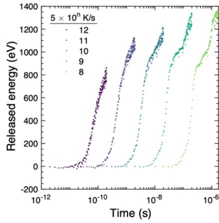
Figure 1: MD simulations determine the energy release associated with radiation damage annealing at different heating rates (K/s).
