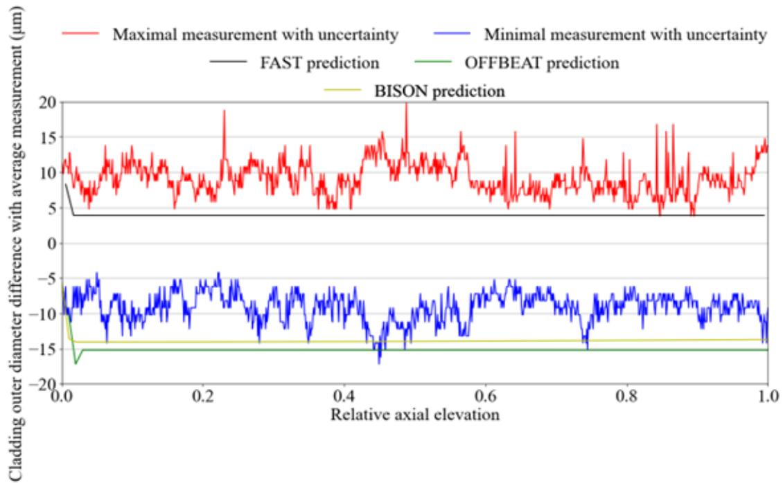
Figure 1: Cladding outer diameter comparison of measured and predicted values.
