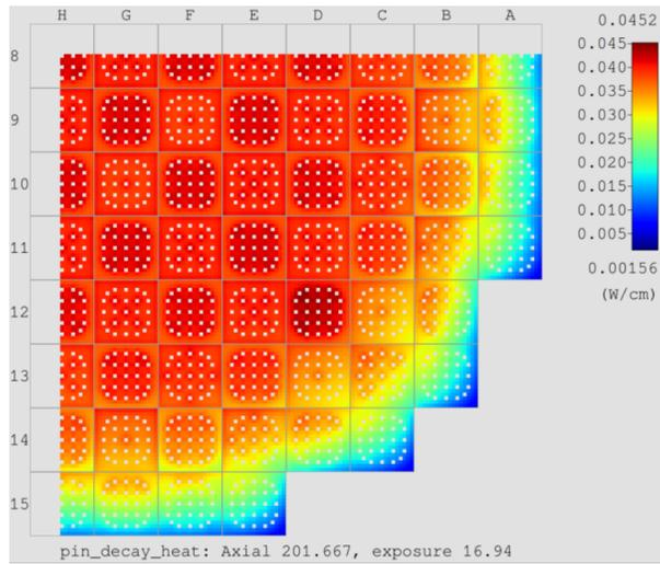
Figure 2: Radial and axial decay heat distribution after 1 year of cooling—Watts Bar Unit 1 Cycle 1.
