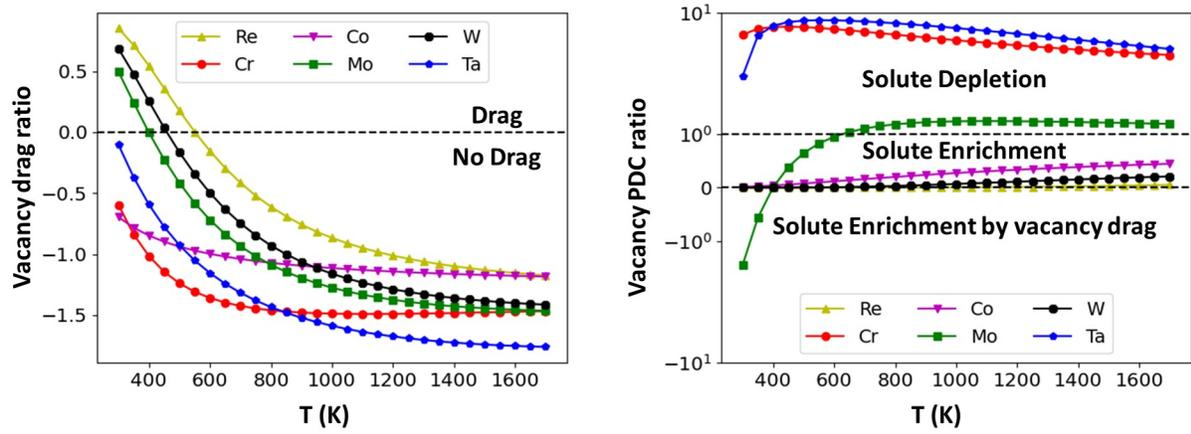
Figure 1: Vacancy drag ratios and partial diffusion coefficient ratios for solute atoms in FCC nickel.
