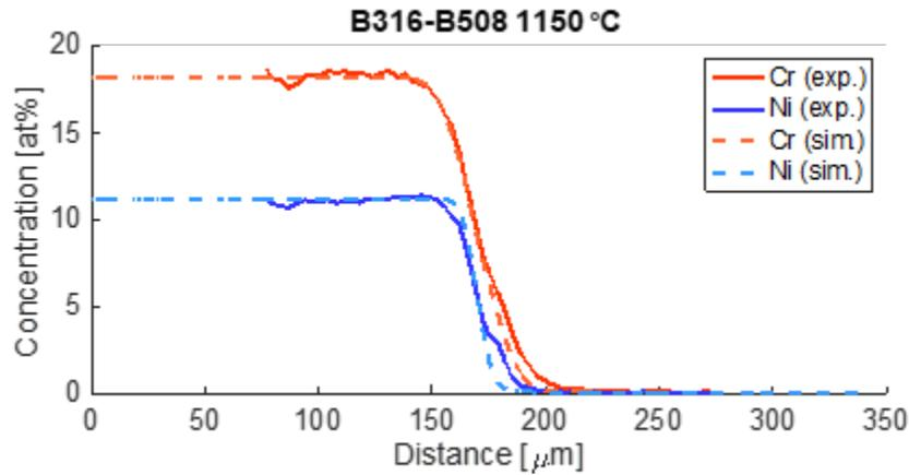
Figure 2: Concentration profiles EPMA (exp.) and phase-field simulation (sim.) of a 316L-A508 1150°C temperature cycle diffusion couple.
