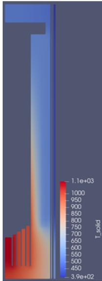
Figure 1: Steady-state solid temperature distribution of reflectors predicted by SAM.
