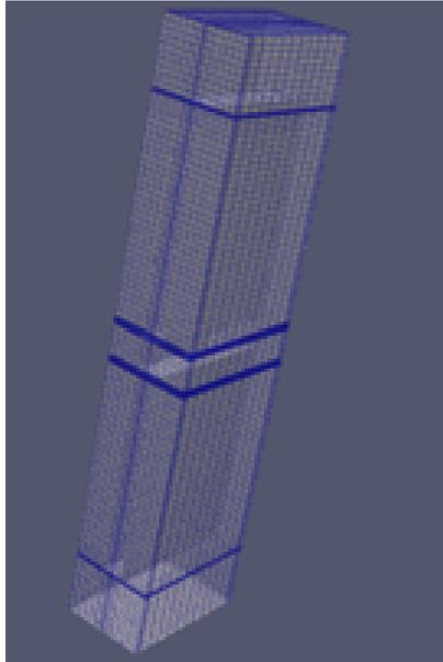
Figure 1: Mesh for NBSR fuel element.
