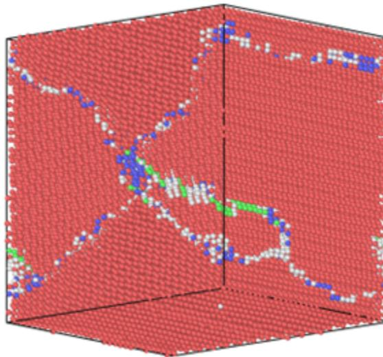
Figure 2: Partially transformed cell in the transition from BCC (blue atoms) to HCP (red atoms). White or green coloring reflects twin or misaligned HCP crystallites as derived from common neighbor analysis in Ovito.
