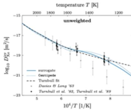
Figure 2: Estimated model predictions for the xenon diffusivity under irradiation conditions compared to the experimental data from Turnbull.
