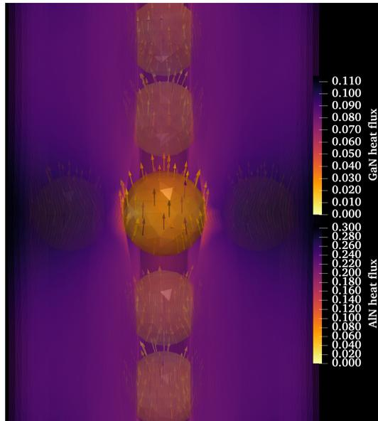
Figure 3: Heat flux streamlines in cruciform geometry of GaN defects in AlN bulk.
