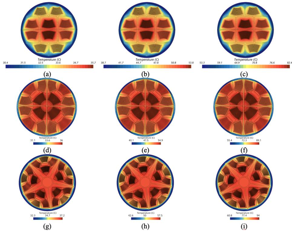
Figure 2: The steady-state temperature for (a) 6 watt, (b) 18 watt, and (c) 42 watt fuel elements in an 18 inch sealed base canister configuration; (d) 6 watt, (e) 18 watt, and (f) 42 watt fuel elements in an 18 inch sealed densely packed canister configuration; and (g) 6 watt, (h) 18 watt, and (i) 42 watt fuel elements in a 24 inch sealed densely packed canister configuration.
