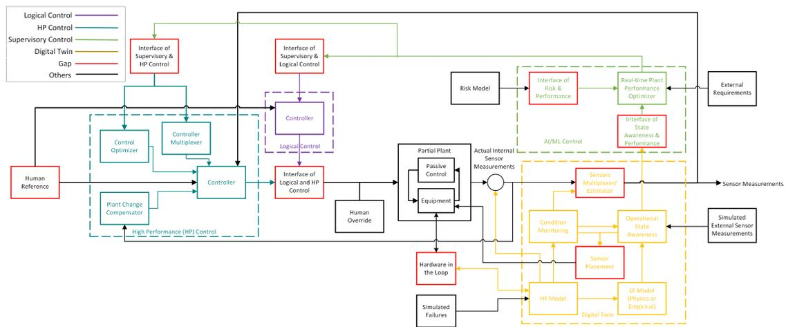
Figure 2: Design approach to integrate advanced control methods and digital twins for advanced nuclear reactors.
