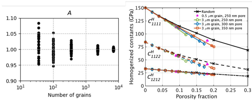
Figure 2: Effective elastic constants of U-10Mo, showing a convergence study for unirradiated fuel with different number of grains (left) and irradiated fuel with triple junction porosity of different pore sizes (right).
