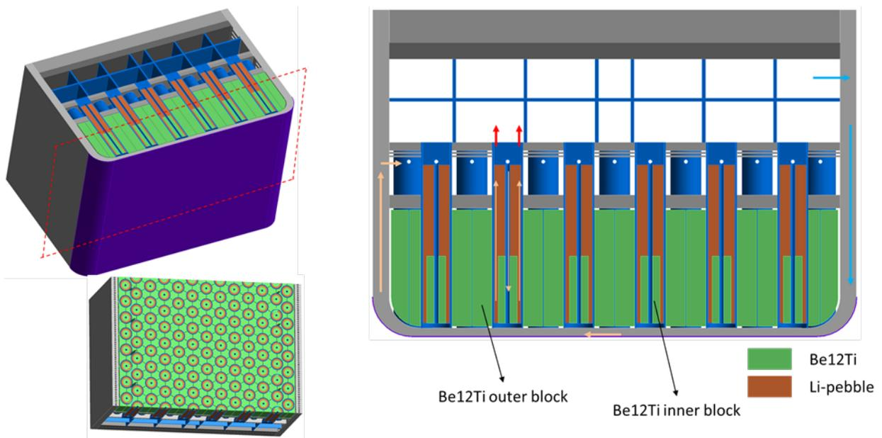
Figure 1: Flow path of the 2022 EU DEMO HCPB.
