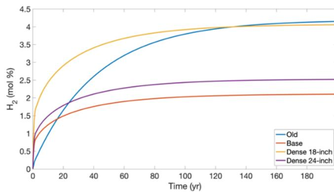
Figure 3: The hydrogen gas generation of the three packing configurations here against the old model data.
