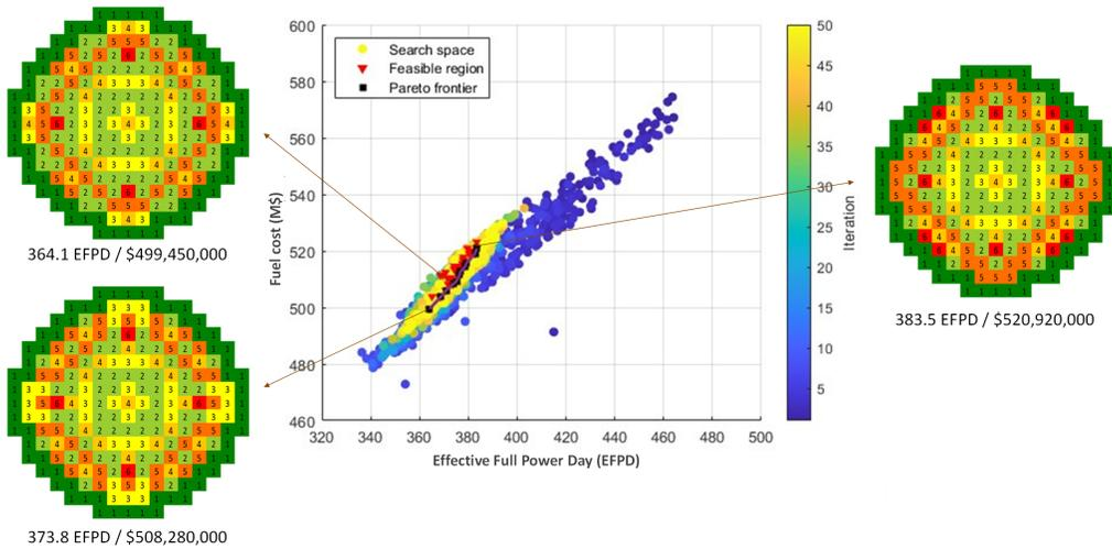
Figure 1: Search space, feasible region, and optimized solutions on the Pareto frontier of fuel loading patterns. Users can select one fuel loading pattern among the ones in the Pareto frontier.
