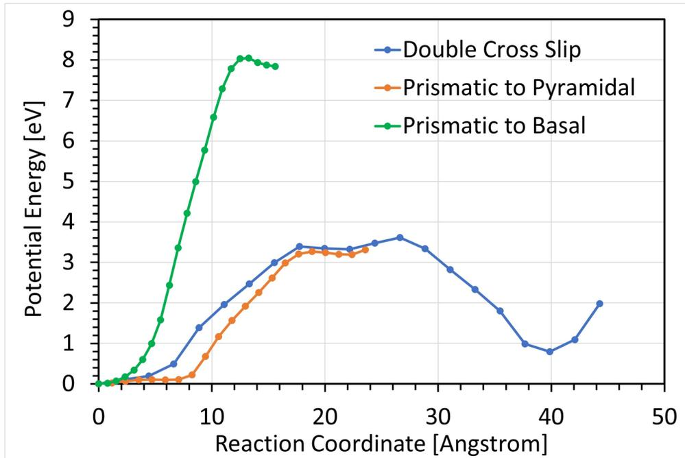
Figure 1: Preliminary plot of various cross-slip reaction path energies.
