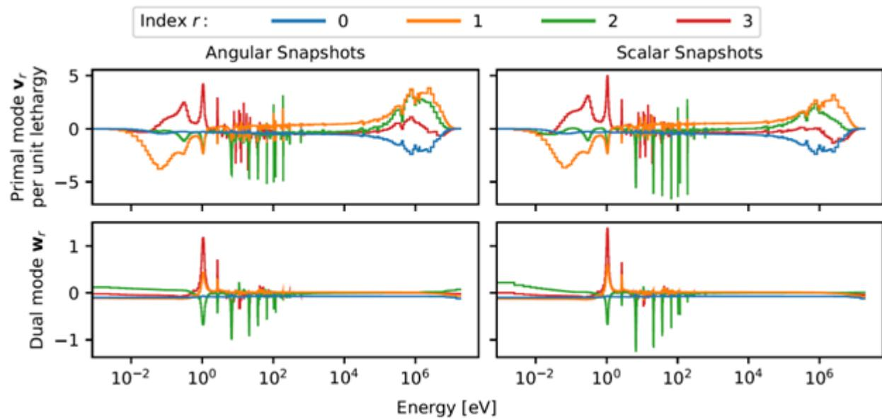
Figure 1: Balanced energy modes computed from light-water reactor pin-cell reference solutions.
