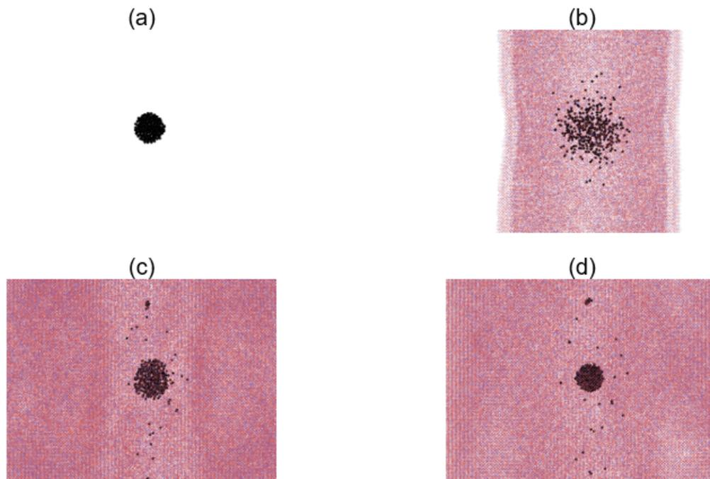
Figure 1: Snapshots of a thermal spike (3.5 MeV) simulation at (a) 0, (b) 1.5, (c) 44.5, and (d) 114.5 ps. Xe atoms are shown in black along with U (red) and Mo (blue) point defects.
