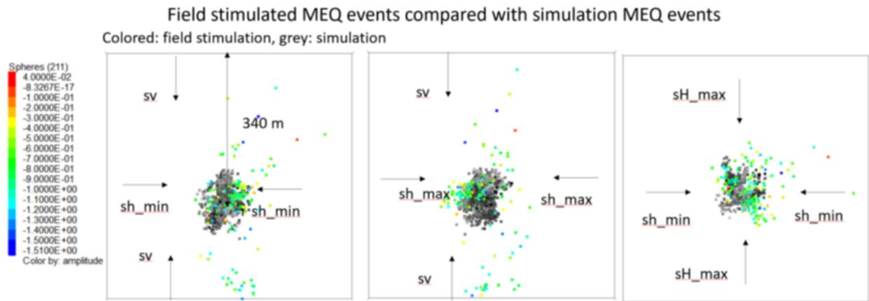
Figure 1: Comparison of the field-detected microseismicity cloud with simulation results for Stage 1. Field detected maximum magnitude is 0.04, and simulation maximum magnitude is 0.03.
