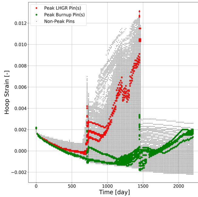
Figure 1: Example of parameters of interest (cladding hoop strain and rod plenum pressure) in full-core fuel performance modeling of a high-burnup PWR core.
