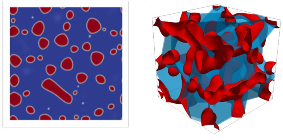
Figure 1: Evolved Xe gas porosity distribution in U-10Mo, showing predominant pores at triple junction points in 2D (left) and interconnected pores along triple junction lines in 3D (right).
