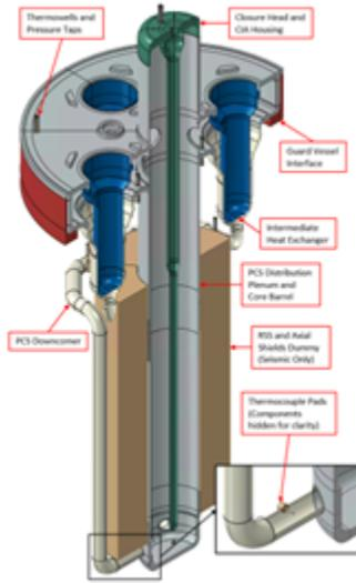
Figure 1: ABAQUS parts for the MARVEL primary boundary.
