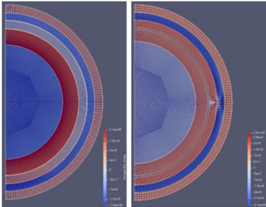
Figure 2: (left) 2D TRISO particle with IPyC layer debonding from SiC and (right) 2D TRISO particle model with crack in IPyC layer subjecting SiC to tensile stresses.
