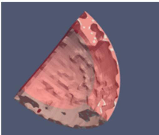
Figure 3: Delamination fracture mode.
