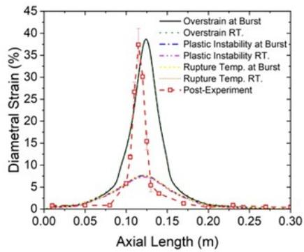
Figure 3: BISON-calculated and measured strain profiles for Zircaloy-2.
