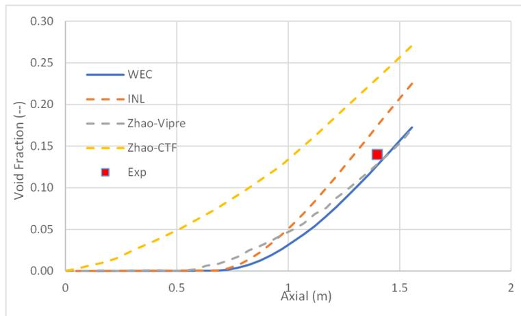
Figure 3: VERA simulation benchmark with PSBT test data.
