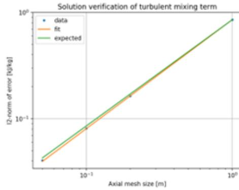
Figure 2: Solution verification of ANTS turbulent mixing term.
