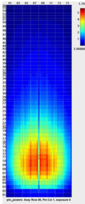
Figure 2: Axial pin powers BWR mini-core.
