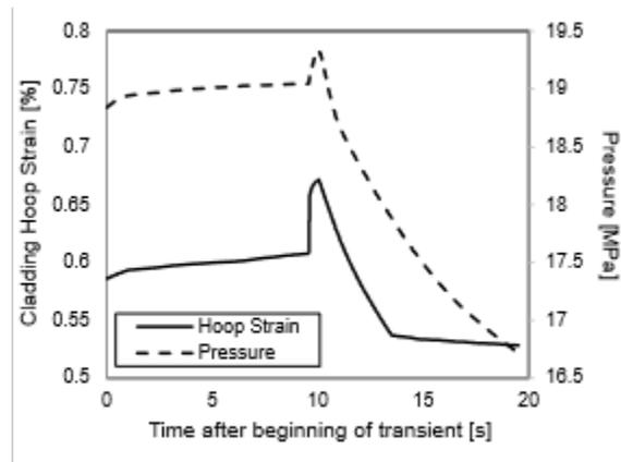
Figure 2: Cladding hoop strain and pressure for the IFBA core peak burnup rod during a control rod ejection accident.
