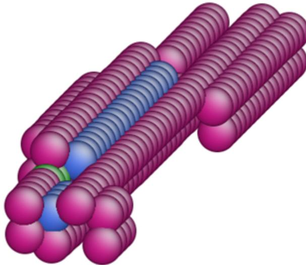
Figure 2: Atomic configuration of the double cross-slip transition. The miscoordinated atoms are shown, and the center of the dislocation line has rotated to rest on an inclined slip plane.
