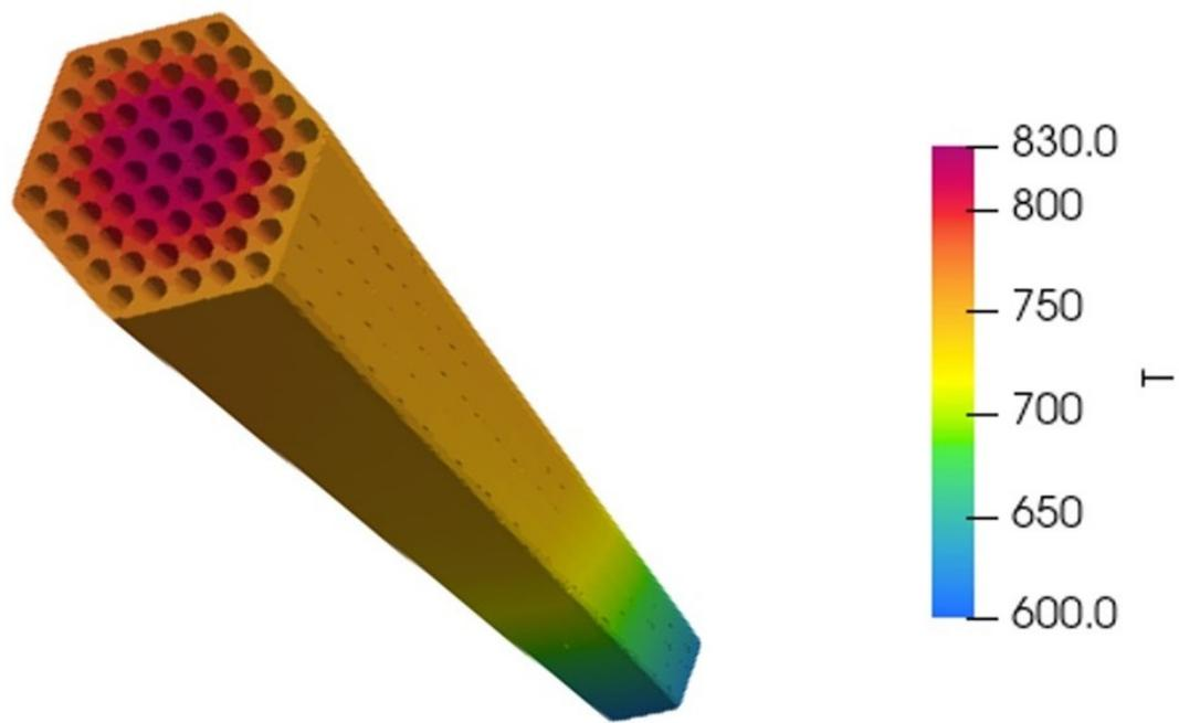
Figure 1: Temperature in an EBR-II assembly predicted by Pronghorn-SC.
