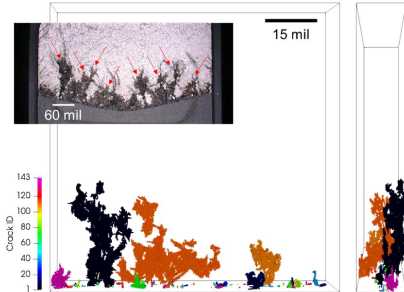
Figure 2: (Top left) Light optical image of SCC fingers in specimen MG5-027 (Heat D2739) developed in a 12.2% cold worked 304 stainless-steel specimen loaded in the LT orientation. Red arrows indicate the fingers. (Bottom) A simulated SCC crack that resembles SCC fingers after 15% cold rolling visualized from the top-down (left) and side views (right) colored by individual crack identification number. The bounding boxes indicate the microstructural volume.
