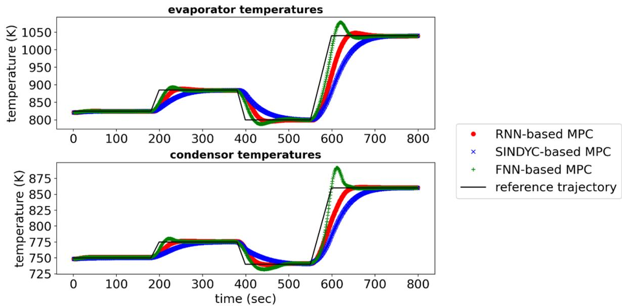
Figure 2: Performance of the FNN-, LSTM-, and SINDYc-based MPCs in tracking the reference temperature setpoints of the central HP evaporator and condenser.
