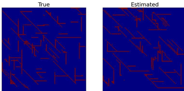
Figure 2: Estimation of heterogeneous permeability of the granitoid layer, where the true permeability field is shown on the left and the estimation result is shown on the right. The red lines represent fractures with a permeability of  $1e-14 \text{ m}^2$ , and the permeability of the blue area is  $1e-16 \text{ m}^2$ .
