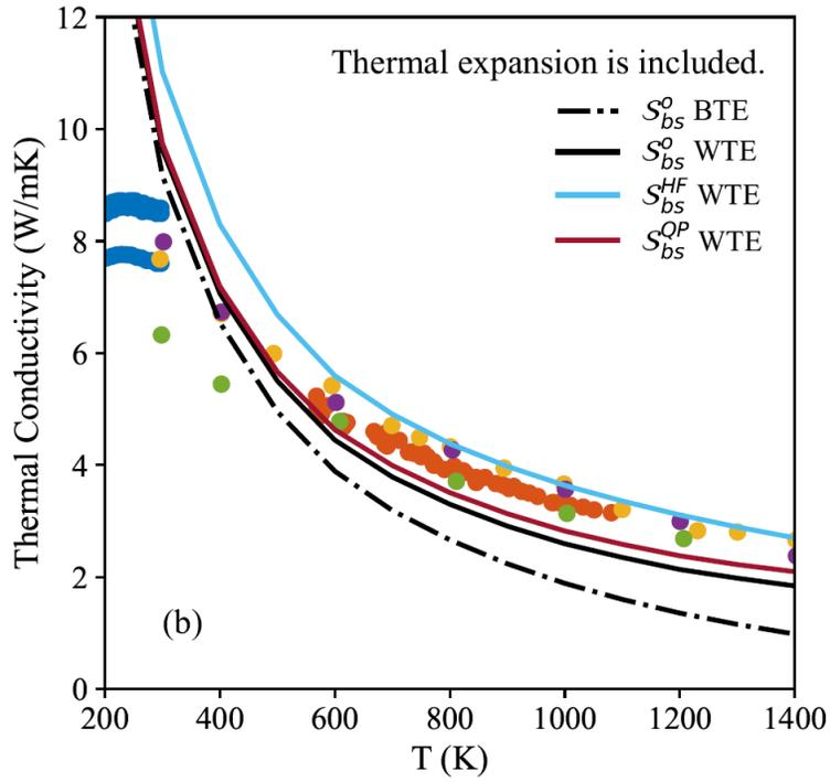
Figure 2: Thermal conductivity computed using GGA + U + SOC ( $U = 4$  eV) and comparing with experiments. Thermal expansion is included. The self-consistent perturbation theory is applied.
