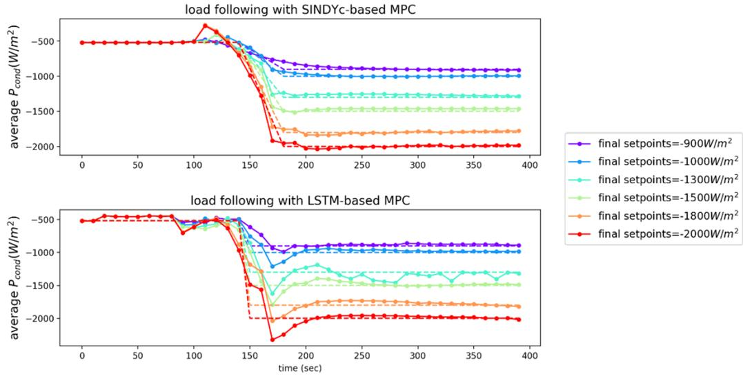
Figure 3: Comparison between the SINDYc- and LSTM-based MPCs in regard to tracking reference trajectories with different final setpoints and ramping speeds. Load following with SINDYc- and LSTM-based MPCs, with different magnitudes of final setpoints.
