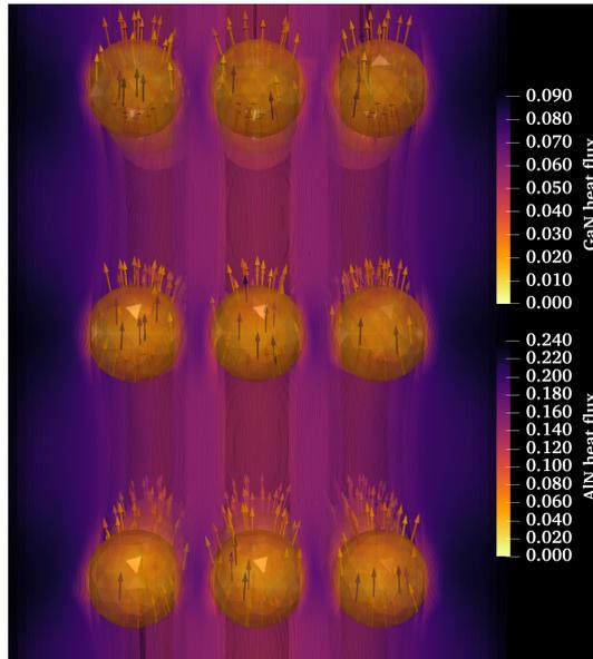
Figure 1: Heat flux streamlines in barricade geometry of GaN defects in AlN bulk, 15 axial layers.
