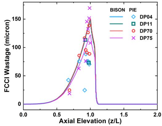
Figure 1: BISON-predicted fuel-cladding chemical interface wastage thickness compared with measured data for four representative U-10Zr/HT9 pins irradiated in X447/A.
