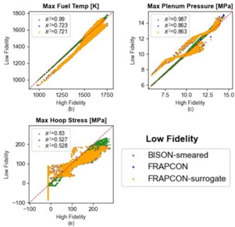
Figure 1: Comparison of BISON to FRAPCON on full-core PWR scale.
