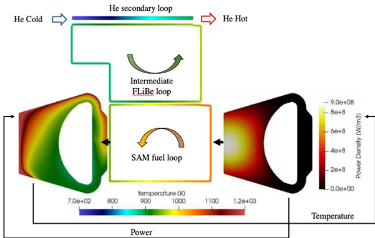
Figure 1: Steady-state results of coupled SAM-Pronghorn-Griffin of an MSR.
