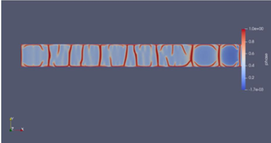
Figure 1: Crack pattern obtained for a tensile on a SFCT beam.
