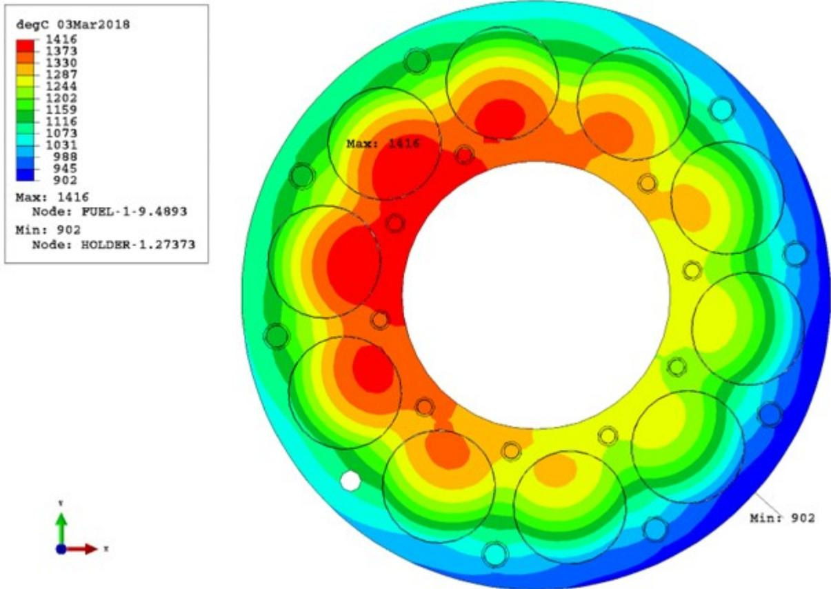
Figure 3: Cross-section temperature ( $^{\circ}\text{C}$ ) of The offset gap in NW for Capsule 1 of the AGR-5/6/7 experiment.
