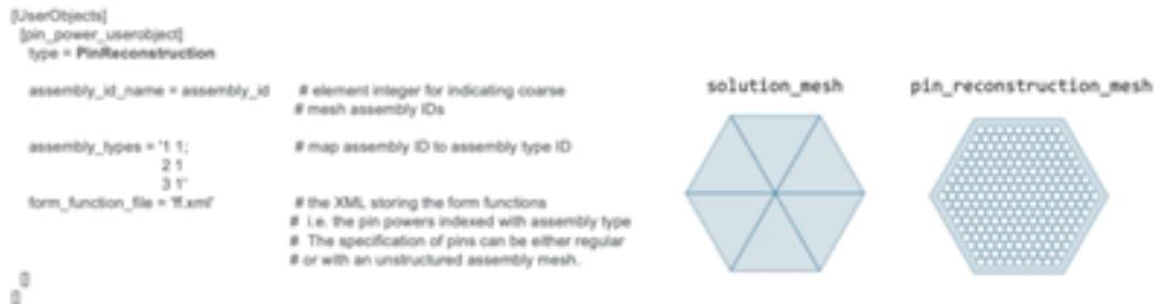
Figure 1: Pin power reconstruction implementation in Griffin reactor physics code.
