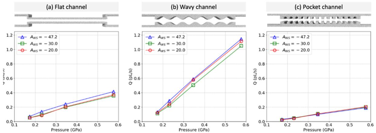
Figure 2: Measured channel outlet volumetric flow rate (picoliter per second) versus inlet pressure: (a) flat channel, (b) wavy channel, and (c) pocket channel. Plotted separately are relatively wetting (triangles), neutral (squares), and relatively non-wetting (circles) silica surface for water.
