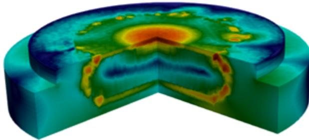
Figure 1: Power deposition [W/m<sup>3</sup>] for an axisymmetric electron density profile.
