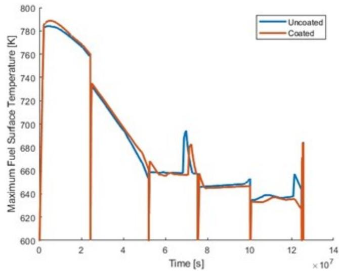
Figure 1: Maximum fuel surface temperature with and without a 30 m chromium coating during commercial irradiation of Halden IFA-650 Rod 10. Oxide growth on uncoated cladding increases thermal resistance from fuel to coolant, leading to higher temperatures at end of life.
