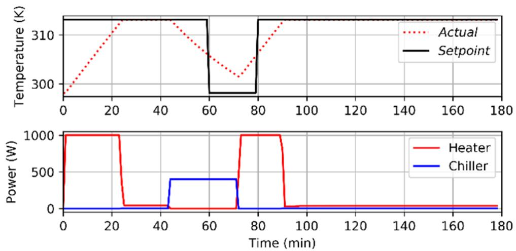
Figure 1: RELAP5-3D MPC with an integer solver and 25 minute time horizon utilizing an absolute difference objective function.
