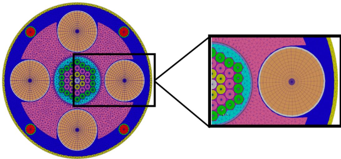
Figure 1: Radial view of the MARVEL core mid-plane.
