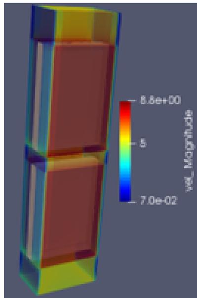
Figure 2: Velocity distribution in fuel element.
