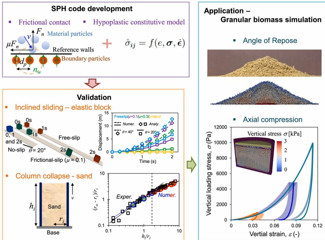
Figure 1: Schematic of the overall workflow. A frictional contact and a hypoplastic constitutive mode is implemented first, then the code is validated using two examples before using to model granular biomass flow through an angle of response and an axial compression test. The granular biomass flow simulation matches the experimental results conducted.
