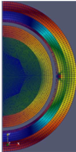
Figure 2: UN TRISO failure mode stress analysis.
