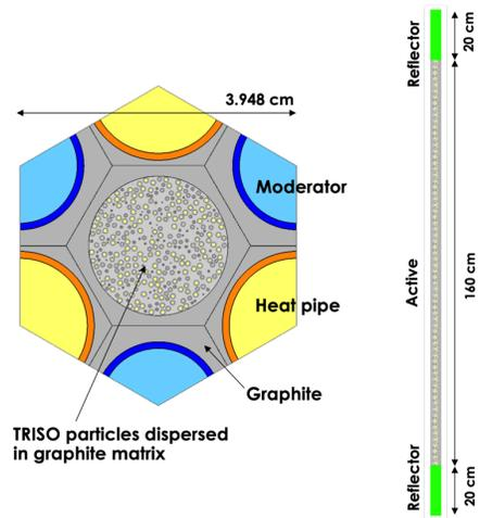
Figure 2: Heat-pipe reactor unit cell.
