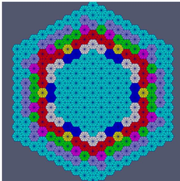
Figure 2: HTGR core design.
