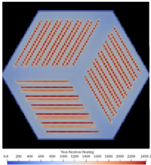
Figure 2: OpenMC gamma-induced energy deposition in the FHR core (arbitrary units), showing the relatively large graphite fraction in the FHR core as well as the complex distribution of gamma energy deposition.
