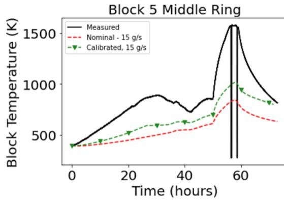
Figure 1: Comparison of RELAP5-3D (nominal and calibrated) results compared to measured data for HTTF experiment PG-26.
