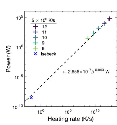
Figure 3: Simulated results are extrapolated to experimental heating rates, demonstrating an excellent match with prior experiments.
