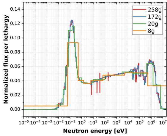
Figure 1: Normalized flux in Shift based on varied group macroscopic cross sections.
