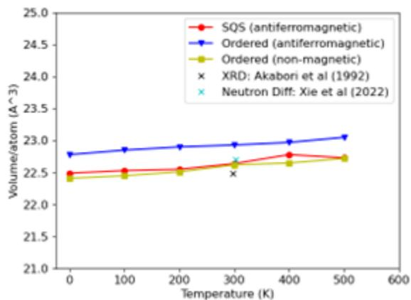
Figure 1: Volume per atom versus temperature using GGA.
