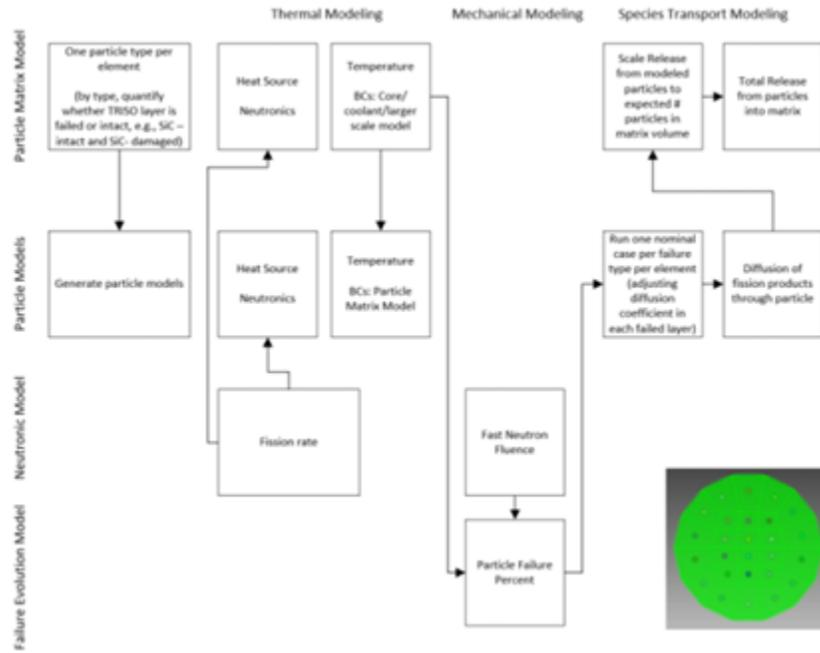
Figure 1: Diagram of the singular particle per element methodology.
