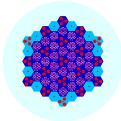
Figure 1: HTGR concept for reactor physics modeling and performance studies.
