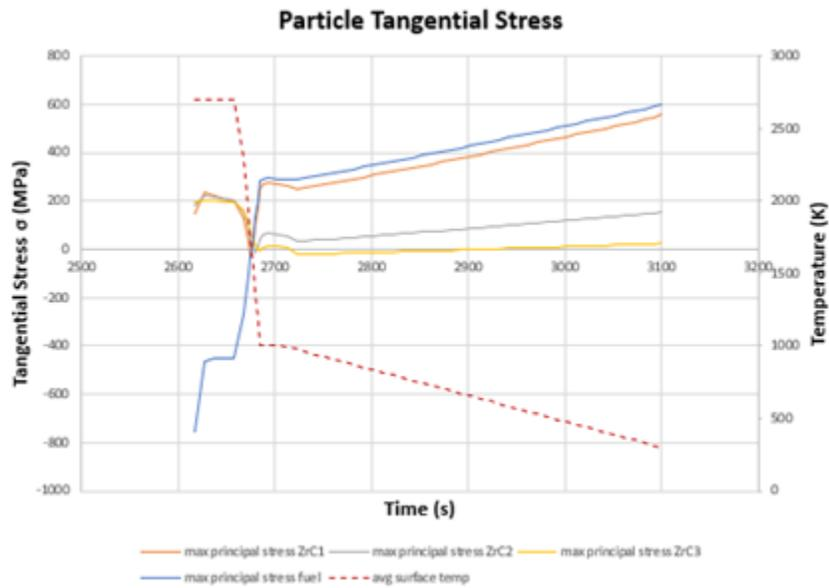
Figure 2: Operation thermal stress assessment on a multilayer Cer-Cer particle design.
