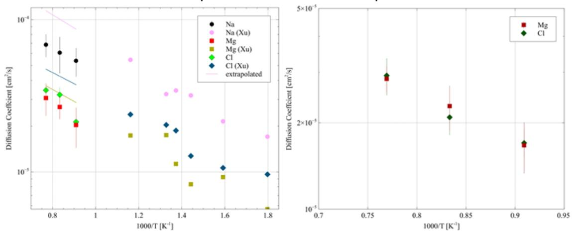
Figure 3: The self-diffusion coefficient for the eutectic NaCl-MgCl<sub>2</sub> and MgCl<sub>2</sub>. What we observed for the eutectic composition is that Na<sup>+</sup> ions diffuse the fastest and Mg<sup>2+</sup> ions the slowest with chlorine ions falling in the middle. This is the exact same behavior observed by the other AIMD study at lower temperatures.
