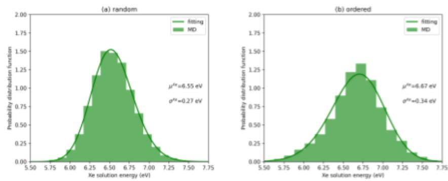
Figure 2: Distributions of Xe solution energies in the (a) random solid solution and (b) the SRO state at 300 K. There is a slight increase in the mean solution energy and a noticeable broadening of the distribution.
