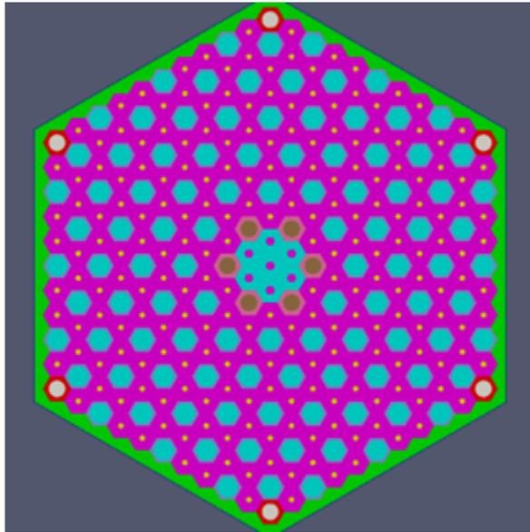
Figure 1: Standard fuel block.
