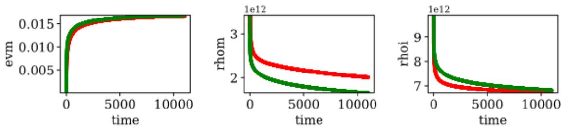
Figure 2: Example of a single output response at the same input parameter set from a physics-based simulation (red) and surrogate model (green) for the strain output ( evm ), the cell dislocation density ( rhom ), and the cell-wall dislocation density ( rhoi ).
