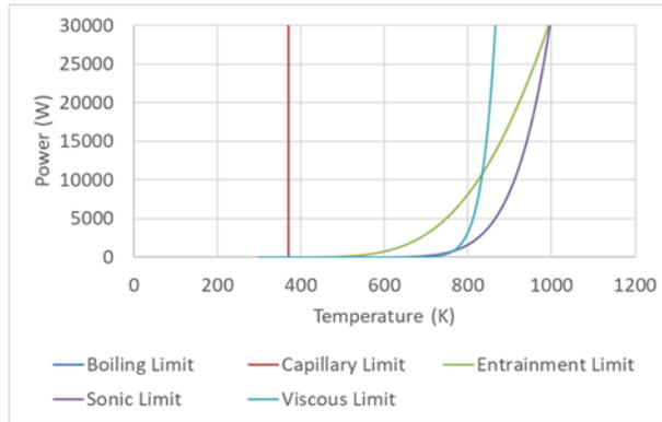
Figure 1: Operational limit of 6 ft heat pipe with mesh #100.
