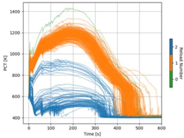
Figure 1: LBLOCA PCT versus time for 281 high-burnup rods (blue and orange lines) and the highest power rod in the core (green line).
