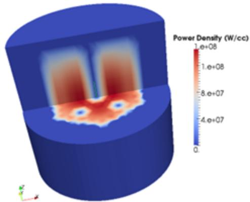
Figure 2: Power density distribution at time of maximum power (2.012 seconds) during an inadvertent drum rotation accident.
