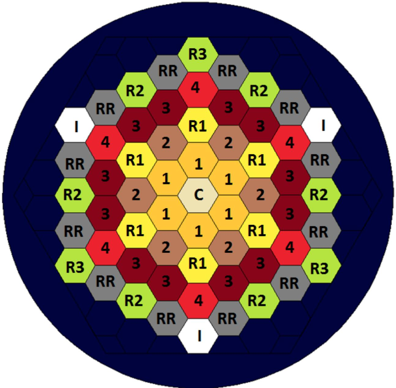
Figure 1: HTTR core layout with fuel (Columns 1-4), control rods (C, R1, R2, R3), replaceable reflectors (RR), and instrumentation (I).
