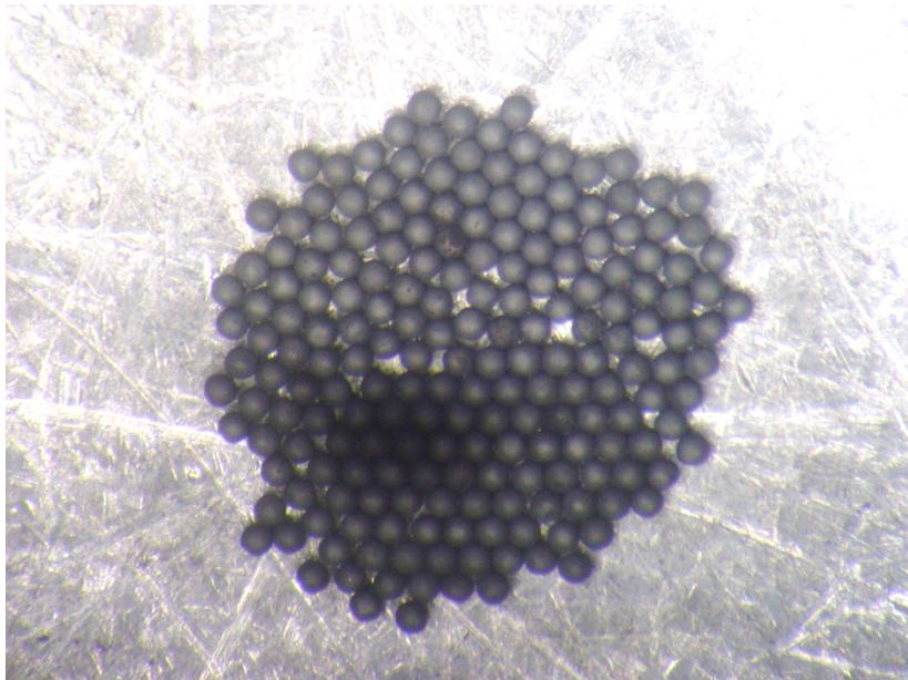
Figure 1: AGR-34 TRISO particles used to measure particle burnup from ATR irradiation.
