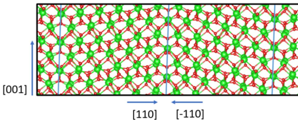
Figure 2: (110)/(-110) grain boundary model in monoclinic ZrO<sub>2</sub>. Locations of the grain boundaries are identified with blue vertical lines. The supercell used in the calculations has periodic boundary conditions. Crystal directions are shown next to the atomic structure. Zr atoms are in green, and oxygen atoms are in red.
