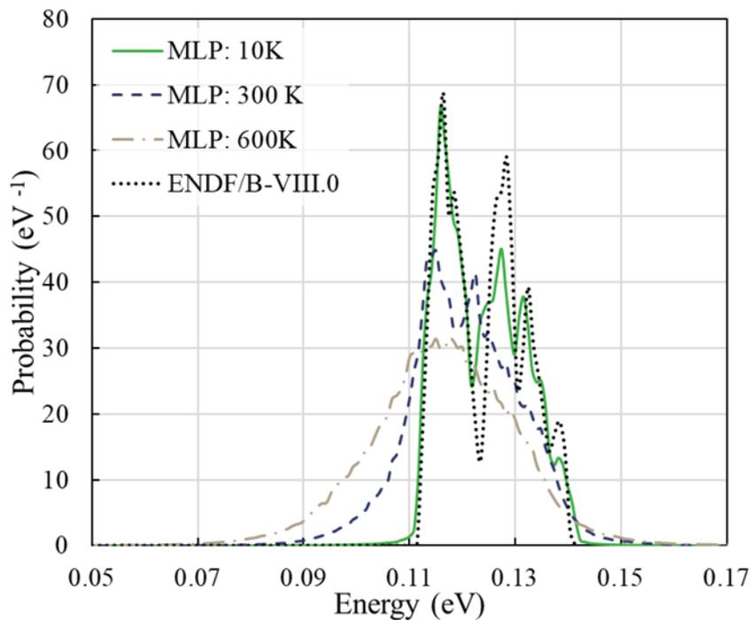
Figure 2: Phonon spectra of H(YH2) predict from molecular dynamics with a YH2 MLP compared to the ENDF/B-VIII.0 ab initio lattice dynamics spectrum. The 10 K MLP is in good agreement with ab initio, which neglects anharmonicity; however, the MLP captures anharmonic spectral shifts and broadening at higher temperatures.
