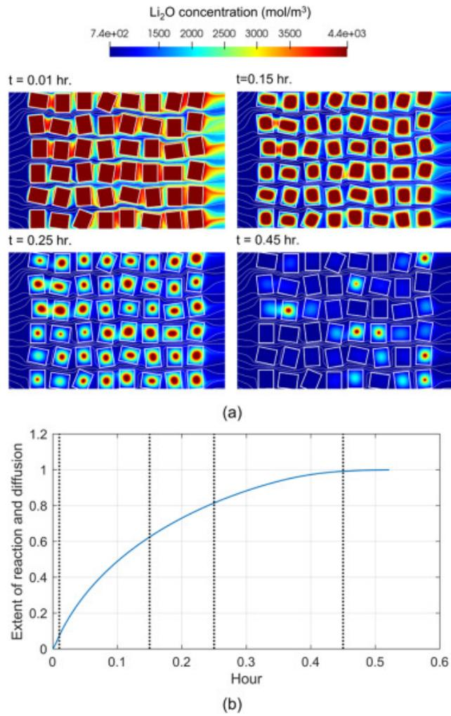
Figure 1: Oxide reduction process in the intermediate Peclet number ( $Pe=56$ ,  $W=24\text{mm}$ ): (a) concentration field of  $\text{Li}_2\text{O}$  at several time instants and (b) extent of reaction and diffusion.
