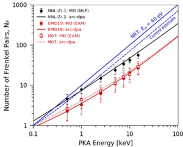
Figure 2: The surviving number of Frenkel pairs that survive post-cascade at  $T = 8$  K for the BMD19.3, M07 #3, and NNL-Zr.1 potentials. Markers indicate MD data averaged over 50 simulations (error bars represent standard deviation) while the solid lines are calculated with based on the arc-dpa damage efficiency curves fitted in Figure 1. The NRT-predicted number of defects ( $E_d = 40$  eV) and the arc-dpa model based on parameters estimated by experimental values are plotted for comparison.
