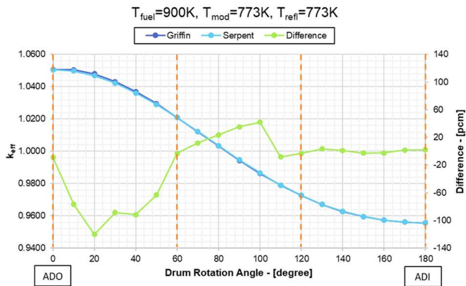
Figure 2: Example of cross-section efficacy study (dashed lines indicate cross-section evaluation point; Serpent uncertainty on keff <10 pcm).
