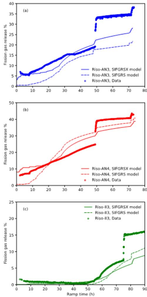
Figure 1: Fission gas release percentage, as a function of time, during the (a) Riso-AN3, (b) Riso-AN4, and (c) Riso-II3 ramp tests. Open circles represent experimental measurements and solid lines represent SIFGRSX model predictions. Original SIFGRS model results are shown in dashed lines for comparison.
