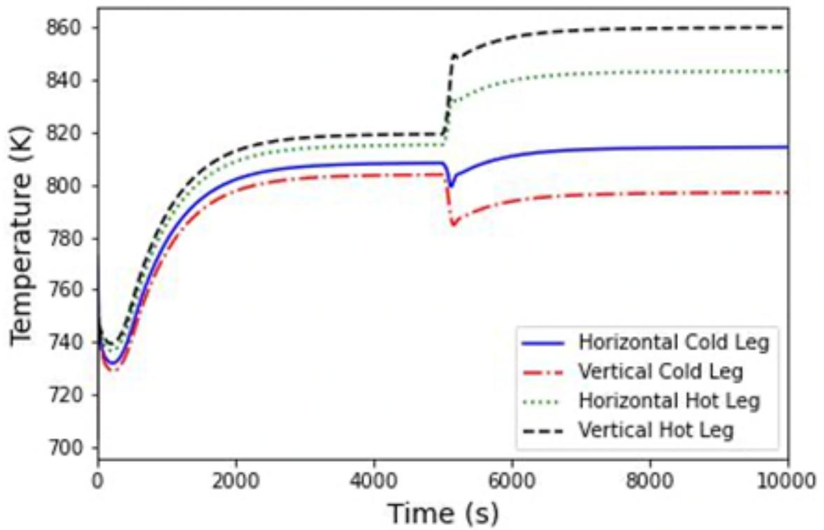
Figure 3: Hypothetical LOFA transient in RELAP5-3D model of loop.
