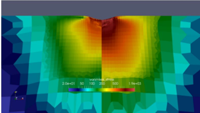
Figure 1: Von Mises stress 0.0 seconds into the holding phase comparing loading rates of 100 and 800 nm/s with a stress exponent of 10. The stress in 800 nm/s is much higher.
