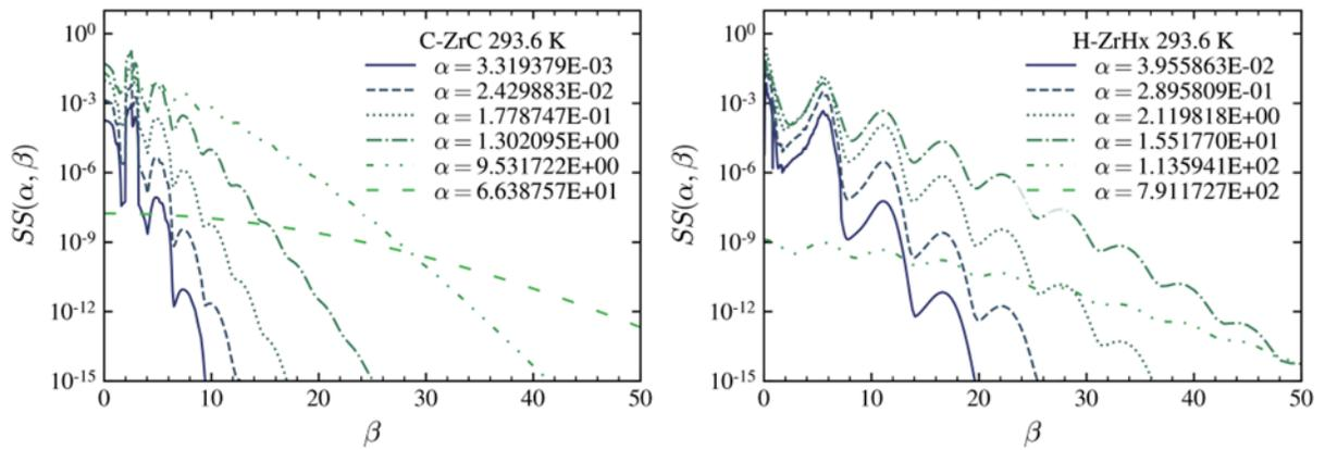
Figure 1: Symmetric TSL of C(ZrC) and H(ZrHx) evaluated with the FLASSH code and phonon spectra from ab initio lattice dynamics and ab initio molecular dynamics methods, respectively. These TSL evaluations have been submitted for inclusion in the ENDF/B-VIII.1 nuclear data library. Both materials exhibit quantized oscillations as a function of unitless energy transfer.
