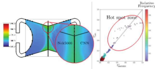
Figure 2: CNN field reconstruction at  $Re = 300k$ . A detailed view is shown for the peaking temperature region. The right-side plot compares the predictions from the CNN with the CFD solution. A red circle highlights probing points near the peaking temperature region, termed the hot spot zone.
