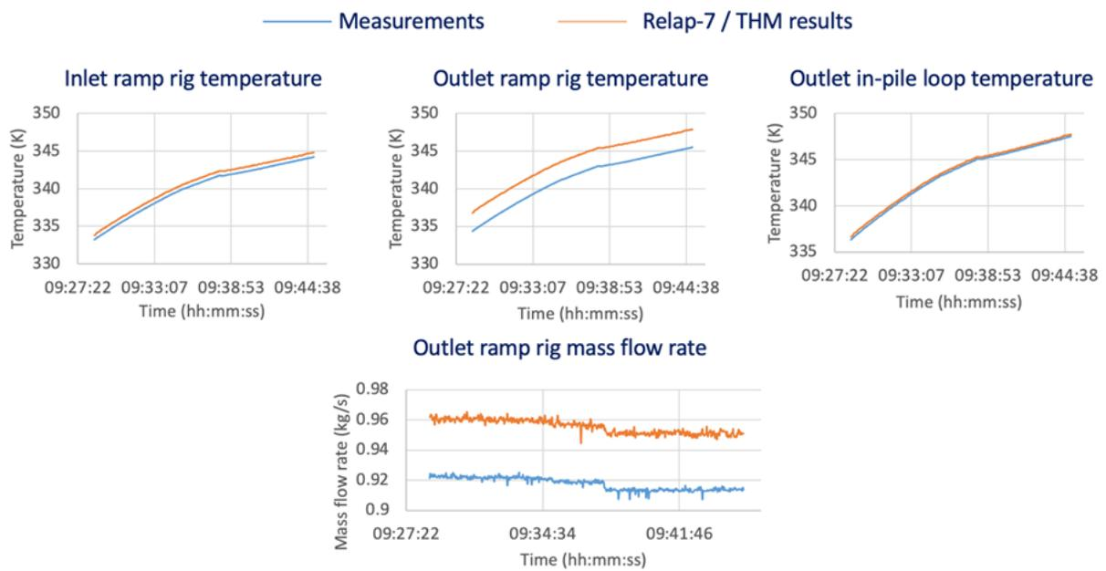
Figure 1: RELAP-7 and THM results, showing that some calibration of the loss coefficient is needed.
