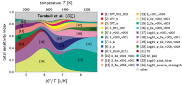
Figure 1: Parameter sensitivities as a function of temperature for xenon gas release under irradiation conditions under the conditions reported in Turnbull et al. (1982).
