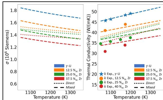
Figure 2: Thermal and Electrical Conductivity of U-Zr Systems: Left: Calculated direct and mixed for U-Zr systems, with direct and mixed for U for comparison. Right: Calculated  $k_e$  direct and  $k_e$  mixed are compared against experimental  $k$  [Touloukian et. al 1970], [ANL-87-19 1986] for U-Zr systems. Calculated  $k_e$  direct,  $k_e$  mixed, and experimental  $k$  [Ho et. al 1972] for U is included for comparison.
