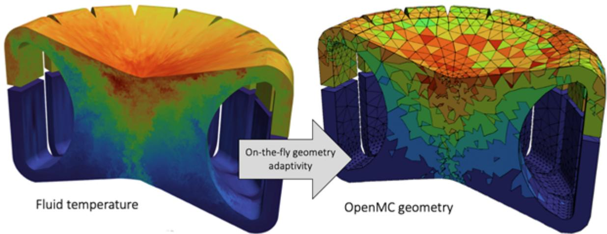
Figure 1: Multiphysics simulation of an MSR, which couples NekRS and OpenMC. Left: NekRS fluid temperature. Right: OpenMC on-the-fly regenerated cell boundaries.
