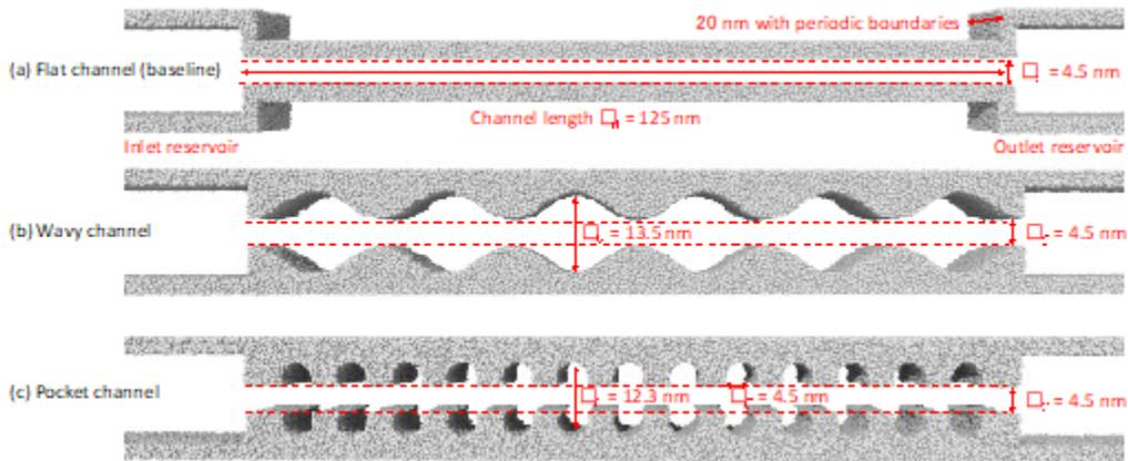
Figure 1: Visualization of the three channel geometries: (a) flat channel, (b) wavy channel, and (c) pocket channel. The full extent of the inlet and outlet reservoirs are not pictured here.
