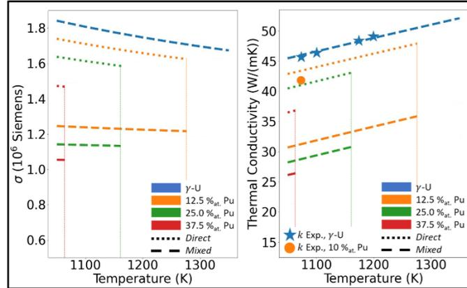
Figure 1: Thermal and electrical conductivity of U-Pu systems.
