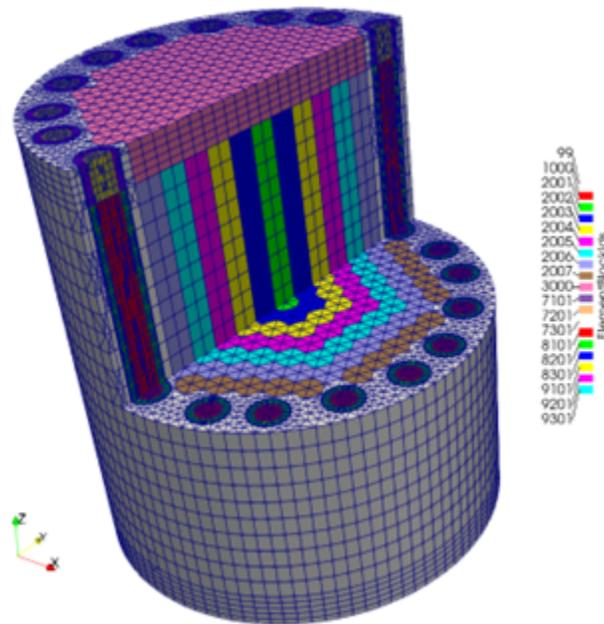
Figure 1: Griffin neutronics mesh (colors represent Block IDs).
