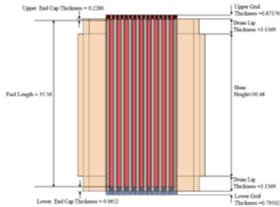
Figure 1: Dimensioned axial view of the S8ER.
