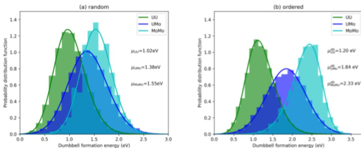
Figure 1: Distributions of interstitial dumbbell formation energies in the (a) random solid solution and (b) the SRO state at 300 K. Substantial increases can be seen in the formation energies of different dumbbells because of SRO.
