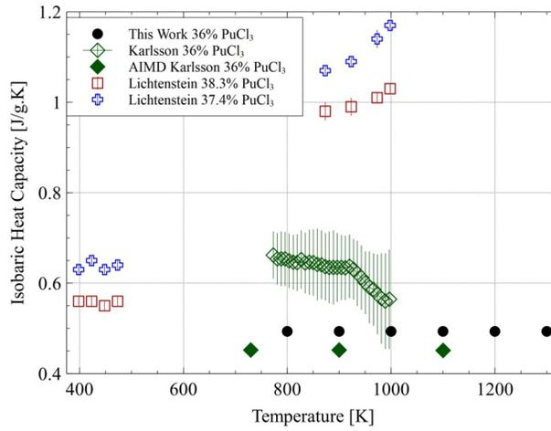
Figure 2: Heat Capacity for eutectic NaCl-PuCl<sub>3</sub>.
