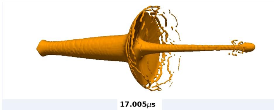
Figure 1: 3D formation model of a shaped charge jet run using ALEGRA deployed in an Apptainer container.
