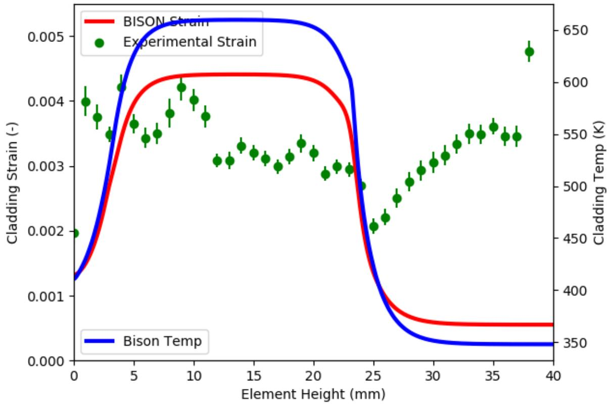
Figure 2: FAST-008 experimental vs. BISON-simulated strain comparison.
