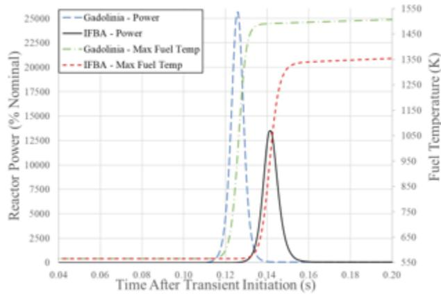
Figure 1: Control rod ejection transients of IFBA and gadolinia core.
