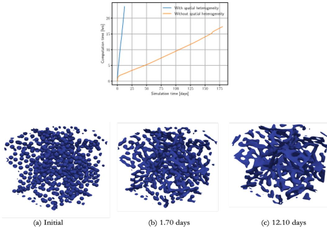
Figure 2: Intergranular gas bubble evolution for the  $203 \mu\text{m}^3$  10-grain polycrystal with spatially heterogeneous diffusivities at the initial condition,  $t = 1.7$  days, and 12.1 days in (a)–(c), respectively. However, the very short time reached in this coupled simulation precludes any meaningful analysis of the intragranular xenon clustering and bubble evolution.
