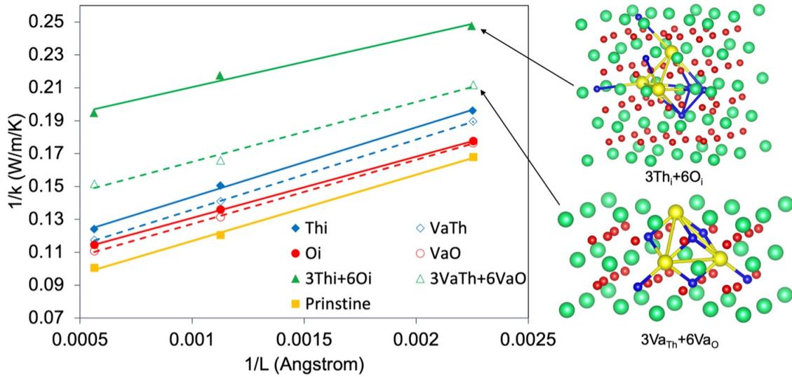
Figure 1: The impact of atomic-scale defects on the thermal conductivity of thorium dioxide.
