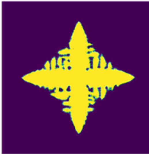
Figure 2: Predicted dendrite of Fe-C at the first timestep in microstructure evolution by a model trained on a large dataset.
