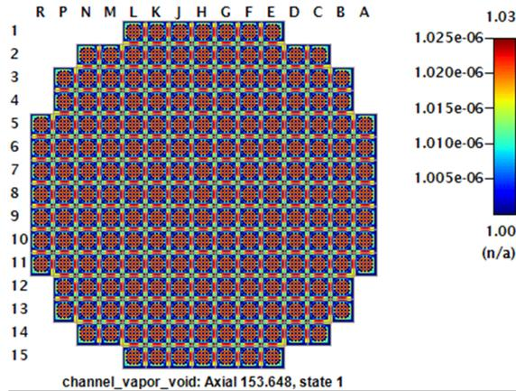
Figure 1: VERA simulation of reactor core void fraction distribution.
