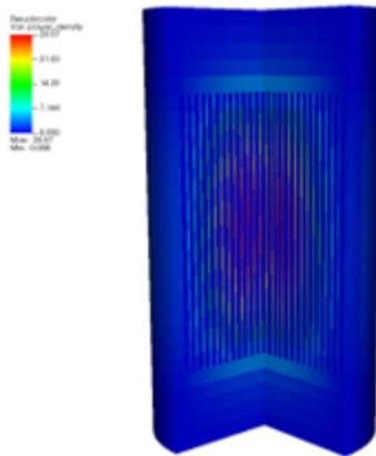
Figure 2: Power density in the Griffin MSRE model.
