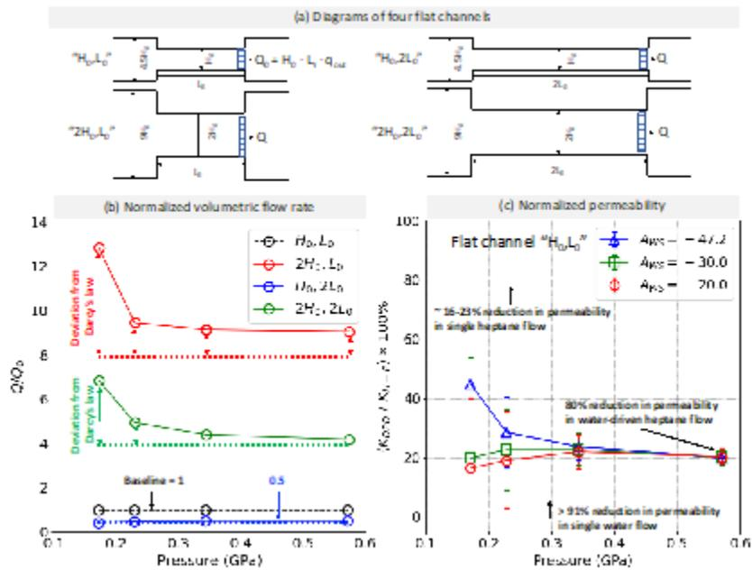
Figure 2: (a) Diagrams of four flat channels with relevant dimensions and the flow rate measurement region. (b) Plot of the normalized volumetric flow rate. (c) Plot of the normalized permeability.  $H_0 = 4.5$  nm and  $L_0 = 125$  nm are the default flat channel height and length, respectively.
