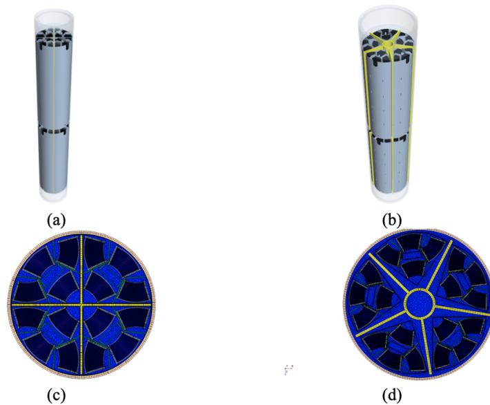
Figure 1: The geometry layout for (a) 18 inch diameter and (b) 24 inch diameter canisters, and the meshed geometry for (c) 18 inch diameter and (d) 24 inch diameter canisters.
