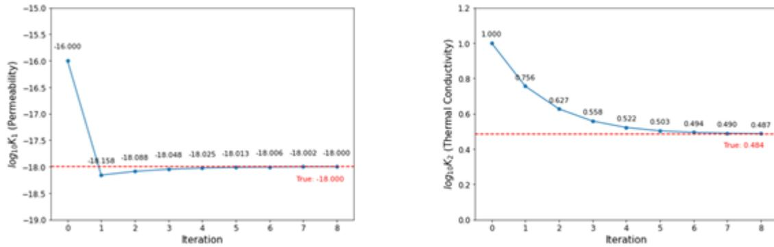
Figure 1: Estimation of permeability and thermal conductivity of the granitoid layer, assuming that the permeability and thermal conductivity are homogeneous and isotropic.
