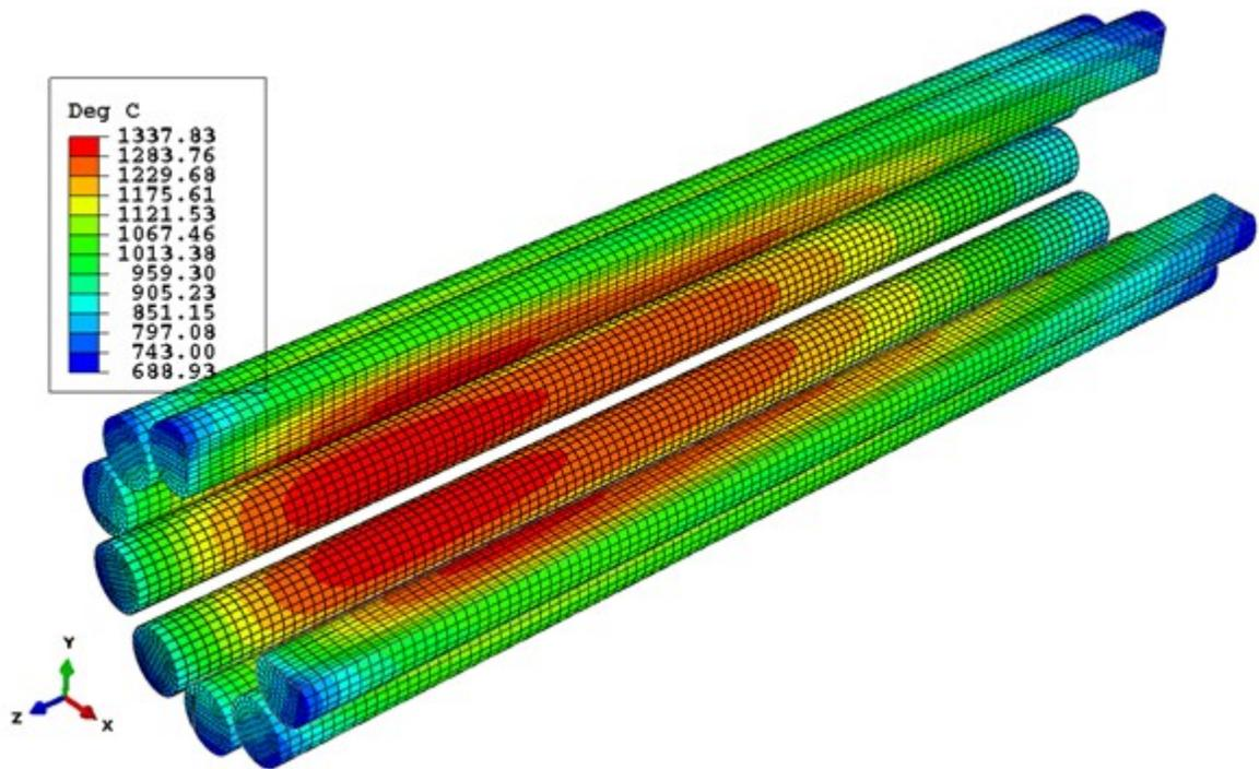
Figure 2: Typical temperature ( $^{\circ}\text{C}$ ) of the fuel in Capsule 1 of the AGR-5/6/7 experiment.
