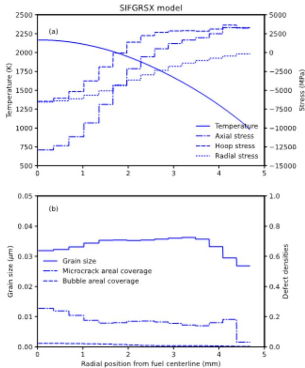
Figure 2: SIFGRSX model results for the variation of (a) temperature, axial stress, hoop stress, and radial stress and of (b) grain size, microcrack areal coverage, and bubble areal coverage, with the radial position from the centerline of the fuel rod, immediately after the temperature transient 48 hours after the start of the Riso-AN3 ramp test.
