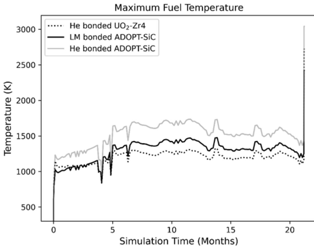
Figure 1: Calculated maximum fuel temperature comparison.
