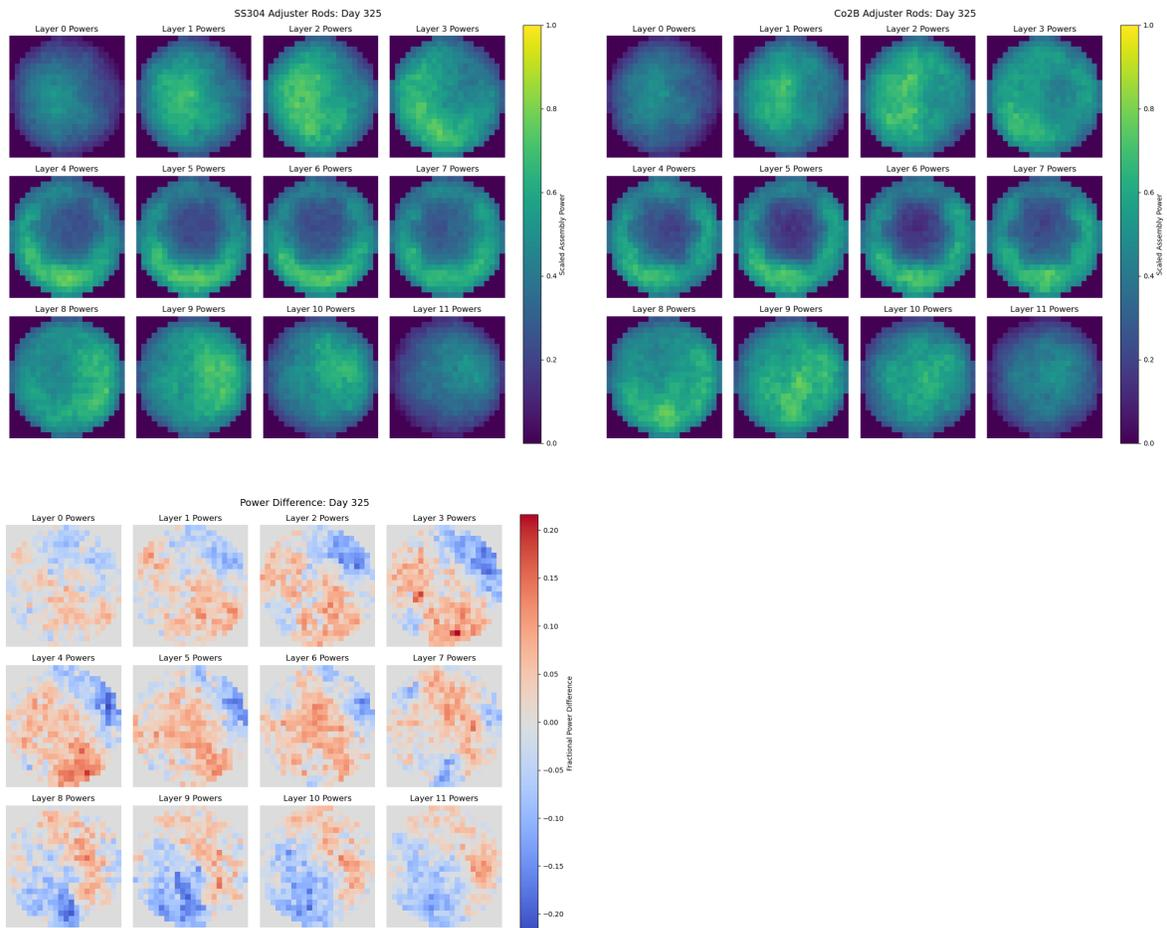
Figure 1: Comparison of assembly powers between the reference case (SS304) and perturbed case (Co2B).
