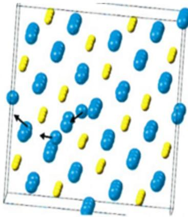
Figure 2: Interstitial diffusion mechanism.
