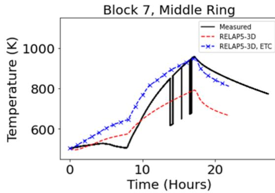
Figure 2: Comparison of RELAP5-3D (nominal and calibrated) results compared to measured data for HTTF experiment PG-29.
