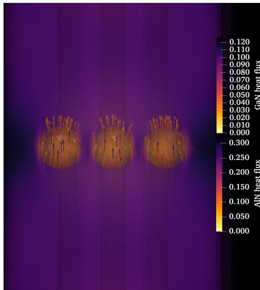
Figure 2: Heat flux streamlines in barricade geometry of GaN defects in AlN bulk, seven axial layers.
