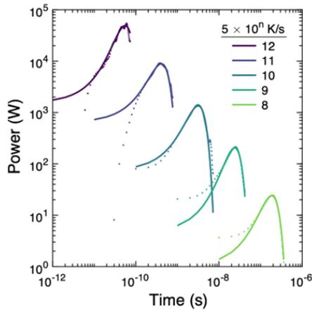
Figure 2: The energy release is differentiated to determine the power output associated with defect recovery.
