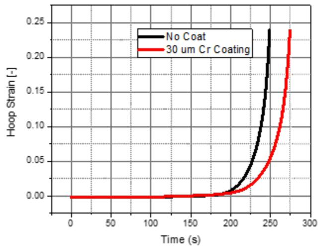
Figure 2: Maximum cladding hoop strain during the LOCA test sequence.
