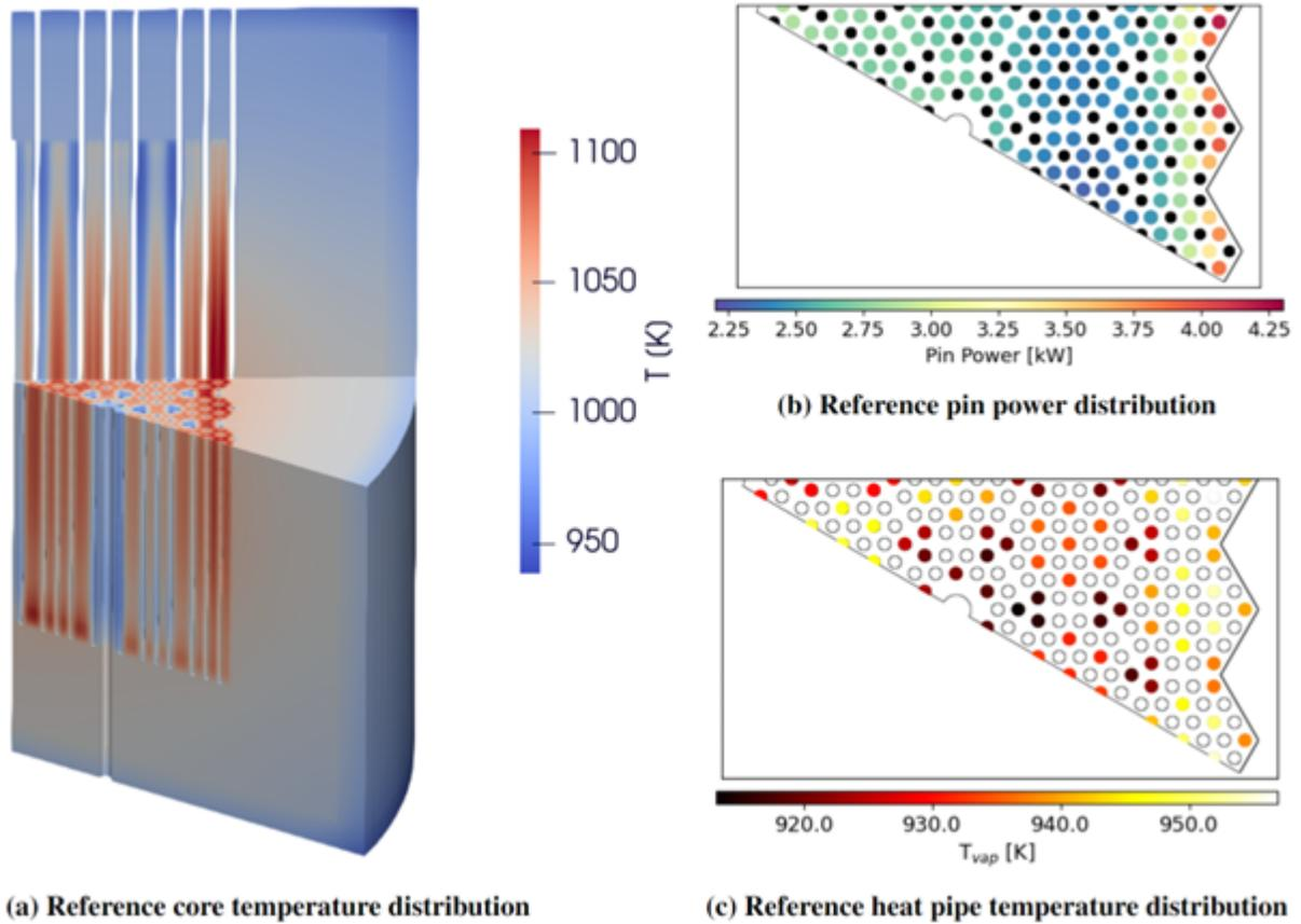
Figure 2: Reference core operating characteristics calculated with the multiphysics coupling procedure.
