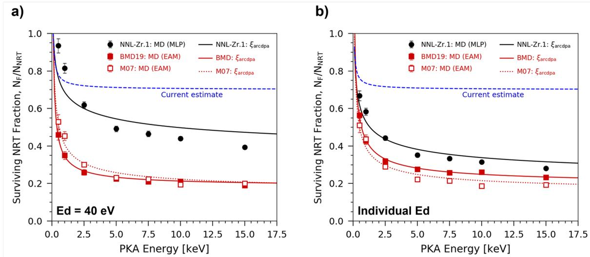
Figure 1: The surviving fraction of Frenkel pairs that survive post-cascade at  $T = 8$  K compared to the NRT-predicted number of stable defects when calculated with: a) the standard  $E_d = 40$  eV for each potential or b) the individual ( $E_d$ ) values calculated for each potential. The arc-dpa damage efficiency function, arc-dpa, is fit to the averaged MD results. Error bars represent the standard error of the mean.
