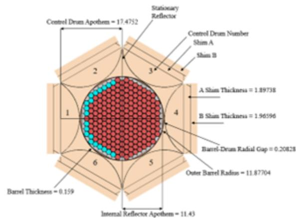
Figure 2: Dimensioned radial view of the S8ER.
