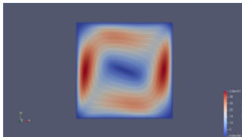
Figure 1: Neural-network-generated velocity field.
