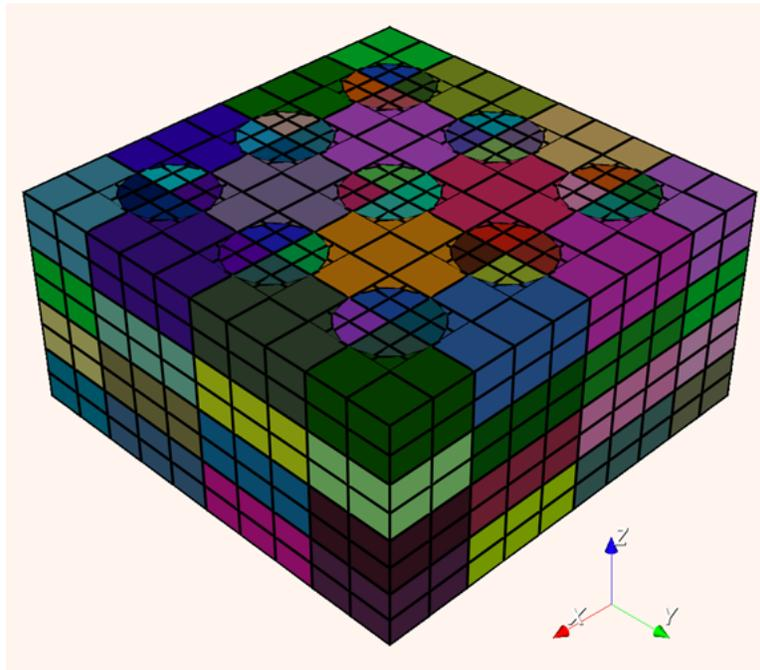
Figure 1: Meshed  $3 \times 3$  assembly with a thermal grid.
