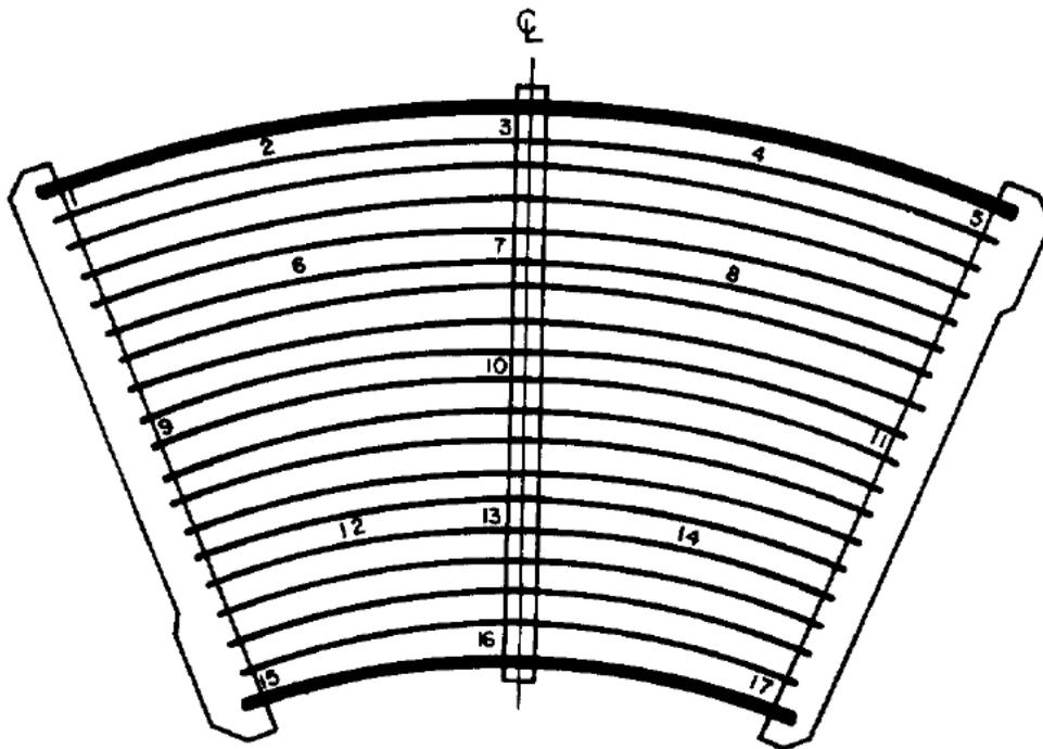
Figure 1: Location of the fission wires used to measure the fuel element power distribution.
