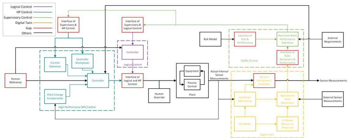
Figure 1: Operational approach to integrate advanced control methods and digital twins for advanced nuclear reactors.
