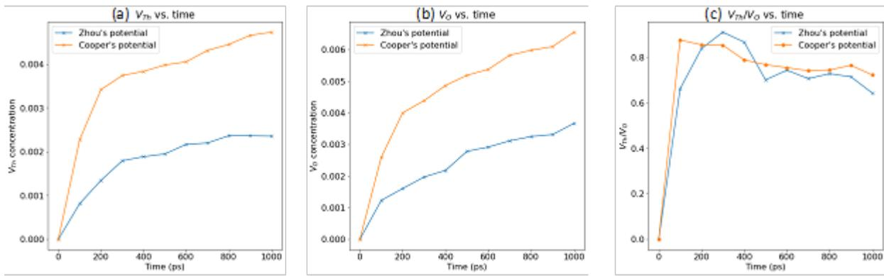
Figure 1: Concentrations of (a) Th vacancy ( $V_{Th}$ ) and (b) O vacancy ( $V_o$ ) and (c) the ratio of  $V_{Th}/V_o$  as functions of time.
