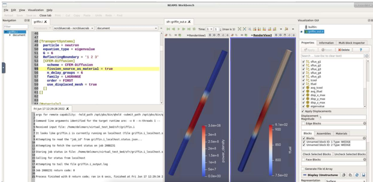
Figure 1: The NEAMS workbench GUI with `griffin.i` input file (top left), the output from the scheduler (bottom left), and the numerical solution visualized with embedded ParaView (right).
