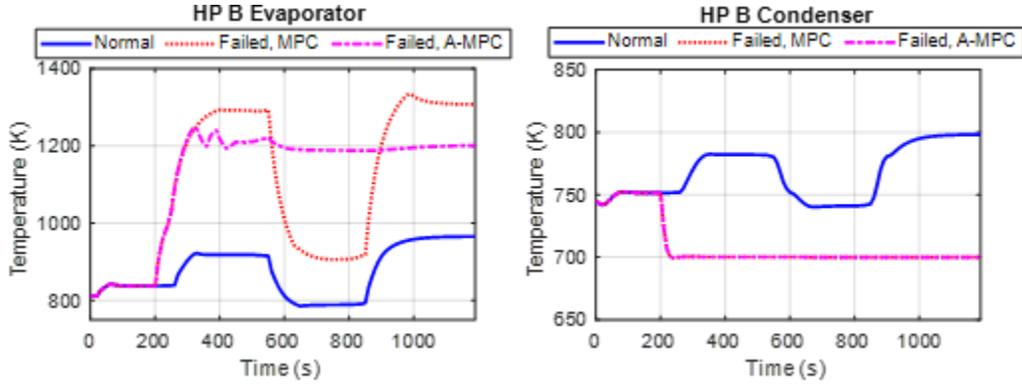
Figure 5: HP B temperature under HP B and C failure conditions.
