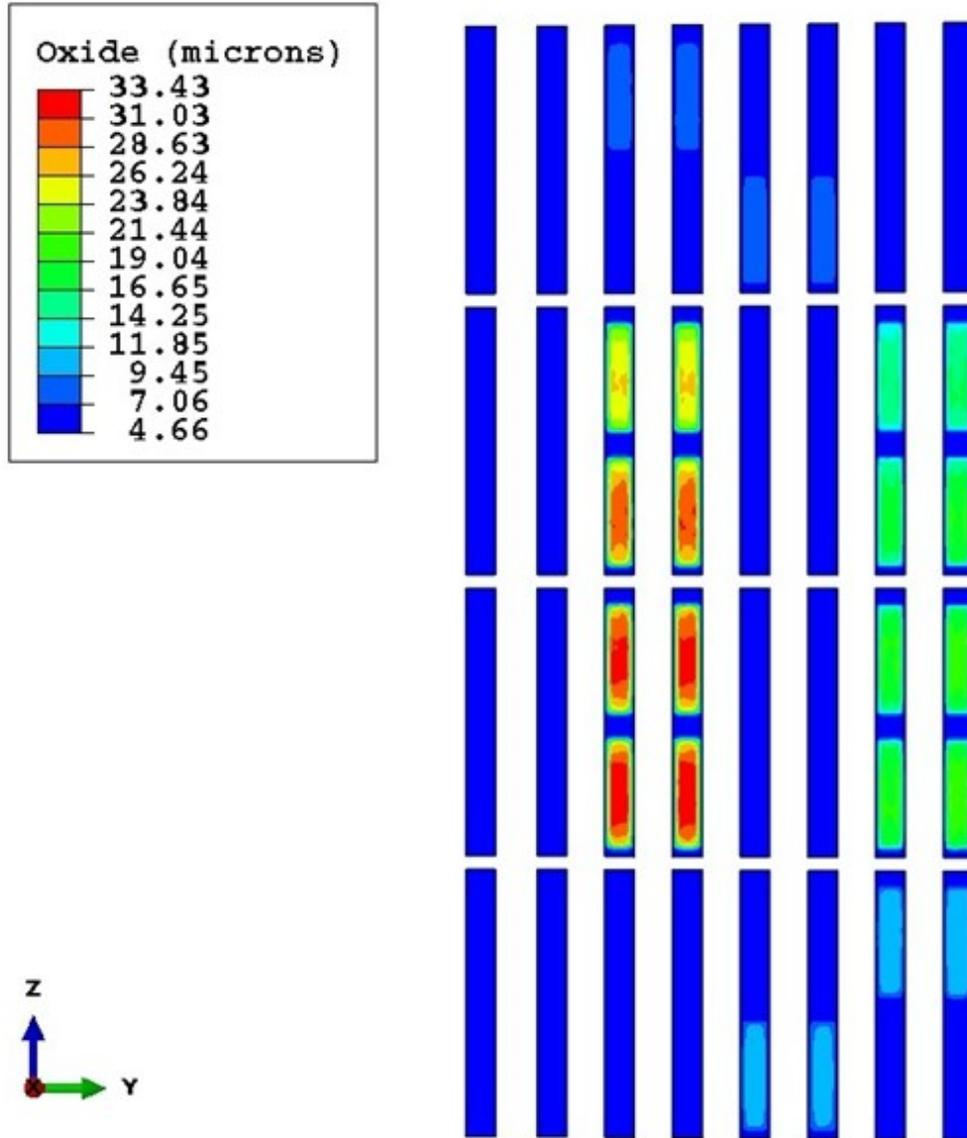
Figure 2: Oxide growth (microns) on MP-2 plates at end of irradiation.
