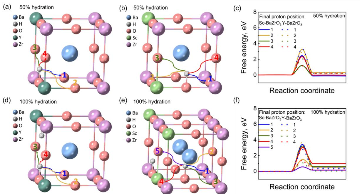
Figure 1: DFT calculation for proton migration of 25 mol% Sc or Y-doped BaZrO<sub>3</sub>. (a–b) Proton migration paths in the lattice at 50% of hydration. (c) Potential energy profiles for the proton migration paths in (a–b). (d–e) Proton migration paths in the lattice at 100% of hydration. (f) Potential energy profiles for the proton migration paths in (d–e).
