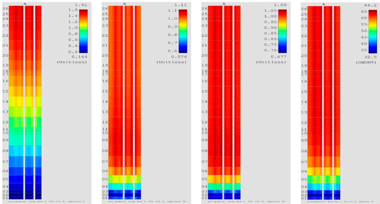
Figure 1: Axial relative power distribution at 0, 30,000, and 60,000 MWD/MTU and burnup distribution at 60,000 MWD/MTU of the NPP Krako  $16 \times 16$  fuel.
