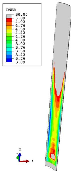
Figure 3: MURR-DDE Plate 4 minimum DNBR during RIA2 transient.
