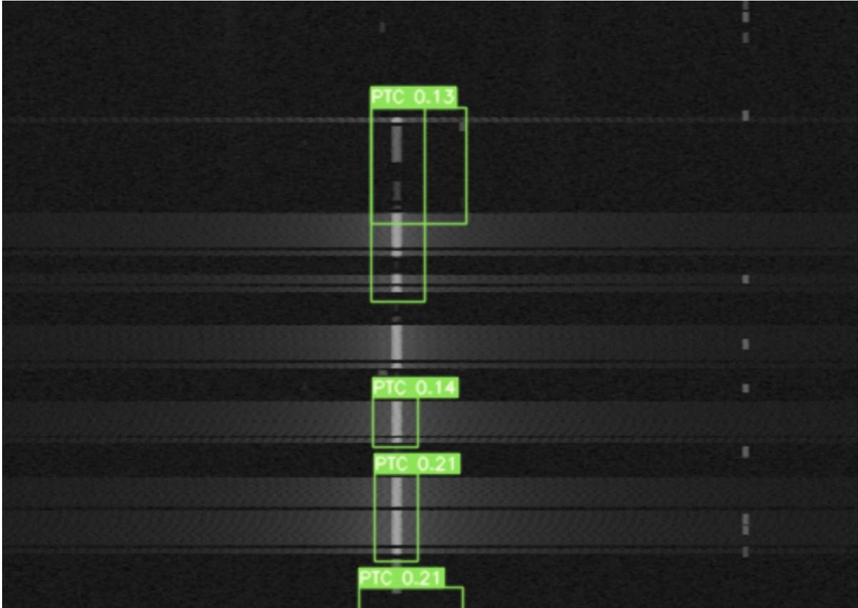
Figure 1: Identification of positive train control and narrow band FM RF signals.
