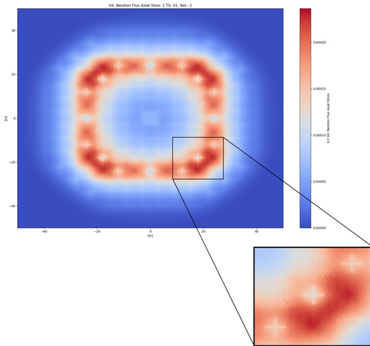
Figure 1: Neutron flux distribution in the PWR-1 core.
