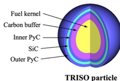
Figure 1: TRISO fuel particle.
