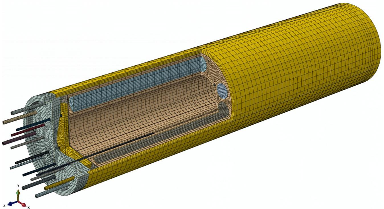
Figure 1: Finite-element mesh of Capsule 1 of the AGR-5/6/7 experiment.
