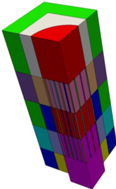
Figure 1: Deimos 1/4th radial, full-axial geometry, and mesh created in Cubit.
