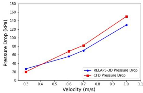
Figure 2: Comparison of pressure drop calculations between RELAP5-3D and CFD [1] in specimen holder.
