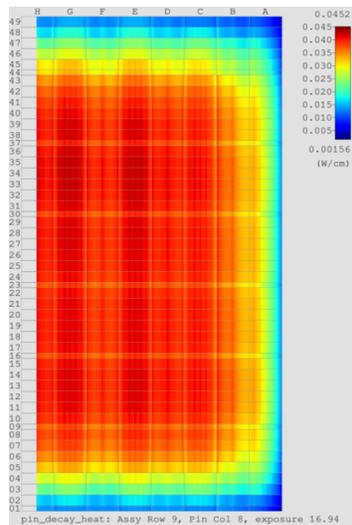
Figure 3: Radial and axial decay heat distribution after 1 year of cooling—Watts Bar Unit 1 Cycle 1.
