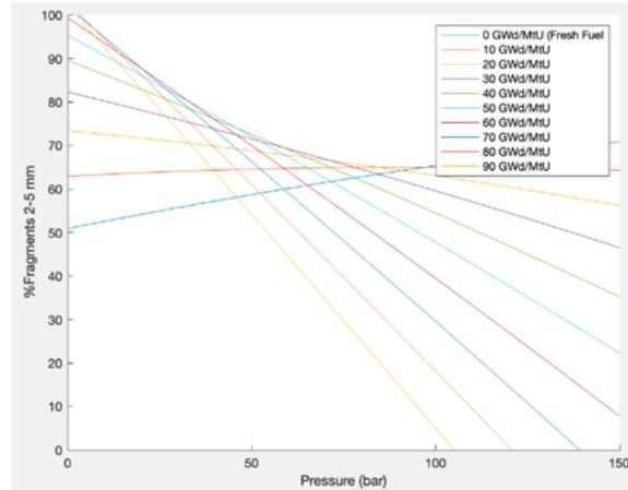
Figure 1: Preliminary fit for fraction of 2–5 mm fuel pellet fragments post-LOCA as a function of burnup.
