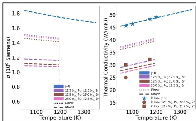
Figure 3: Thermal and electrical conductivity of U-Pu-Zr systems.
