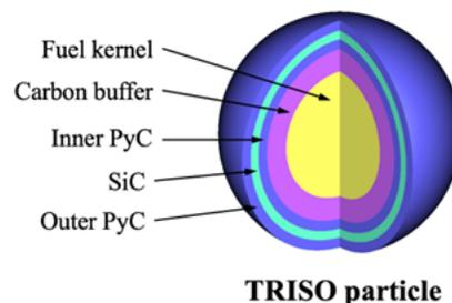
Figure 1: TRISO fuel particle.
