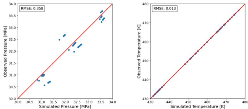
Figure 3: Pressure and temperature data fitting of the heterogeneous case. The fitting error is shown as the root mean square error.
