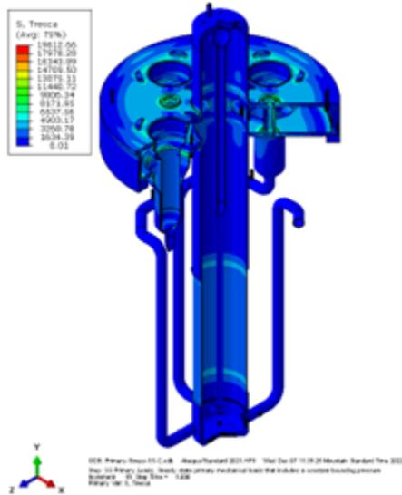
Figure 2: Primary stress intensity for normal operating conditions.
