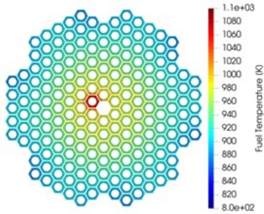
Figure 1: Coupled multiphysics prediction of fuel temperature with a single heat pipe failure in the INL Design A microreactor.
