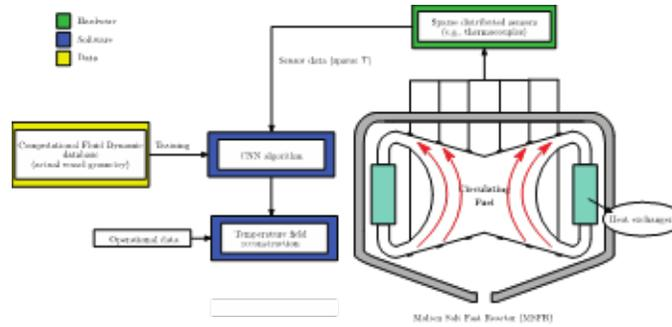
Figure 1: Temperature field reconstruction employing the novel CNN algorithm.
