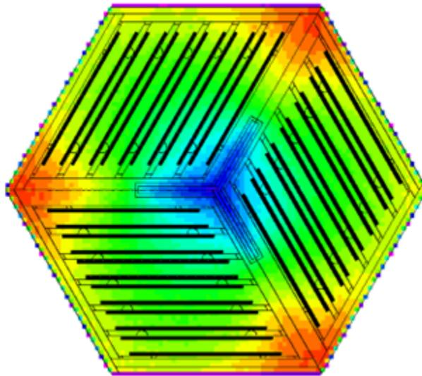
Figure 1: Thermal neutron flux in core midplane during control rod insertion, showing thermal flux shifting to assembly periphery due to thermal absorber placement.
