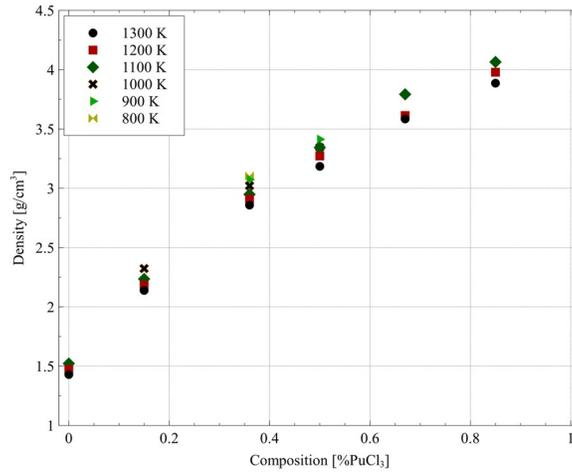
Figure 1: NaCl-PuCl<sub>3</sub> density.
