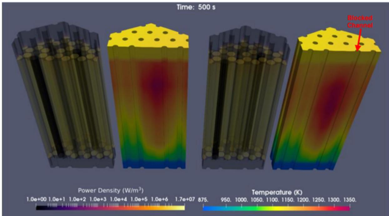
Figure 1: A typical power density and temperature profile of a gas-cooled microreactor assembly after a single channel blockage incident as predicted by multiphysics models using diffusion (left) and CMFD DFEM-SN (right) neutronics approaches.
