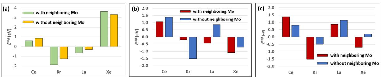
Figure 2: Segregation energy of fission products (Ce, Kr, La, Xe) at the (a) coherent interface, (b) misfit region in the semicoherent interface, and (c) coherent region in the semicoherent interface.
