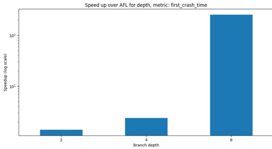
Figure 1: Speedup of our approach over AFL versus nested branch depth.
