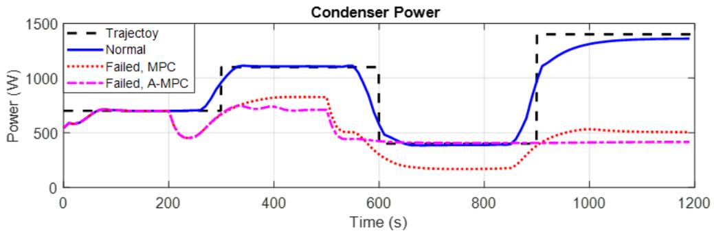
Figure 6: Average HP condenser power output under HP B and C failure conditions.
