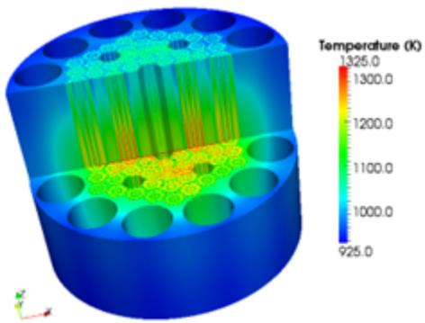
Figure 3: Temperature distribution at time of maximum fuel temperature (3.66 seconds) during an inadvertent drum rotation accident.
