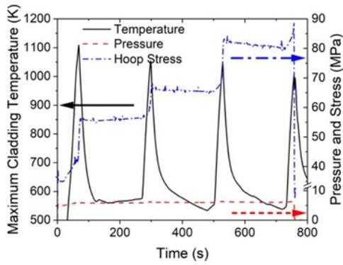
Figure 1: Applied boundary conditions and BISON-calculated hoop stress during the cyclic dryout test.
