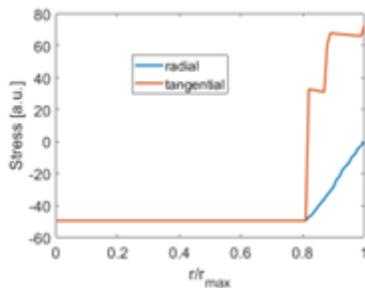
Figure 1: Stress profile in particle.
