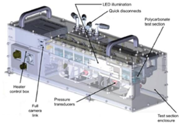
Figure 1: ISS flow boiling module.
