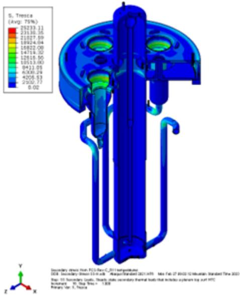
Figure 3: Secondary stress intensity for normal operating conditions.
