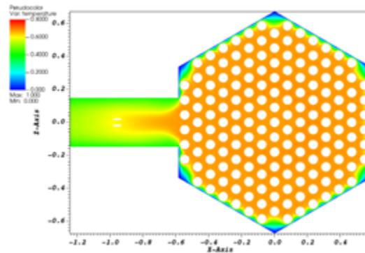
Figure 2: Time-averaged velocity field (nondimensional) in the lower plenum at  $y=-0.1$  m.
