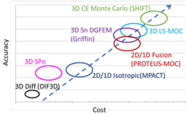
Figure 1: Accuracy vs. cost of various neutronics methods.
