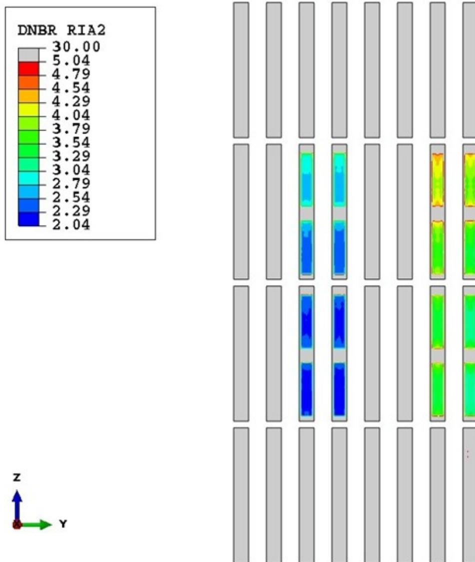
Figure 1: MP-2 minimum DNBR on plate surfaces during RIA2 transient.
