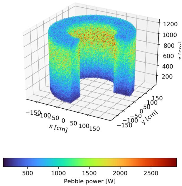
Figure 1: 3D representation of pebbles in an HTGR core showing pebble power distributions at equilibrium.
