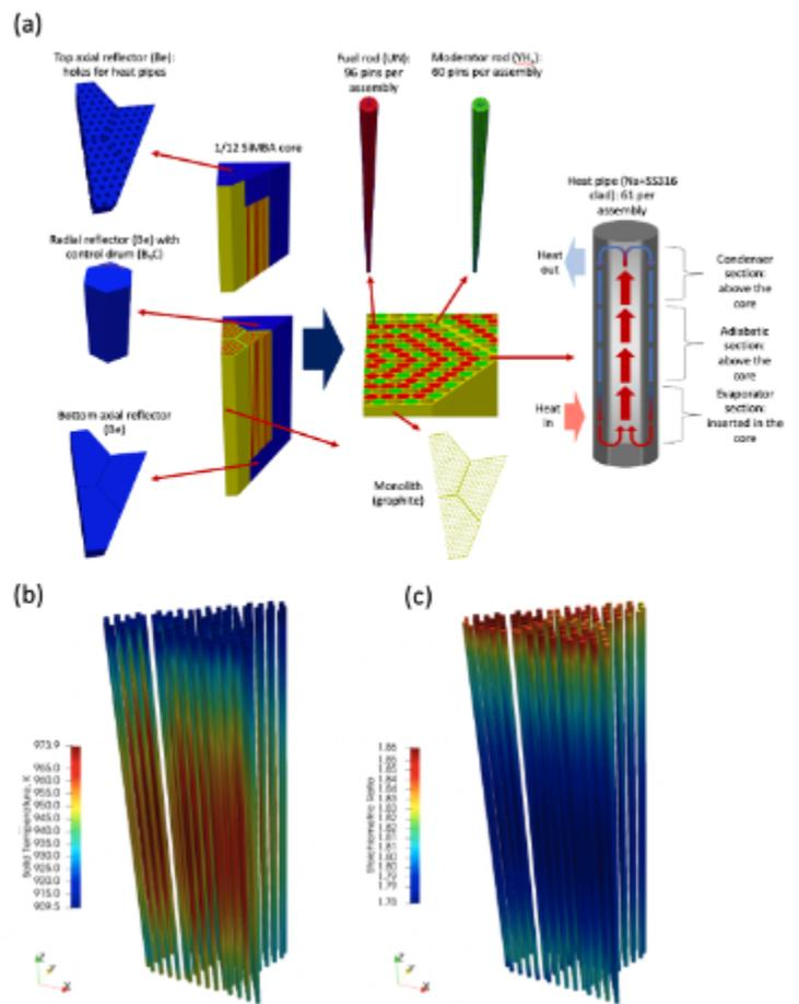
Figure 1: (a) Simplified microreactor benchmark assessment problem overview, (b) computed temperature, and (c) computed hydrogen stoichiometric ratio in the YH<sub>x</sub> moderator pins.
