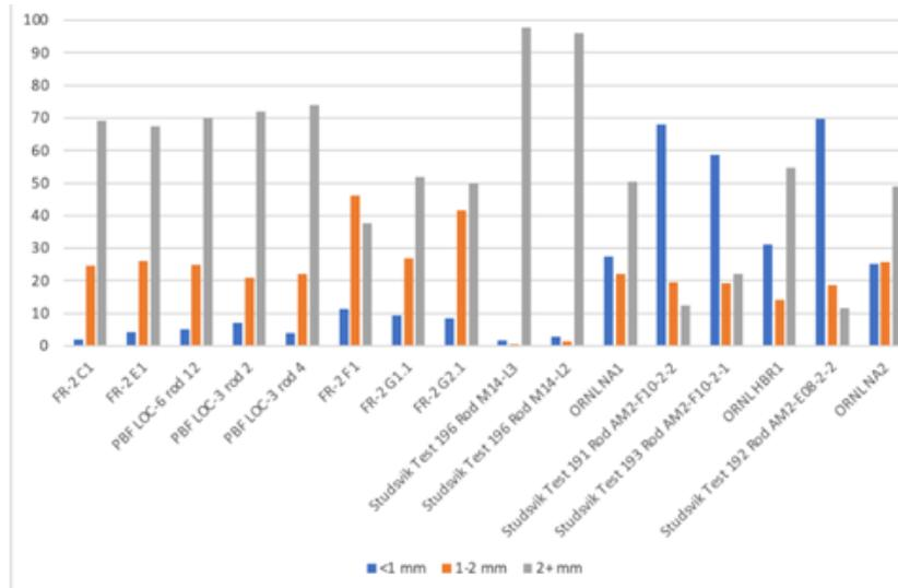
Figure 2: Existing fuel fragment size distribution data from LOCA testing.
