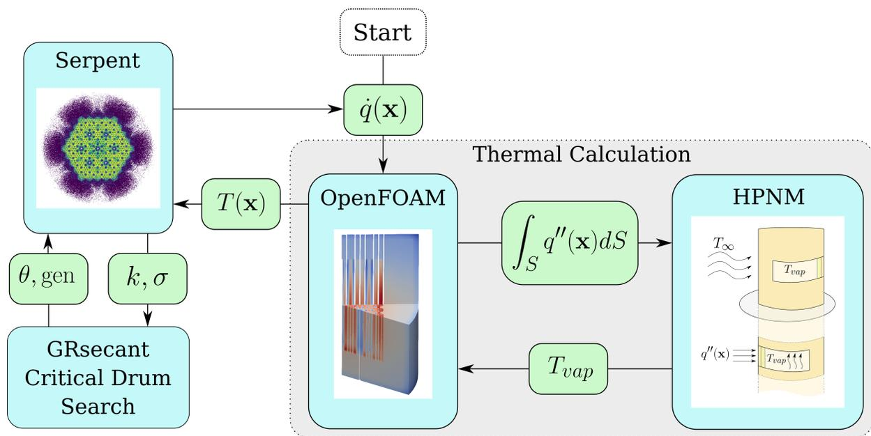
Figure 1: Coupling procedure used for simulating the heat-pipe microreactor.
