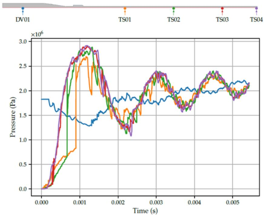
Figure 1: Coupled STAR-CCM+ Serpent 2 pressure results for the 250 psi initial pressure OSTR helium-3 injection experiment.
