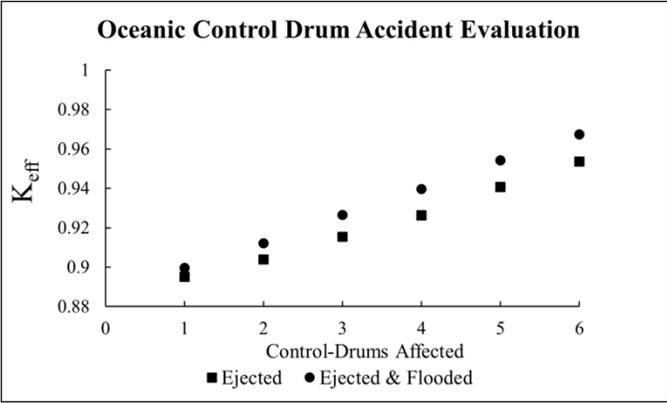
Figure 1: Criticality safety evaluation for a launch failure and subsequent oceanic submersion with affected control drums.
