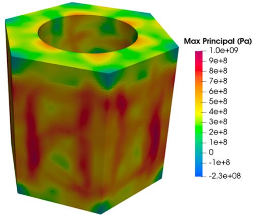
Figure 1: a) Can stress and b) matrix stress at about  $7\times$  the expected energy deposition for the maximum accident condition for HTGRs.
