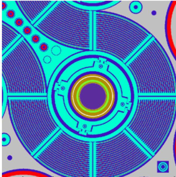
Figure 1: Standard ATR core.
