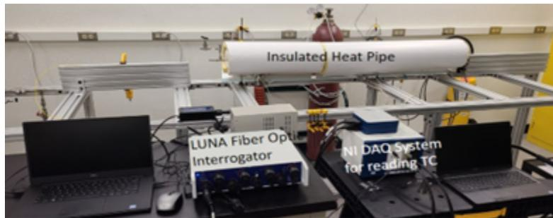
Figure 2: Heat-pipe design and experimental facility based on the Sockeye code simulations and current status.
