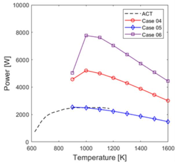
Figure 2: Capillary limit for Cases 04, 05, and 06 with different liquid friction factor correlations.
