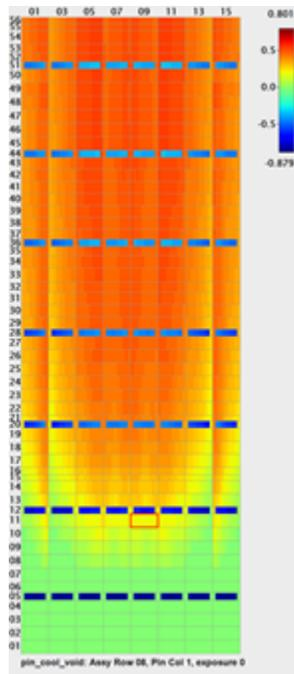
Figure 3: Axial void distribution BWR mini-core.
