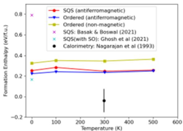
Figure 2: Formation enthalpy per unit formula of -UZr2 using GGA.
