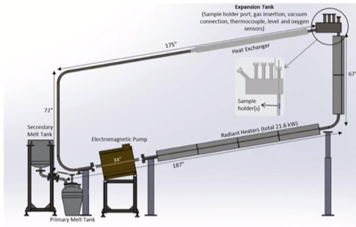
Figure 1: Diagram of the Lobo Lead Loop Facility [1].
