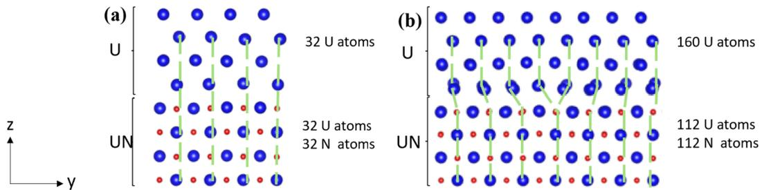
Figure 1: The relaxed U/UN interfaces: (a) coherent interface and (b) semicoherent interface. Orientation relationship:  $[001] \text{ U} \parallel [001] \text{ UN}$  and  $(100) \text{ U} \parallel (110) \text{ UN}$ .
