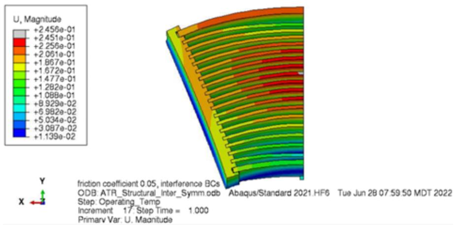
Figure 2: Finite element analysis distortion results.
