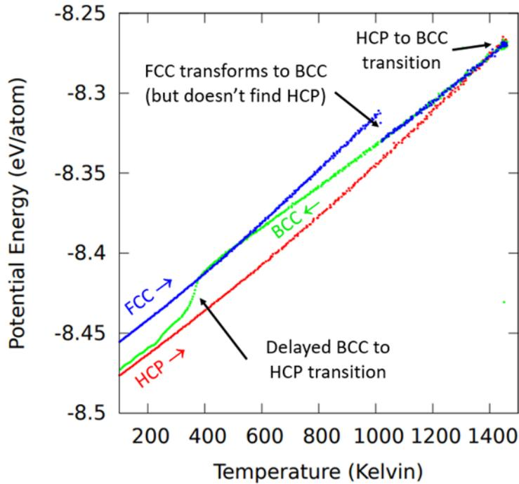
Figure 1: Potential energy trends for phase changes from heating and cooling simulations. HCP transforms to BCC when heated above 1400 K. Significant undercooling is required to observe the BCC ! HCP transition for the ramp rates of this MD study. Upon heating, FCC transforms to BCC near 1000 K bypassing any transition to HCP.
