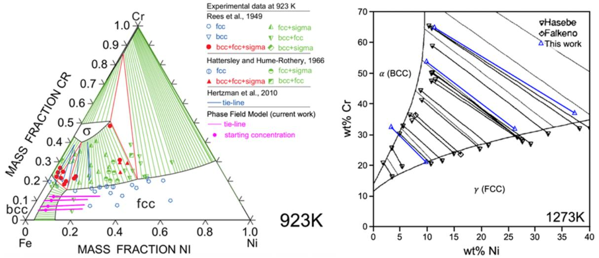
Figure 1: Experimental phase diagrams adapted from Xiong, W. [1] and Hillert, M., & Qiu, C. [2] with phase-field results overlaid.
