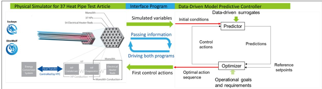
Figure 1: Schematic configurations for the anticipatory control system coupled with a 37 HP system with monolith block.
