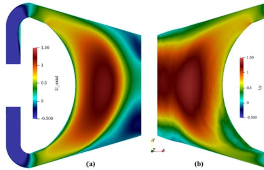
Figure 1: Comparison of the (a) RANS and (b) time-averaged LES results of axial velocity field.
