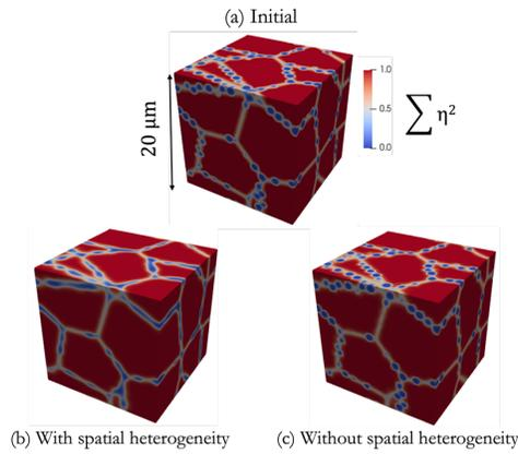
Figure 1: Bubble evolution in a  $203 \mu\text{m}^3$   $\text{UO}_2$  polycrystal with 10 grains and 600 initial intergranular bubbles. The initial microstructure is shown in (a), the simulation after 12 days with spatial heterogeneity in the Xe diffusivity is shown in (b), and the simulation after 180 days without spatial heterogeneity is shown in (c). (d) Computation time as a function of simulation time.
