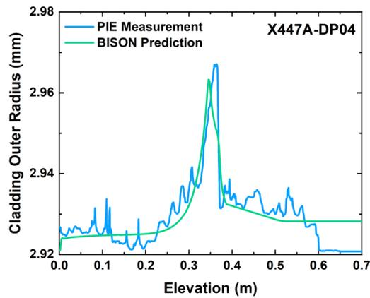
Figure 2: BISON-predicted cladding outer radius in comparison to profilometry measurement for Pin DP04.
