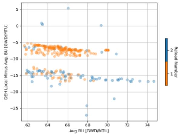
Figure 2: Difference between the local burnup at the PCT location and rod average burnup.
