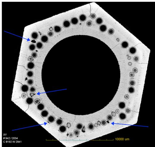
Figure 2: XCT image of a compact after 3,097 J/g-UN (99 ms FWHM) deposition, which is about  $7\times$  the maximum HTGR accident condition.
