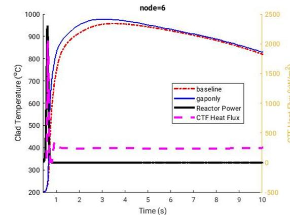
Figure 2: VERA simulation of fuel rod responses in a RIA scenario.
