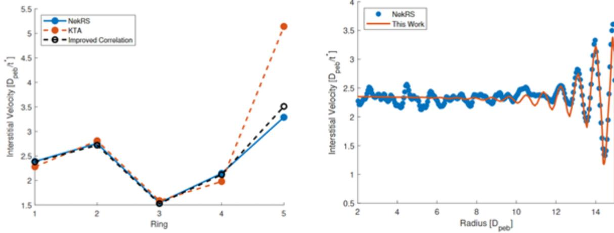
Figure 2: Radial velocity profiles from NekRS and Pronghorn with coarse (left) and fine (right) bed discretization, showing significant improvement over the KTA correlation.
