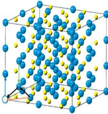
Figure 1: Vacancy diffusion mechanisms for U atoms.
