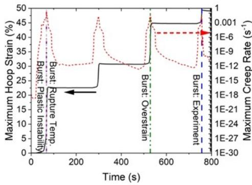
Figure 2: Zircaloy-2 cladding hoop strain and creep strain during the cyclic dryout test.
