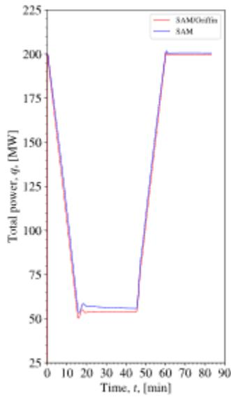
Figure 2: Comparison of the power levels during the load-following transient predicted by the SAM-Griffin and SAM-standalone models.
