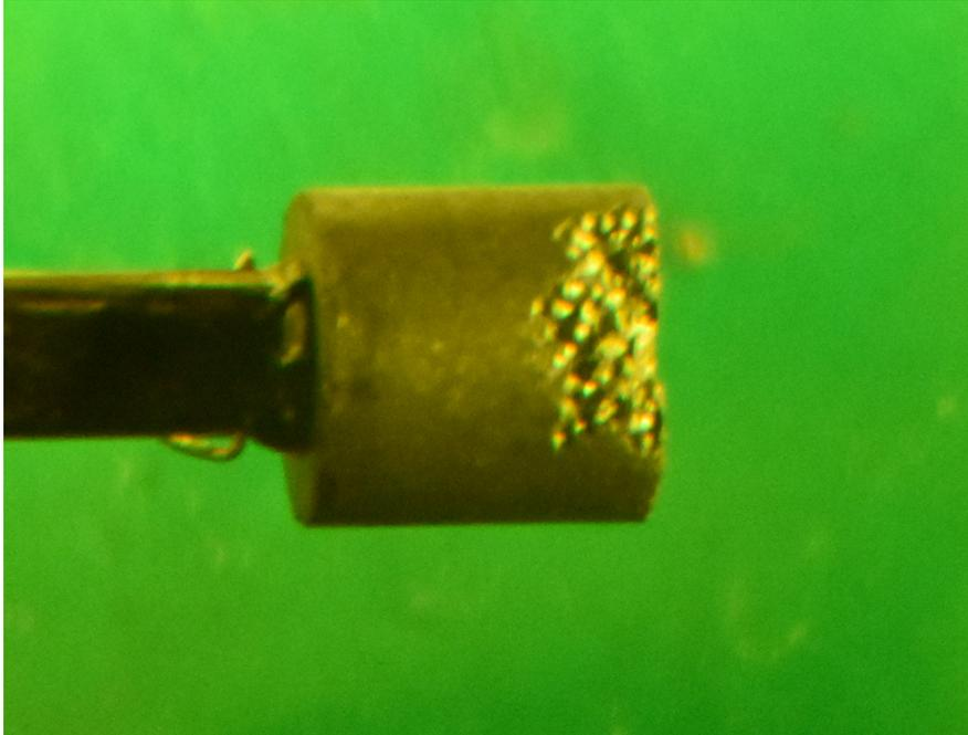
Figure 12. Pre-deconsolidation photo taken through the hot cell window showing a piece of material missing from Compact 7-3. The compact was pneumatically rabbited from HFEEF to AL, and the piece was missing when the compact was removed from the rabbit at AL.
