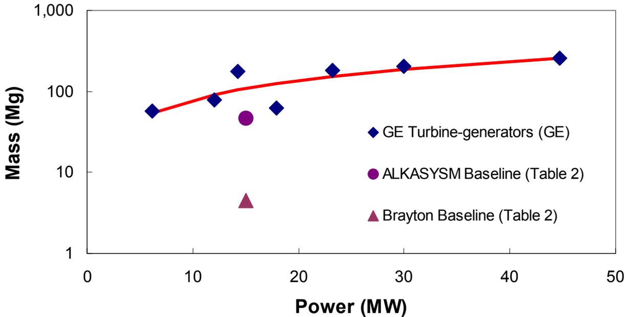
**Figure 10.** Comparison of commercial turbine masses with those predicted by the Glenn Research Center model and by ALKASYSM for baseline cases.
