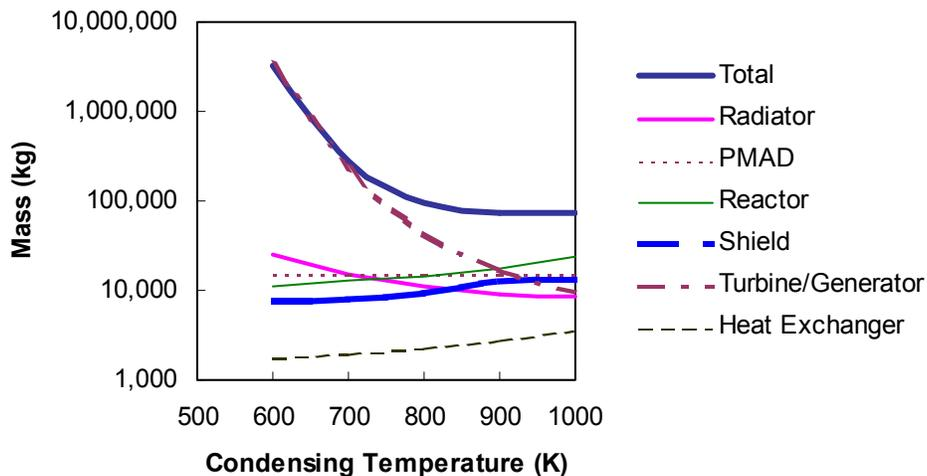
**Figure 12.** Variation in mass of Rankine system components with variations in condenser temperature for Li-cooled reactor having a 1,350-K turbine inlet temperature.
