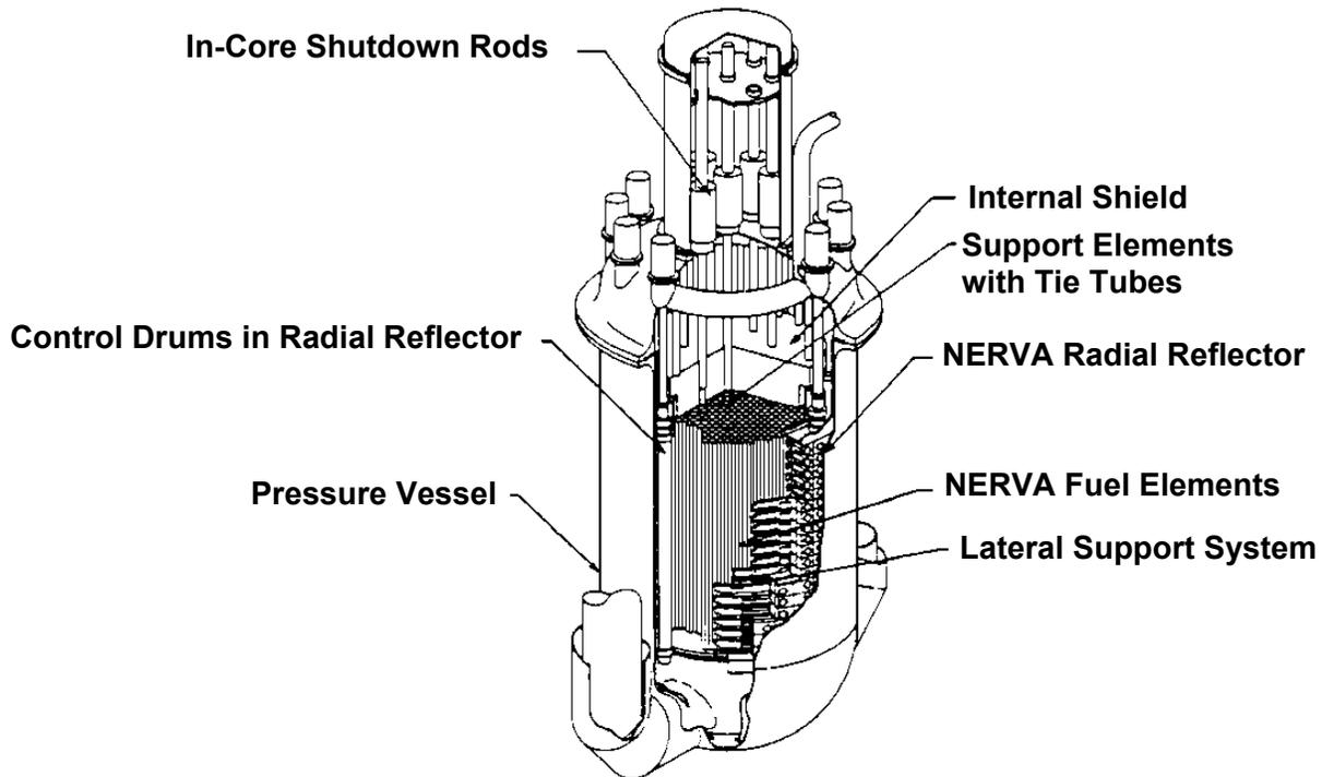
**Figure 4.** Configuration of the NERVA Derivative “Enabler” reactor design.
