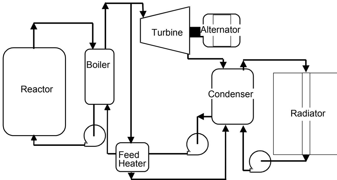
**Figure 6.** Liquid-metal cooled power system using the Rankine power cycle.
