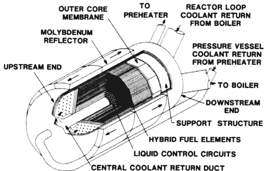
Figure 1. SPR-6 reactor configuration
