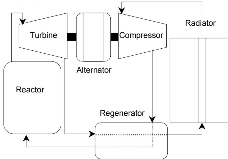
Figure 5. Typical Brayton cycle configuration.
