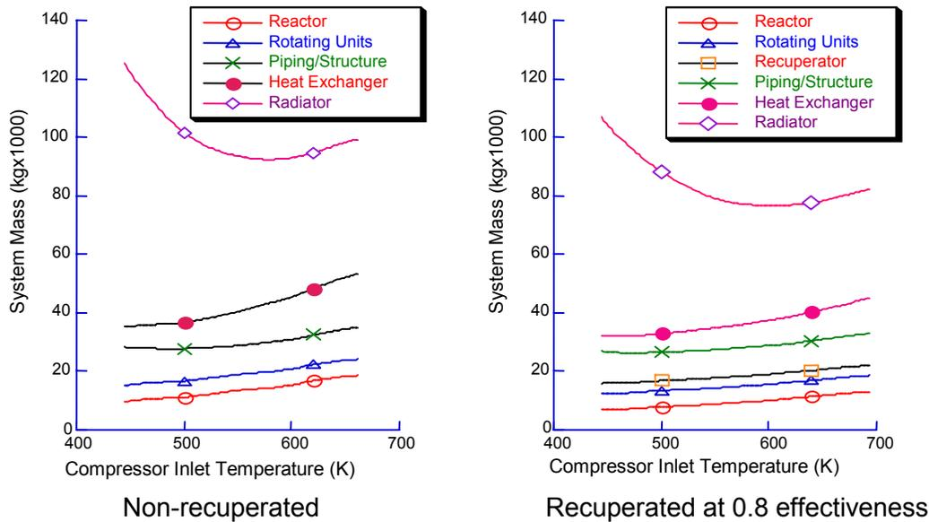
**Figure 9.** Cumulative system masses for various segments of a proposed Brayton cycle power system (from Wetch<sup>25</sup>).
