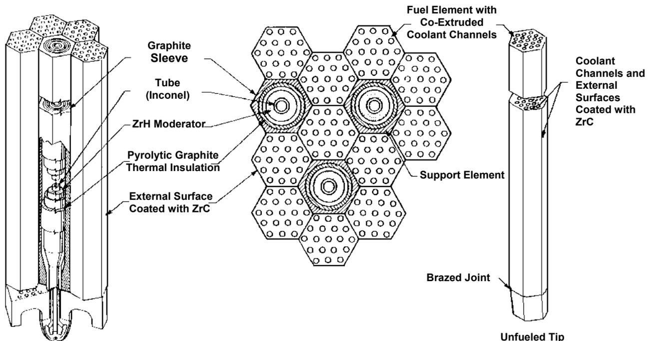
Figure 3. NERVA fuel configuration.
