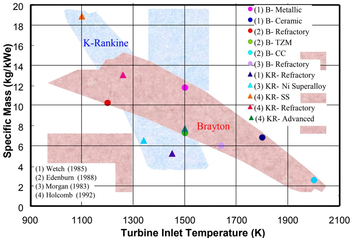
**Figure 7.** Specific mass trends for Rankine and Brayton systems as a function of turbine inlet temperatures.
