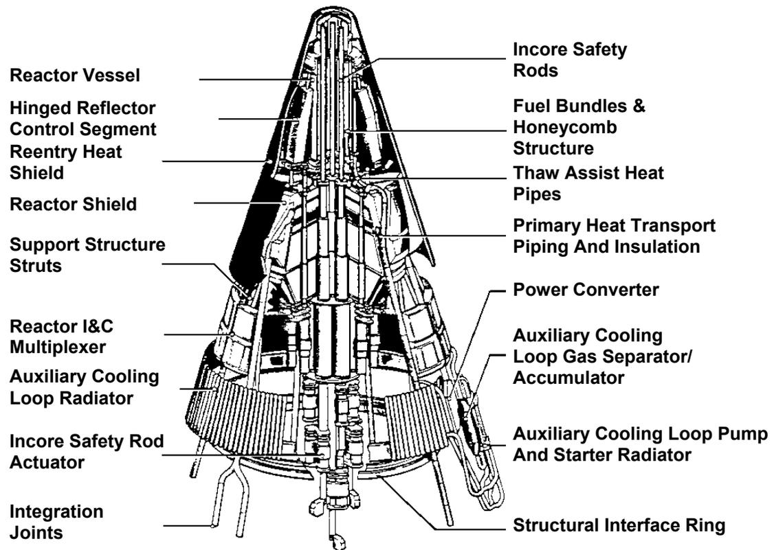
**Figure 2.** SP-100 system configuration.
