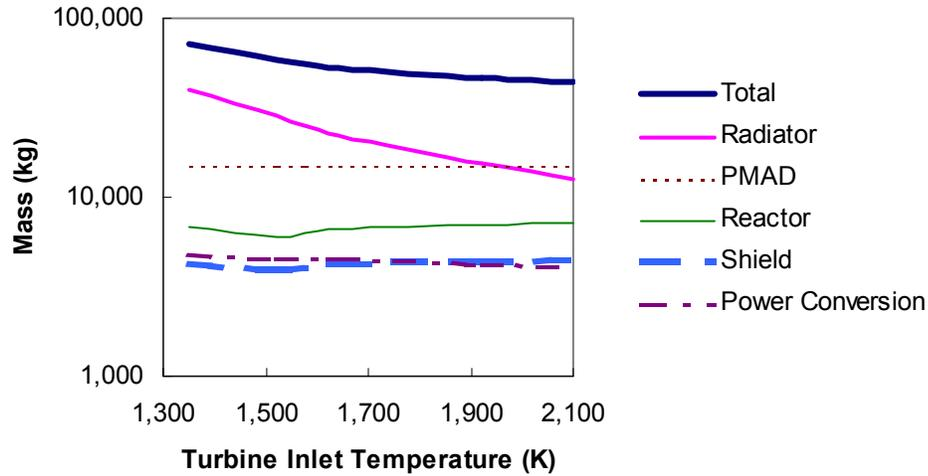
**Figure 11.** Brayton system mass decreases with increasing turbine inlet temperature.
