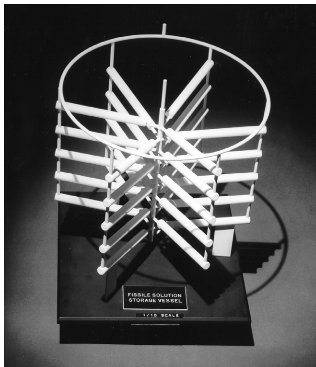
Figure 1. A novel method of routine critically safe storage of large volumes of fissile solution in production facilities was proposed based on these experiments. This one-tenth scale model was built to illustrate the concept. No prototype tank was ever built for testing purposes at Rocky Flats. The notion was rejected because too many welds gave too many potential leak points.
