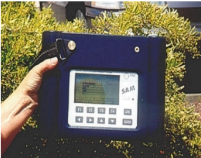
Figure 11. The SAM Model 935 With an Internal NaI probe
