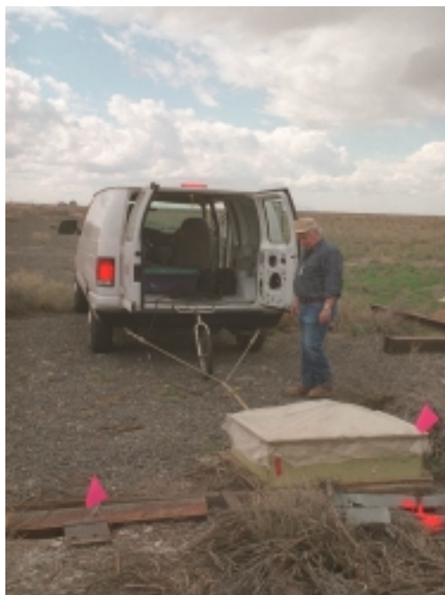
Figure 12. The EMR Antenna and Tow Vehicle, Typical Large Area Survey Setup.
