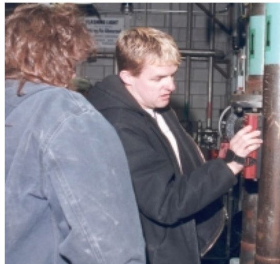
Figure 9. Alloy analyzer making a measurement on piping in the PBF
