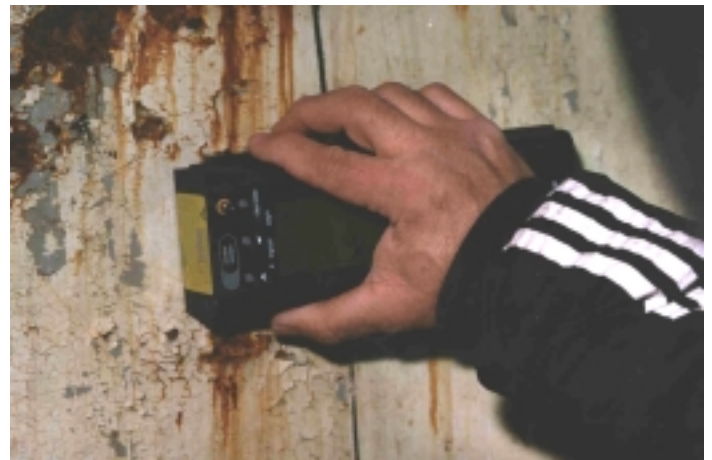
Figure 7. The LPA (Niton Series 700) Collecting a Surface Measurement.
