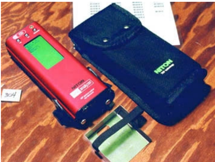
Figure 8. The NITON Series 800 Multi-Element Spectrum Analyzer with bar code template and shielded belt pouch receive the laboratory results.
