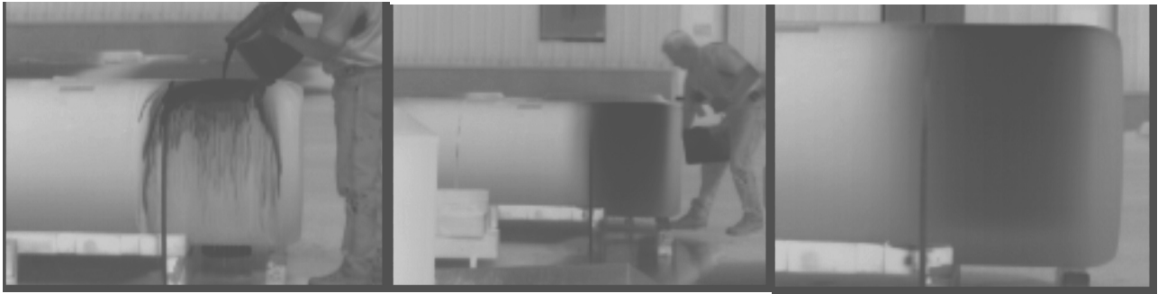
Figure 4-3. Pouring Cold Water Over the Hot Container is One Way to Enhance the Visibility of the Water Line
