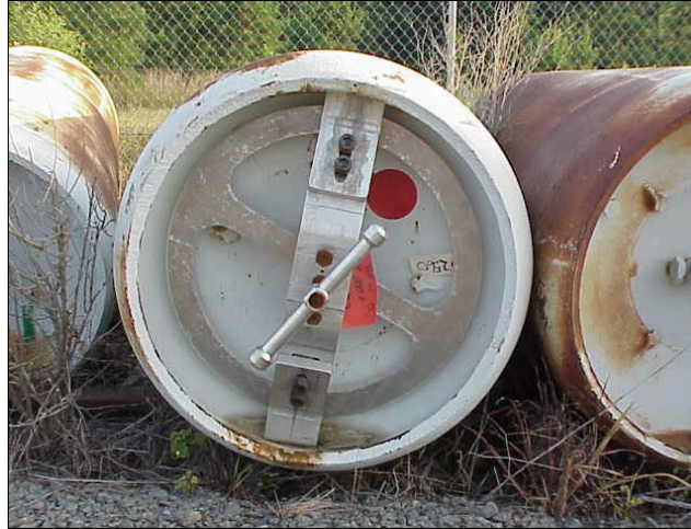
Figure 2-2. Ton Container With Fixture Securing End Plugs
