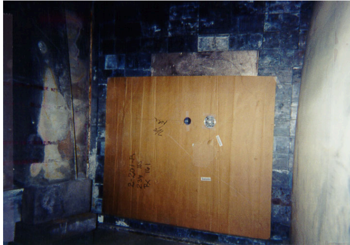
Figure 19. Activation foil packages positioned on the bismuth shield face at WSU.
