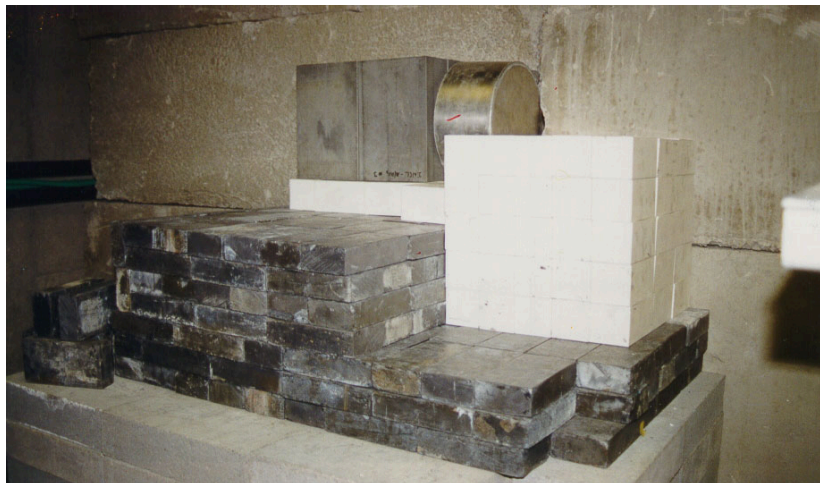
Figure 4. Partially-assembled neutron production and filtering assembly at the Idaho Accelerator Center L-band LINAC Facility.
