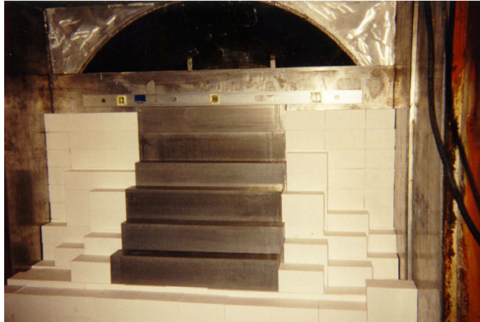
Figure 7. Partially completed WSU filter-moderator assembly, showing the \text{AlF}_3 , \text{Al}_2\text{O}_3 blocks and boral backing sheet.
