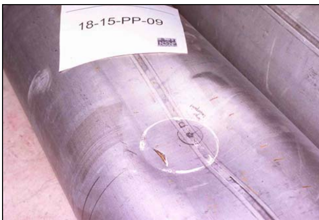
Fig. 6. Puncture drop of 457-mm (18-inch) standardized test canister response (left) and analytical prediction (right).
