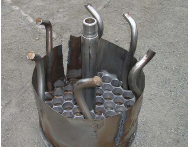
Fig. 7. Bottom basket of vertically dropped MCO (left) and analytical prediction (right). (Cuts in the basket shroud are from post-drop examination efforts.)
